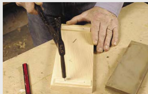
Scraps of wood nailed to the board with brads will serve as stops and hold the stone in place.
