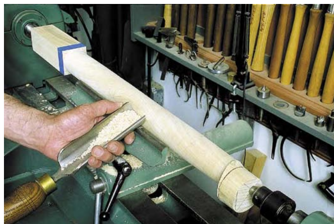
The leg is then remounted on "axis A" to cut the pommel shoulder and to turn the main portion of the leg.
