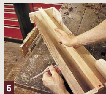
6 After defining the shoulders of the other four facets with a backsaw, sketch in the next set of tapers freehand.
