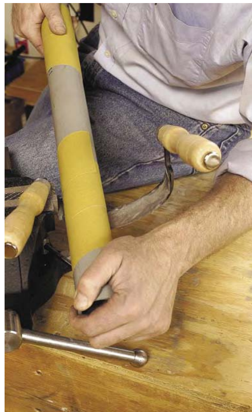
Sandpaper glued to a length of PVC pipe makes a good tool for working the inside of a curved drawknife, inshave or scorp.
