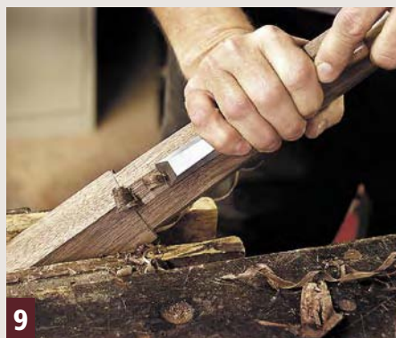
9 The top section of each of the second set of facets can't be reached with a plane. Clean up these saw marks with a sharp paring chisel.
