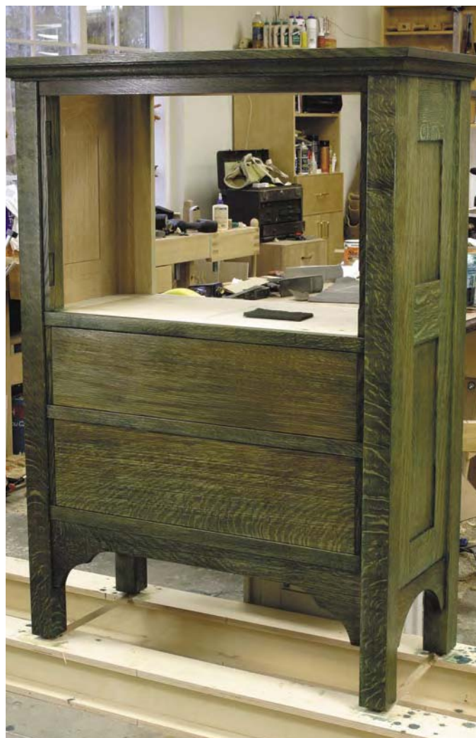
The stain is followed by a coat of natural color Watco, which lightens the color and highlights the figure of the quartersawn wood.
