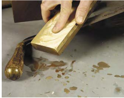
Follow the coarse stone with a succession of finer stones to remove scratches and create a smooth, uniform surface.
