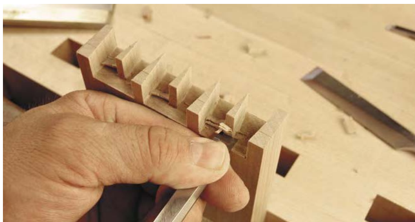
Once you have removed most of the waste with your fret saw, you'll need to remove an extra chunk of waste behind the houndstooth by chopping and paring it out.
