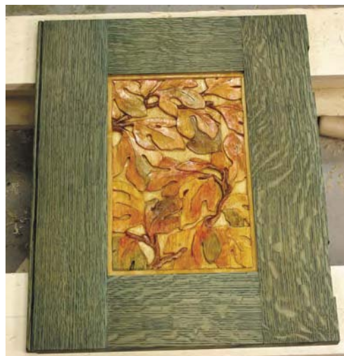
After staining, the wood is a rich green color and the open pores of the wood are filled with pigment.
