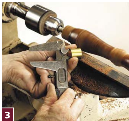
3 Having roughed out the handle, I begin fitting the ferrule by measuring the inside diameter with a caliper.
