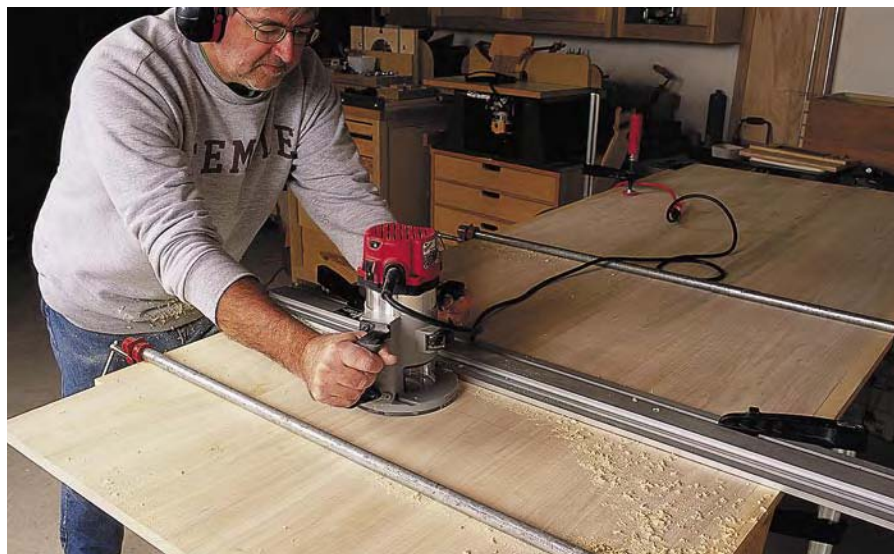
The dovetail slot must be cut with the bit set to final depth. Clamp scrap to each edge of the tabletop to prevent tearing out the top's edges. Make sure your guide is straight and rigid, perpendicular to the tabletop edges, and securely clamped.
