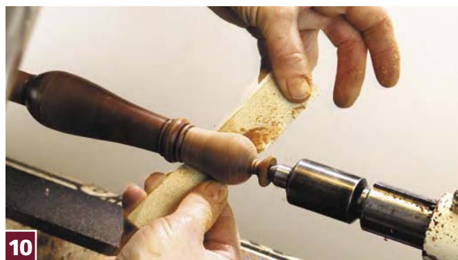
10 I've cut in close to center on the tailstock end, and am finishing up the sanding. I then finish with a hard wax, buffed out with the tool rest moved away and the lathe turned on.
