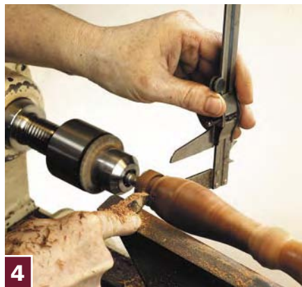
4 I hold the caliper and cut at the same time, but if you are not experienced, it is much better to cut, stop the lathe to check the diameter, and so on.
