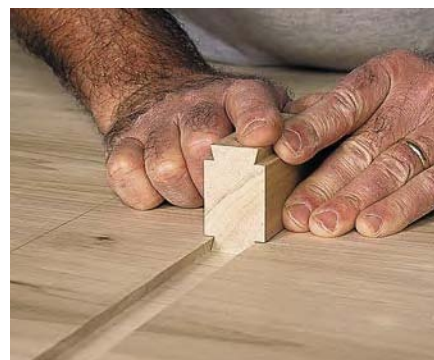
As you set up your router table for cutting the tails on the battens, fit the test block to the slots. When you have a test block that fits the slot, slide it all the way through to ensure you won't have an unpleasant surprise during final assembly of the actual batten.
