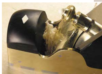
With no chipbreaker, shavings tend to collect in the mouth. However, the tool doesn't clog, it just doesn't eject shavings as quickly.
