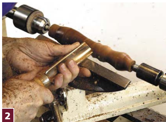
2 Using a wide, shallow spindle gouge (itself in need of a new handle!), I rough in the general shape. I prefer a handle that is wider near the ferrule than farther back, but also has a bulge on the end so I always know by feel exactly where to hold it for various types of cuts.
