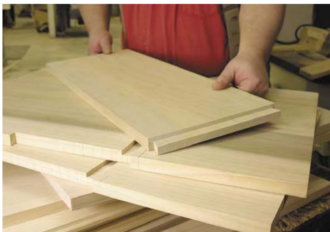
I'm just about to begin cutting the dovetail portion on the notch. Here you can see the rabbet on the front and back pieces, plus the mating notches and the dados on the sides.
