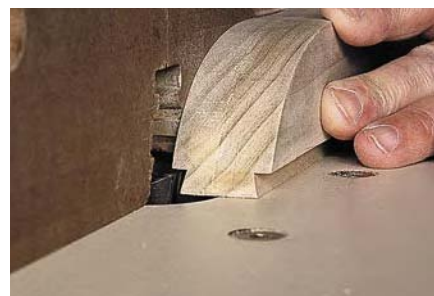
Cut the tail on each batten only after you are satisfied that you have the right fit. Slide it along the fence and cut into one face, then turn it around and cut the second face, completing the tail. You can make an angled sanding block to remove any high spots on the tail.
