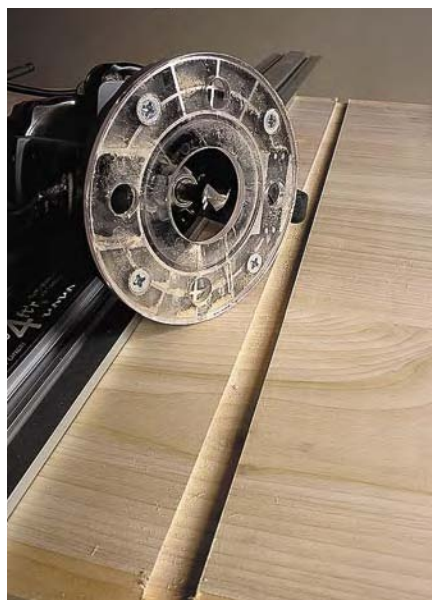
The dovetail slot for a batten doesn't need to be more than \frac{1}{4} " to \frac{5}{16} " deep. You can rout that in a single pass with a \frac{3}{4} " to 1" 14° bit on a \frac{1}{2} " shank. If you use a smaller dovetail bit, its waist will be weaker; then it's advisable to first rough out the groove with a straight bit.
