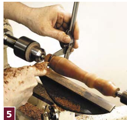
5 You'll want the fit of the ferrule to be snug, so check the diameter carefully. Leave it a bit large at this point; you will refine the fit later.
