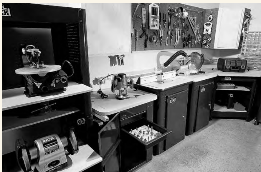
The cabinets in this organized shop have sliding storage shelves for easy access to tools that aren’t used every day.
