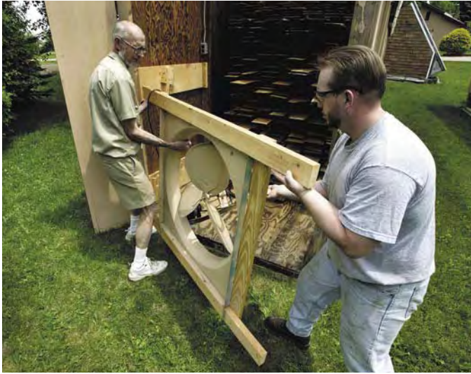
Before loading, the end of the kiln is opened by a hinged door panel and unscrewing a 4'-wide main panel. The 30" fan is being removed to give access.
