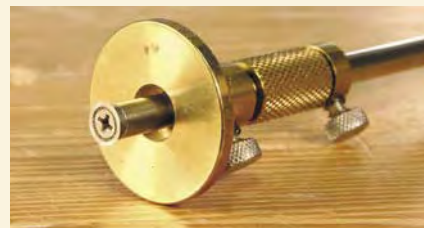
The contemporary Tite-Mark is technically a cutting gauge. Some cutting gauges have an even larger circular blade.
