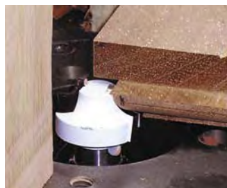
Adjust the height of your cut first, then set the ovolo cutter to leave a \frac{3}{8} " flat area on the wide stile of your fixed door.
