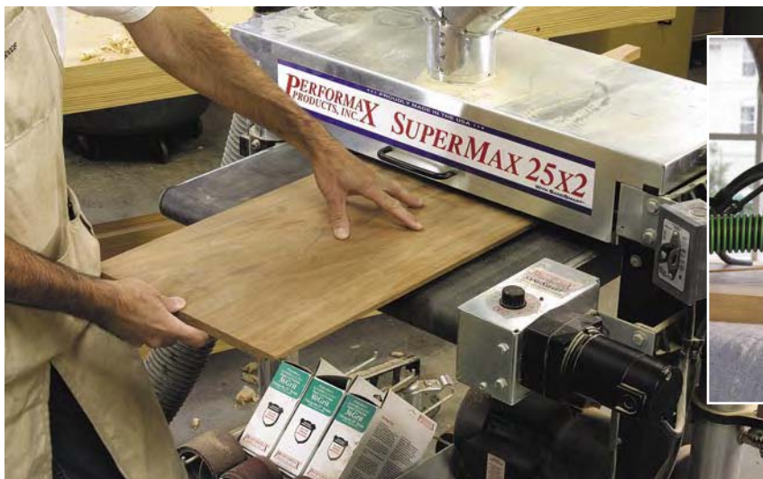
A drum sander (left) can level and true a panel much like a jointer plane. A random-orbit sander (above) is ideal for removing machining marks in a power-tool workshop.
