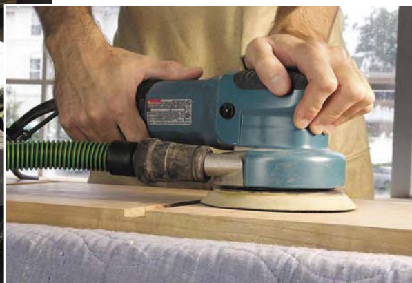
A drum sander (left) can level and true a panel much like a jointer plane. A random-orbit sander (above) is ideal for removing machining marks in a power-tool workshop.
