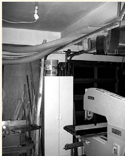
A single 50-watt halogen spot light on the ceiling augments the workshop's fluorescent lighting and provides focused brightness at the band saw blade.
