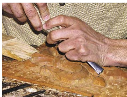
The bevel on the inside of the tool creates another shoulder, allowing the tool to cut both concave and convex shapes.
