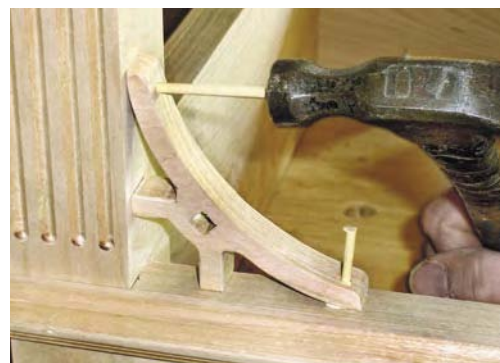
The pierced brackets fit into the corners where the aprons meet the legs. Use a small amount of glue and \frac{1}{8} "-diameter dowels to secure.
