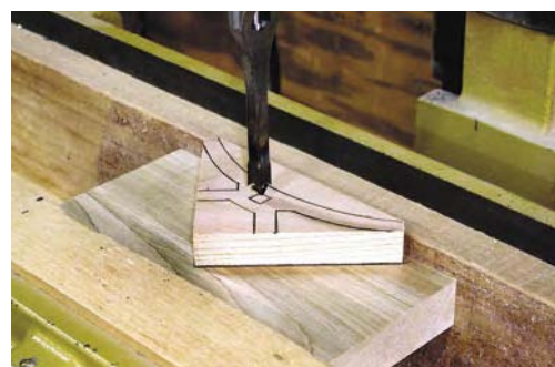
Locate the first bracket for the square hole and mark the edges on the scrap below in order to position the remaining brackets for this step.
