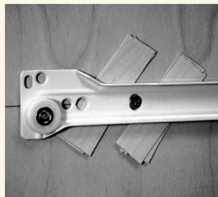
Even if the slide isn't equipped with adjusting tabs, slight adjustments in width are possible. Pieces of veneer tape can be used as shims for a tighter fit. Leave the shims oversize while fitting, then trim to size to hide behind the slide.
