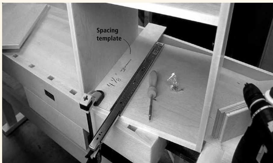
A spacing template makes getting the drawer slides mounted to the cabinet easier and helps ensure that you won't need to do as much adjusting to fit the drawers.
