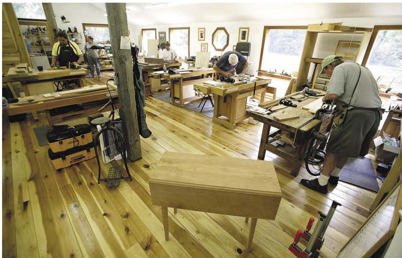
Students are hard at work on drop-leaf tables on the shop's second floor. Here, they do handwork and use portable power tools. Like downstairs, all the equipment connects to dust collectors, and air filtration systems help students breathe cleaner air – another health/safety issue that Mehler is diligent about.
