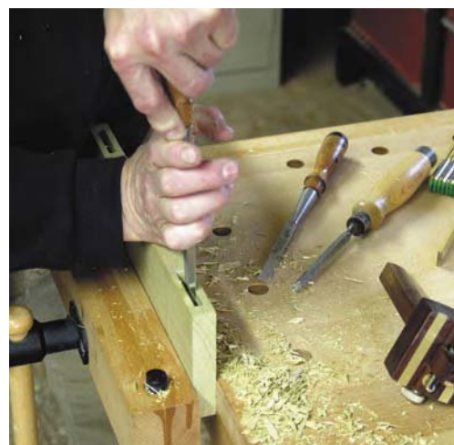
These narrow, deep mortises can be tricky to chop with hand tools.
