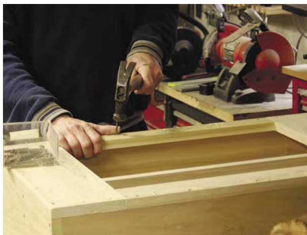
The junction of the horizontal and vertical beads must be completed with a little paring chisel work.
