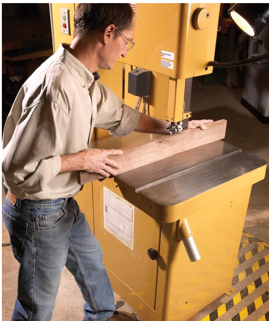
A safe saw. Band saws also offer excellent control points. The rotating blade pushes the stock against the control of the table, which eliminates the problem of the work kicking toward the operator – as long as the work is supported by the table.
