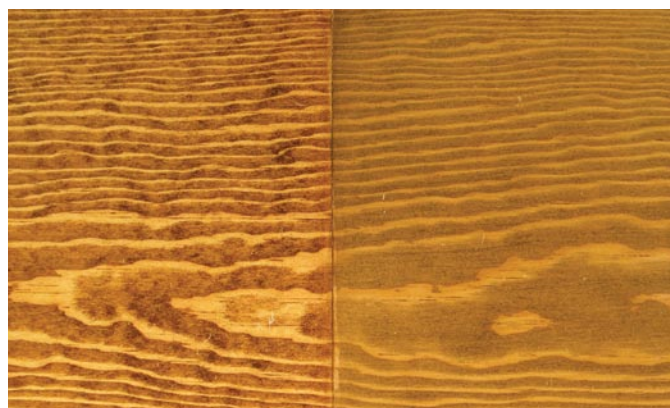
Eliminate blotching. The easy way to eliminate blotching in pine is to apply a gel stain as I have done to the right half of this pine board. The left side is stained with a liquid stain. Gel stains are so effective on pine they should be called "pine stain."
