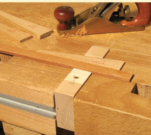
The wedge vise in use. One of the beauties of this jig is that the more you push on the work, the tighter it is secured in the jig.
