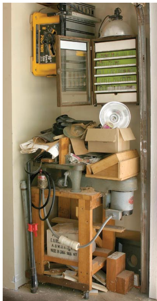
Not your average stationary tools. You have to look closely to spot the table saw hanging above a small shaper that acts as a “catch all” shelf.
