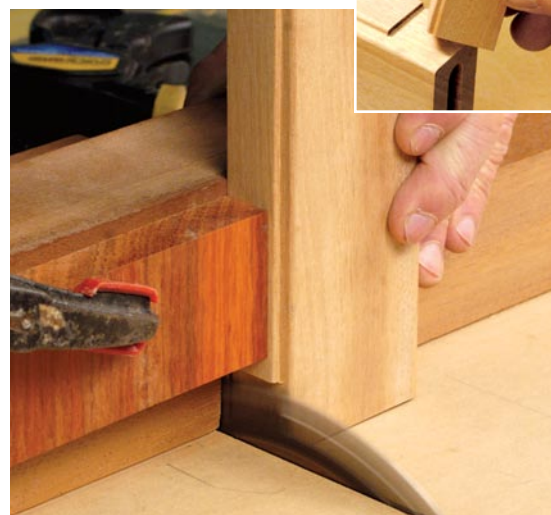
Cutting corners. A portion of the stepped radius is removed at the inside corners of the drawer openings.
