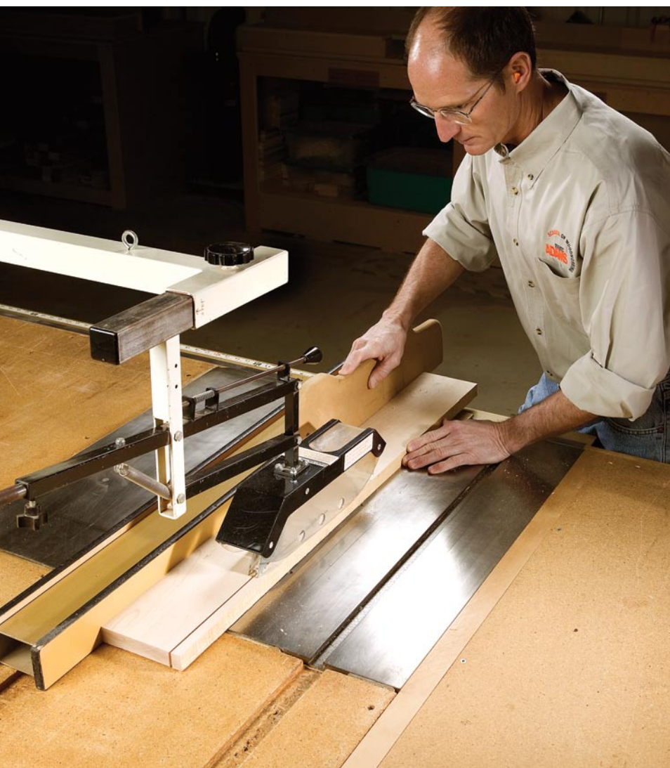
Keep away from the guard. Your push sticks and hold-downs should be designed so you can obey the 3" rule. These push sticks look different than traditional ones, but they offer advantages.
