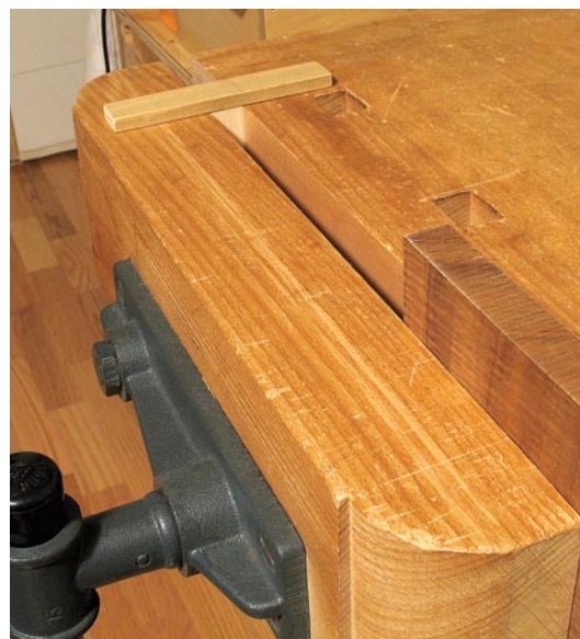
No racking, no falling. The crosspiece with the magnet rests on top of the benchtop and vise jaw. The appropriate thickness of spacer block hangs below it thanks to the magnet and screw.
