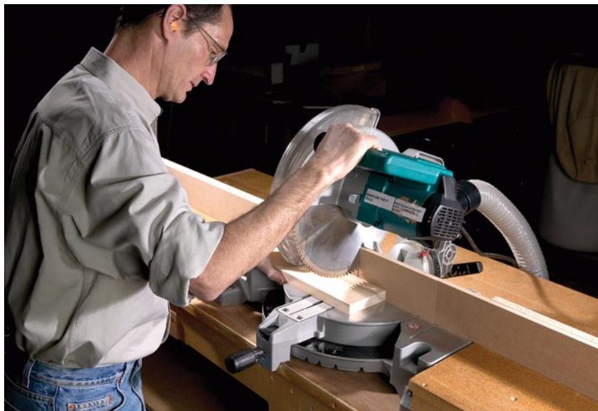
Good control. Miter saws offer good control points. The spinning blade pushes the stock down and against the fence during the cut.
