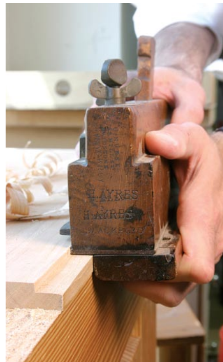
"New" way to make rabbets. A small-scale project such as this is a great way to try out different ways of making joints. Here I'm making the rabbet in the bottom with a moving fillister plane.
