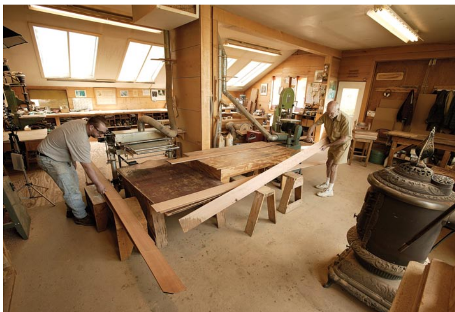
Re-purposed. Recycled sliding-glass doors serve as skylights, flooding the shop with natural light.
