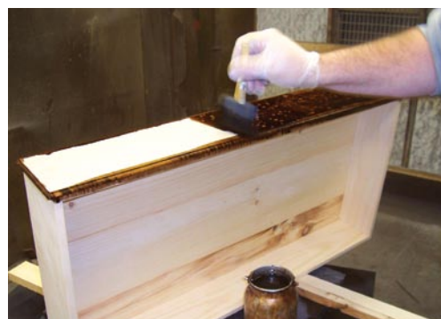
The most effective way to apply the stain to a drawer front without getting the interior of the drawer covered is to use a foam brush.
