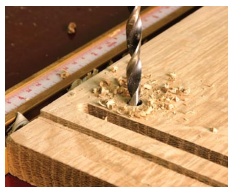
There are pin locations at both the top and bottom that act as guides for the doors. Use the drill press for this step – unless you've a steady hand and good eye.
