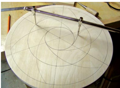
The layouts for both a four-jaw and a six-jaw chuck. (You could use a trammel for both layouts.)
