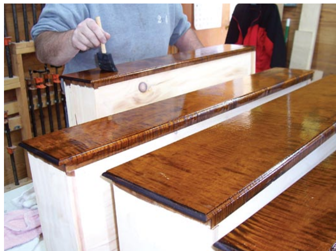
A coat of boiled linseed oil is a great way to add depth to your finish. Make sure it is boiled (not raw) linseed oil. The raw will not dry properly.
