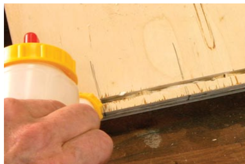
Practice getting the right amount of glue in the slot. You want to coat the surface of the plate without having excessive glue squeeze-out, or introducing too much moisture in the interior of the joint.
