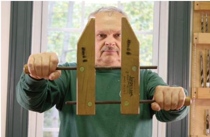
Adjusting a handscrew: The hand that holds the center handle remains stationary. You move the jaws by cranking the lower handle over the center handle. Clockwise opens the jaws. Counterclockwise closes them.
