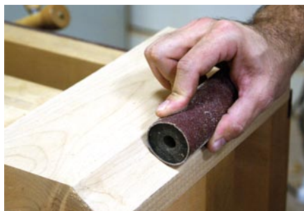
Multi-function sander. A great way to clean up a sculpted cove is with a sanding sleeve and rubber spindle from a spindle sander.
