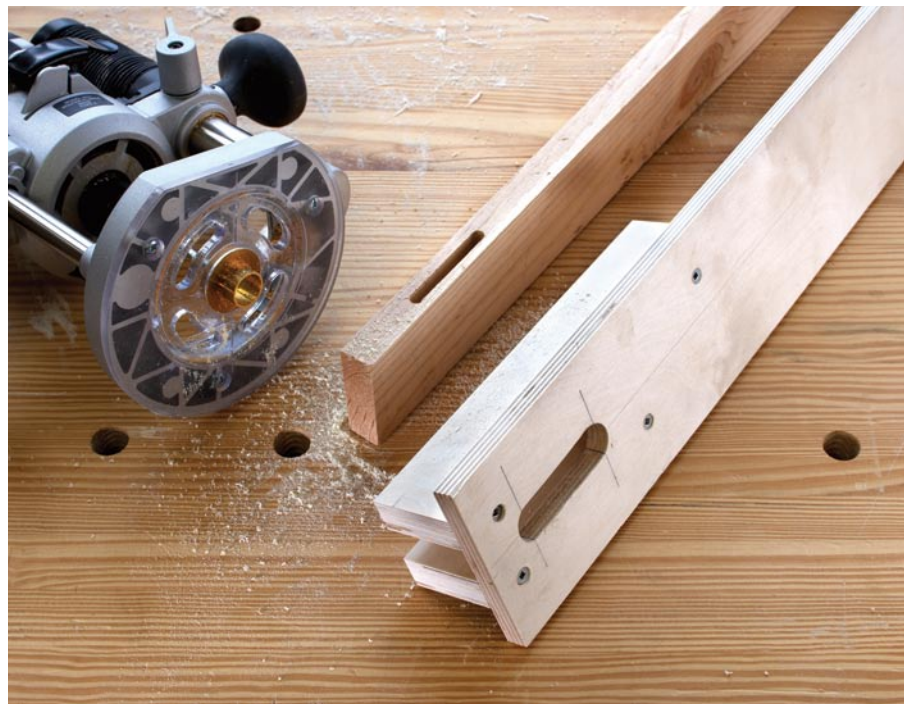
Job-specific tooling. A mortise-and-tenon joint is one of the strongest, most useful joints in woodworking. With scraps from the waste bin, you can create a jig that does the job and is simple to use.
