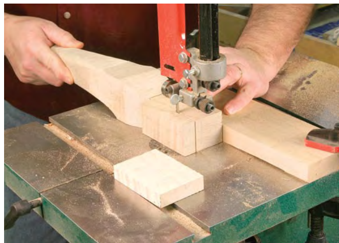
A right way to cut. There is a specific cut order to remove the waste from the two faces of the leg block. Choose wisely and the work is quick.
