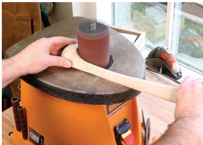
Shape with power. Hand tools can achieve a flat foot top, but power sanding at a spindle sander is quick, accurate and repeatable. Goodbye hard-to-work end grain.
