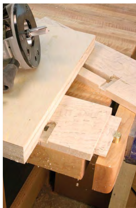
Right with the pattern. Routing the dado for the candle-slide supports is a snap. Use a pattern bit with a straight fence that you set right on the layout line.
