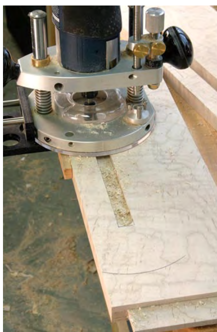
Plough out the groove. A plunge router and straight bit make quick work of cutting the candle-slide opening. Of course, an attached fence is a must-have.
