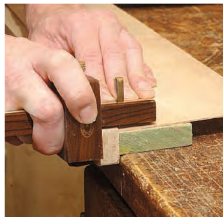
An efficient way to cut. With a simple jig and a marking gauge you can cut or rip string inlay easily.
