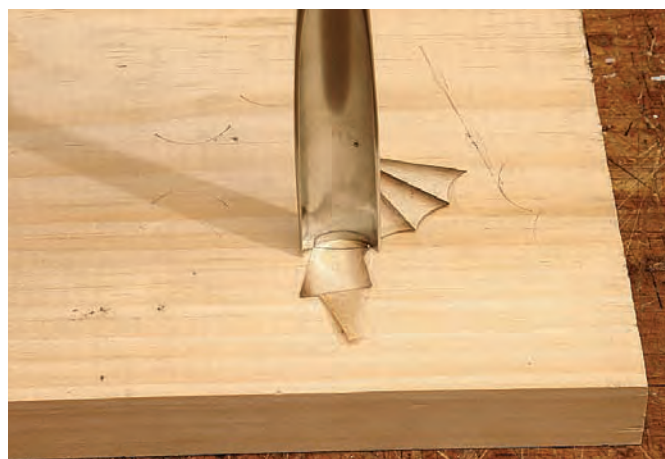
Gouge the ends. Use an appropriately sized gouge to create the scallop at the end of each blade.
