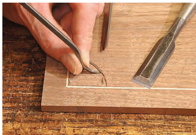
Preparing the recess. Once the recess is routed to the correct depth and close to the edges, remove the remaining waste with small chisels.
