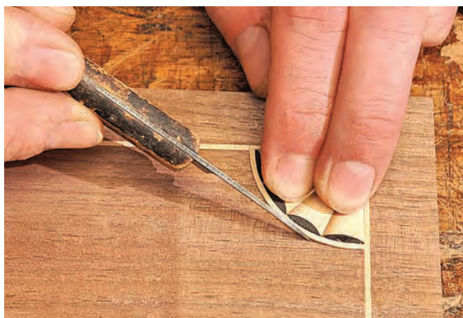
A fine line. Carefully cut a line for the fan inlay after the piece is trimmed and final shaped.
