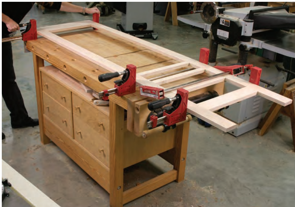
Dry fit, then glue. With everything squared up and fitting, add glue and clamp your face frame together and set it aside to dry.
