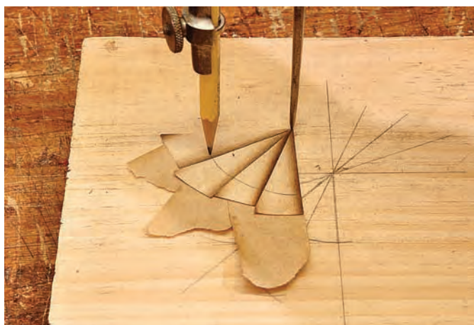
Mark the arc. A compass marks the outer edge of the fan, which is held together with veneer tape.
