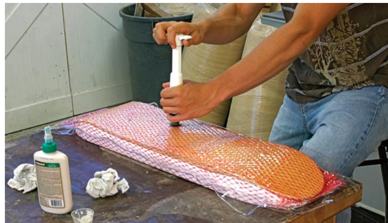
This sucks the air. Pumping the press produces a vacuum that forces the plies to the shape of the mold.
