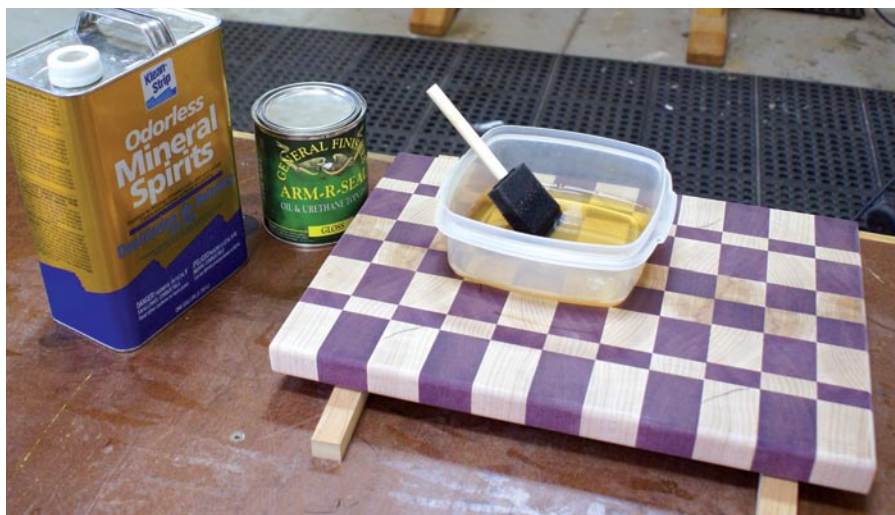
Prepped and ready. The varnish, diluted about 75 percent with mineral spirits, is ready to use.
