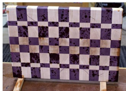
Travelin' through. The varnish travels through the grain and seeps out on the other side. Once it starts to soak through and you've coated both sides, let it dry in this position overnight.
