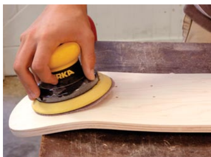
Get ready to paint. Sand the bottom of the board with a random-orbit sander and #120 grit to smooth the board out and remove excess glue.
