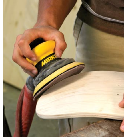
Ease the edges. Use the sander to round over the edges to prevent splintering when riding.
