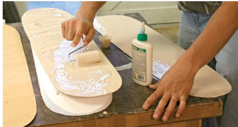
Even coat. Roll glue onto the veneer with a 3" roller included in the kit, and make sure there is plenty of glue on the edges.
