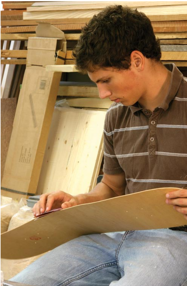
Sand first. Sand off any rough edges to prevent them from puncturing the vacuum bag and to guarantee the veneers glue together tightly.
