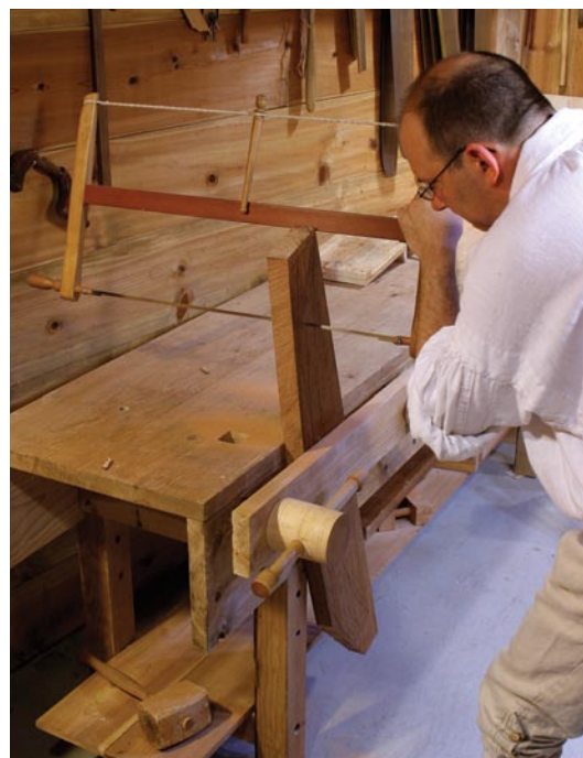
Tricky driving. This frame saw is fitted with a 3 / 8 "-wide blade. It's basically a huge coping saw. It cuts fast, but can be tricky to use. Steering the cut requires a light touch and constant attention, especially as the cut gets closer to parallel to the grain. Even though these teeth are filed for ripping, the wood's grain can grab the blade, pushing it one way or another. It's much easier to use it at some angle to the grain. Unfortunately, the most critical part of this cut, the area where seat rails attach, was purposely oriented with the grain.
