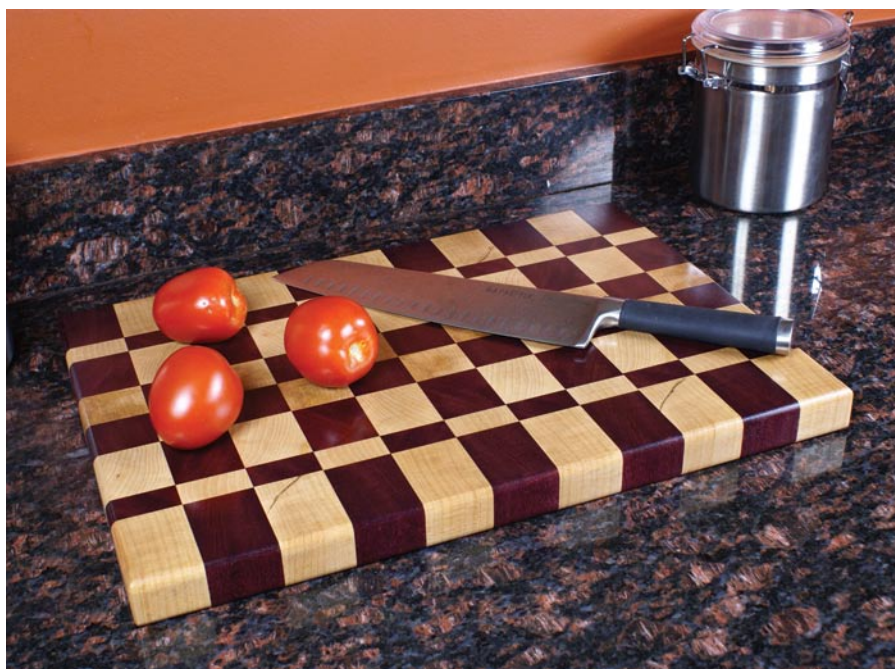
Cut to the finish. Using thinned varnish – instead of the traditional mineral oil and wax – takes a big slice out of the time it usually takes to finish a butcher-block cutting board.
