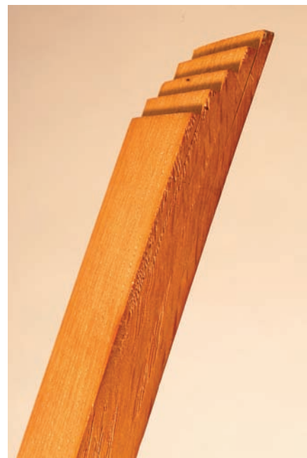
Cut then curved. This example of curved, tapered lamination in English oak shows how the glue lines can virtually disappear. They only become visible near the end, in the waste piece, where the clamping pressure was not adequate.
