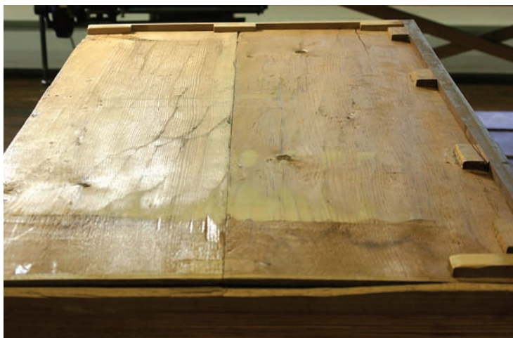
Underneath. The jack plane leaves slight but visible scallops; unseen surfaces on quality pieces, such as the bottom of this 19th-century drawer, were left with the jack's surface. This can be useful in helping to identify authentic antiques.
