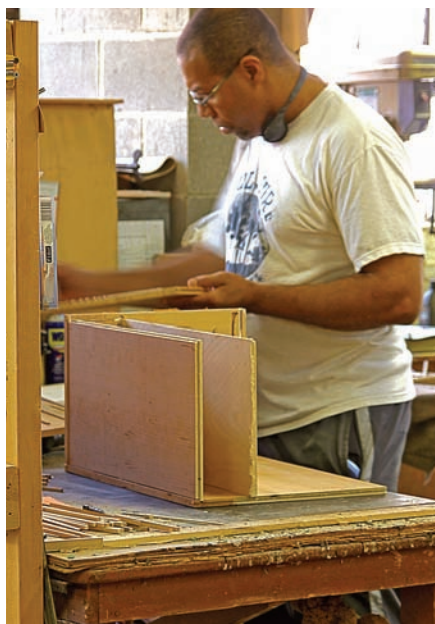
All together now. With all the joints milled precisely, Terrell Adams assembles boxes in a quick, well-practiced process.
