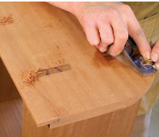
Soak then shave. After sawing off the wedges, the joints are soaked with paint thinner to make it easier to trim the end grain flush.
