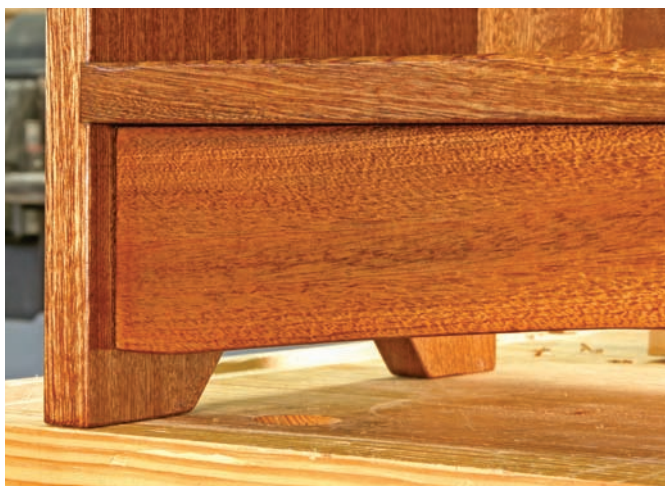
No one will ever know. Located below the shelf and \frac{1}{2} " back from the front edge, the drawer appears to be a fixed apron.
