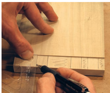
Drafting square. Register a plastic drafting square against the narrow shoulder to divide the "giant tenon" into small tenons.
