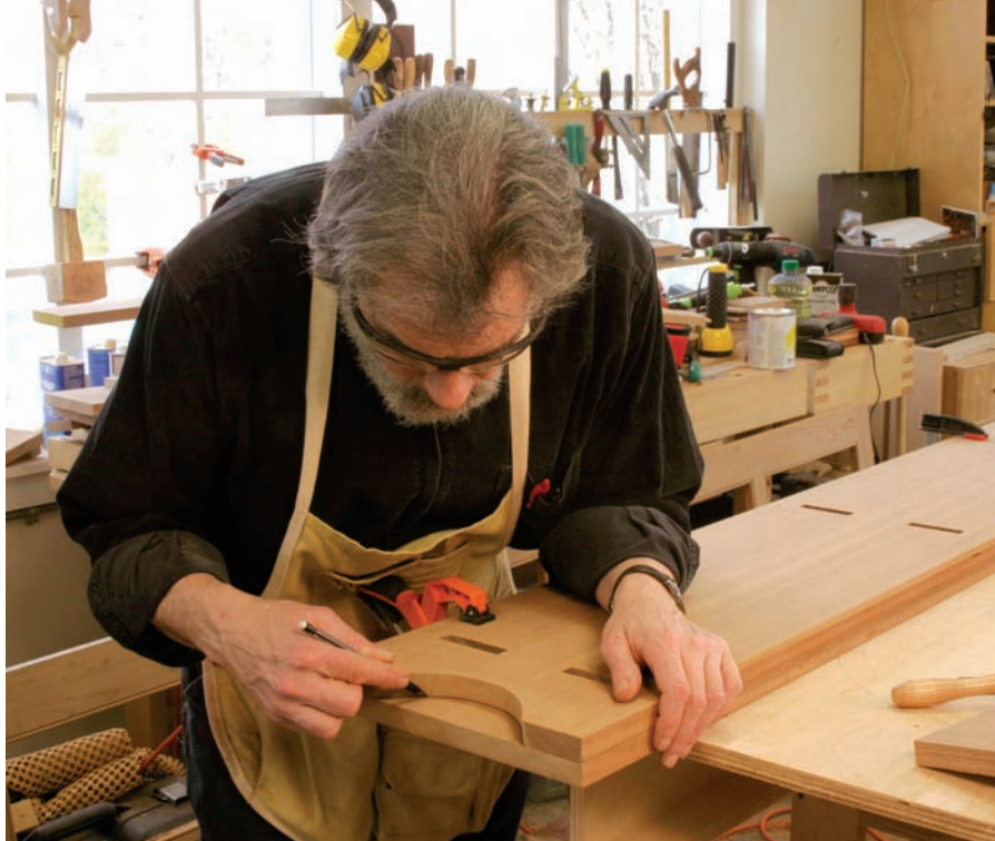
One side makes another. After the curves on one side are completed, the first side is used as a template to make the second side.
