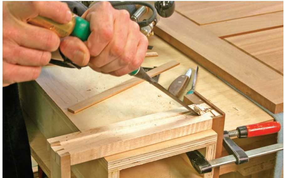
Hidden away. The hidden drawer rides on wooden slides attached to the carcase. The end of the groove will act as a stop for the runners, and needs to end in the right spot.
