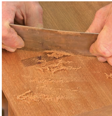
At the same level. Following the plane, a scraper is used to smooth the exposed tenon ends and the cabinet sides.
