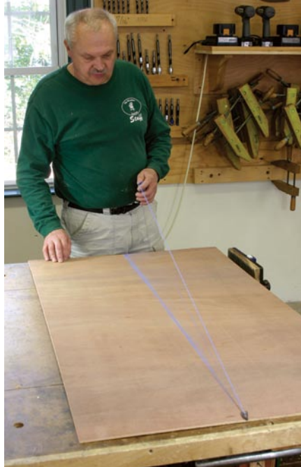
Chalk line. While a chalk line leaves a wide mark in comparison to a pencil, it's unlikely that precision will be paramount in a line that's too long to mark using a straightedge.
