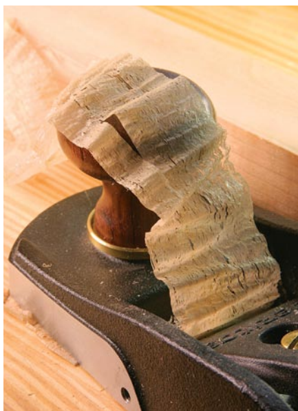
A bit thinner. This shaving is about half the thickness of the thick one. Use this size shaving if you start to see tearing on the surface of your project.
