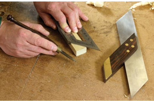
Miter squares. Traditional miter squares resemble try squares, with a wooden handle secured at a 45° angle to the blade. A Japanese miter square has a raised foot that fits over the edge of a board, and a 45° blade at both ends.
