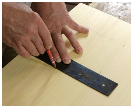
Try square. An easy test to see if your square is indeed square is to place it on a proven straight edge and draw a line. Now flip the square so the handle is pointing in the opposite direction, and see if the tool confirms the line. If it doesn't, buy a new square.
