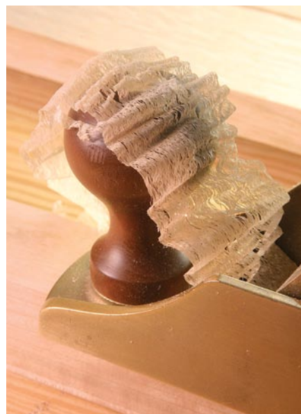
Tissue stops tearing. Before I break out the sander I try cutting a shaving such as this one. It takes more passes than I like, but it is less likely to tear the grain.
