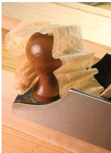
Thicker is faster. A substantial shaving such as this one reduces the number of passes you take, but it can increase your chances of getting tear-out.
