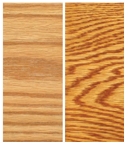
Boiled linseed oil darkens. Boiled linseed oil (shown here on oak) and, to a lesser extent, varnish darken considerably as they age. On the left is freshly applied boiled linseed oil. On the right is boiled linseed oil that has aged about 10 years.
