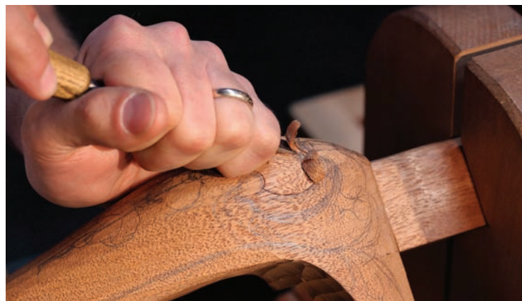
Wiggle room. Storb carefully walks the cut into his stab line, making sure to keep the corners crisp.
