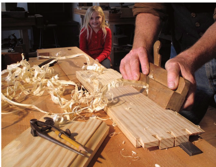
Moulding after mitering. Here I'm using a complex moulding plane on the skirt. Before moulding the skirt, remove the bulk of the waste with other tools.
