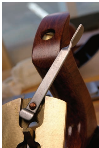
A loose lateral. The lateral-adjustment lever on both planes (the Börg's is shown) is lighter weight than the Lie-Nielsen's.
