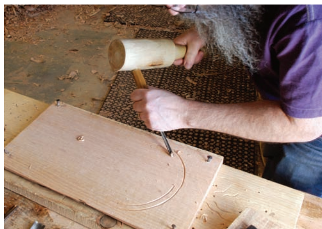
Cut the arch. Define the top and bottom of the arch using a V-tool driven by a mallet.
