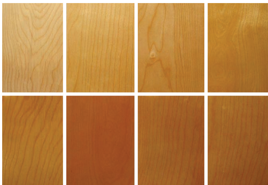
Seven finishes on maple. Top row from left: unfinished, clear paste wax, water-based finish, nitrocellulose lacquer. Bottom row from left: clear/blonde shellac, amber/orange shellac, polyurethane varnish, boiled linseed oil.
