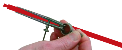
Blade width. Set your first pair of dividers to the thickness of your drawer blade.
