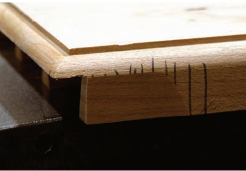
Smooth closure. A bevel on the bottom edge of the drawer front allows the front to seat to the case. There's no bump against the divider and the drawer rides up the bevel to close fully.
