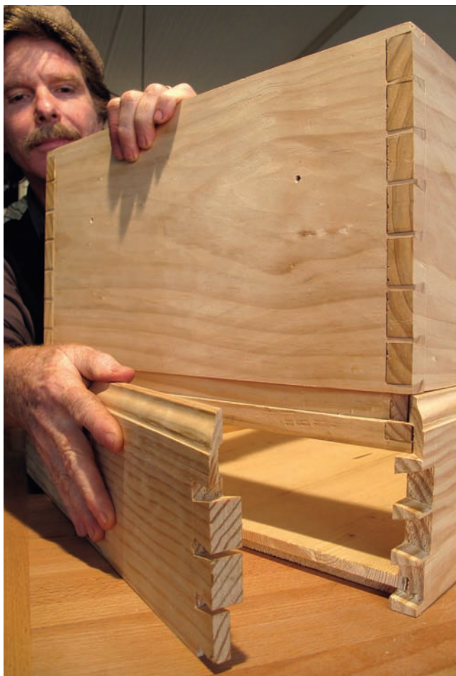
Grooves, pins and tails. Pulling away this one piece of the skirt reveals all this chest's secrets.
