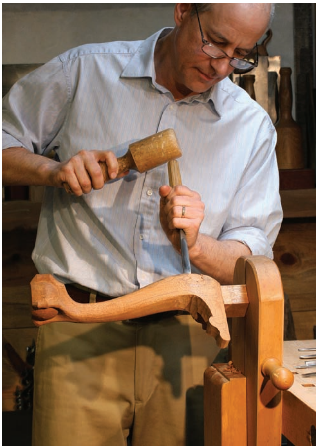
Double-bevel approach. Double-beveled gouges are Storb's secret for maintaining a perpendicular orientation to the workpiece surface.
