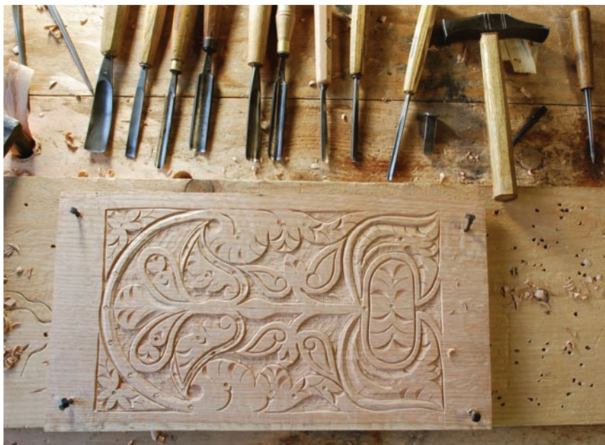
The tools and the workholding. Carving these panels requires a few different tools: simple carving tools (gouges and V-tools), an awl, a compass and stamping tools.
