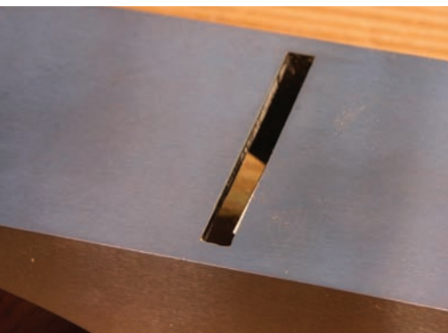
An extra cutter? The frog of the Wood River plane slips below the sole when you adjust the frog. It takes some persuading to get the frog straight in the plane's body.
