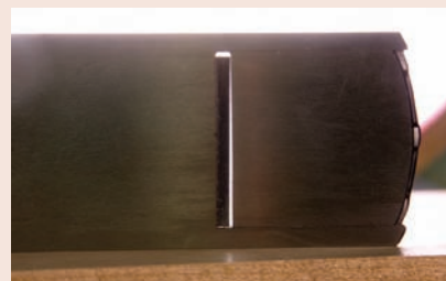
Crooked bed. The mouth of the first block plane in working position.
