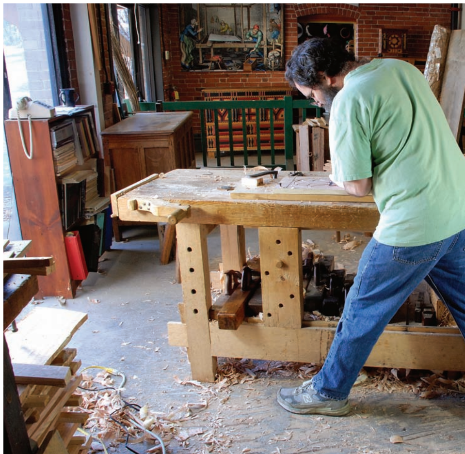
The proper stance. When I carve I keep my elbows close to my body. Most of the movement comes from the lower part of my body.
