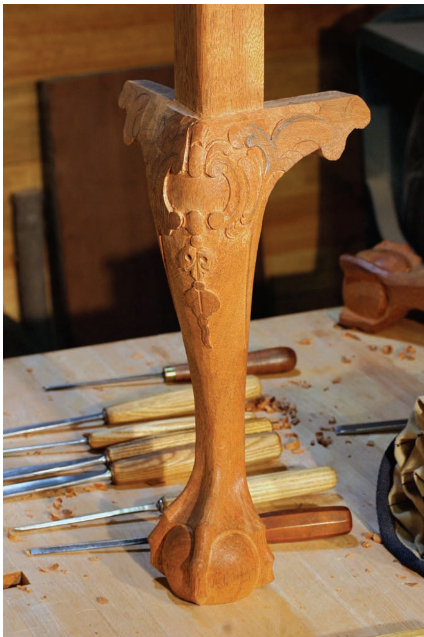
Masterful work. This is the work of master carver Christopher Storb. The C-scrolls and acanthus-leaf carving decorating the knee of this chair leg represent some of the most difficult and prized style of work done in the 18th century.
