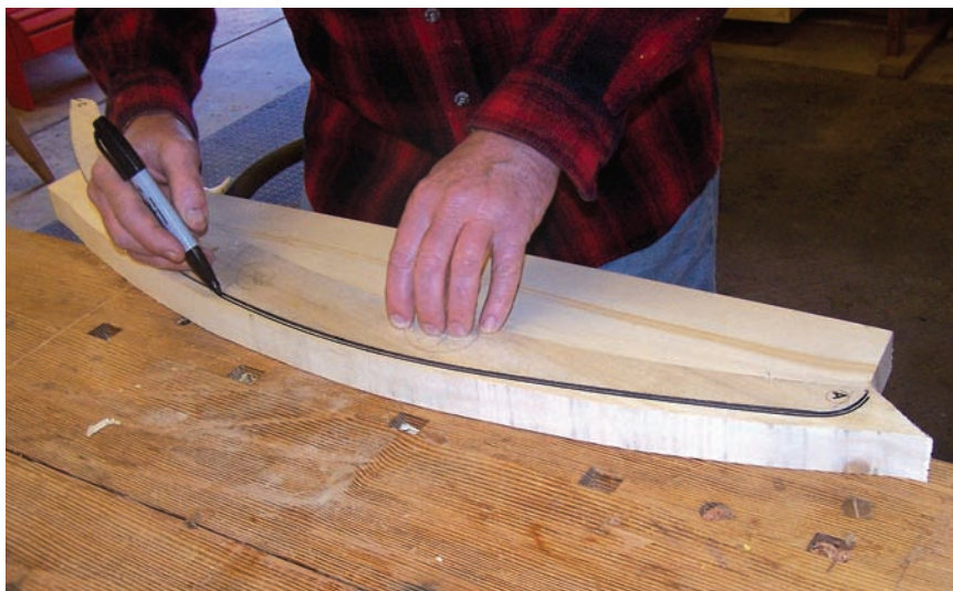
Marking multiples. A template ensures that both frames match, and it speeds the process if you are making several chairs.
