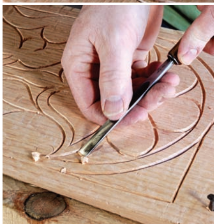
More gouge work. Continue removing background material with a gouge. The goal is a faceted surface, not a flat one. You will stipple the background later.
