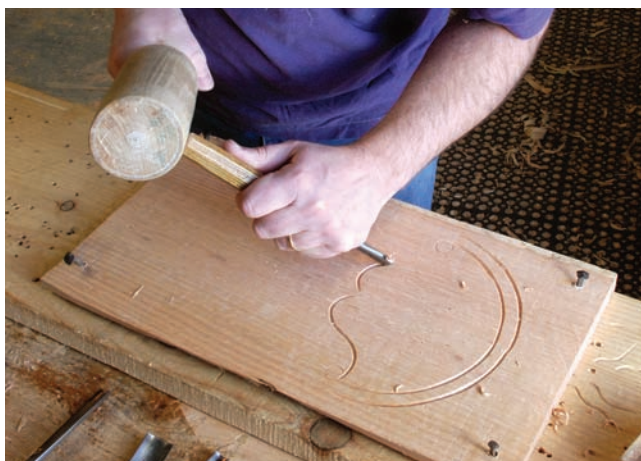
Find the right angle. Here I'm defining the tulip shape below the arch. Note the angle of the tool. Using too shallow of an angle will make it difficult to steer.
