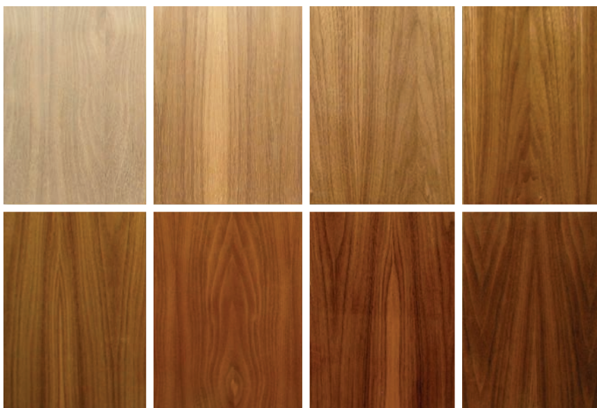
Seven finishes on walnut. Top row from left: unfinished, clear paste wax, water-based finish, nitrocellulose lacquer. Bottom row from left: clear/blonde shellac, amber/orange shellac, polyurethane varnish, boiled linseed oil.
