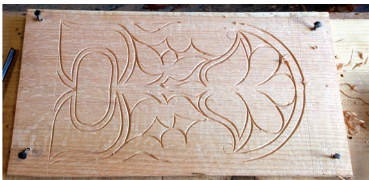
The completed outline. Here's the finished outline of the panel, which was completed entirely with a V-tool and a few simple layout lines.
