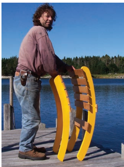
Slip fit. The two curved frames slide together. When assembled as a seat, the three slats at the intersection keep it in position without any special hardware.
