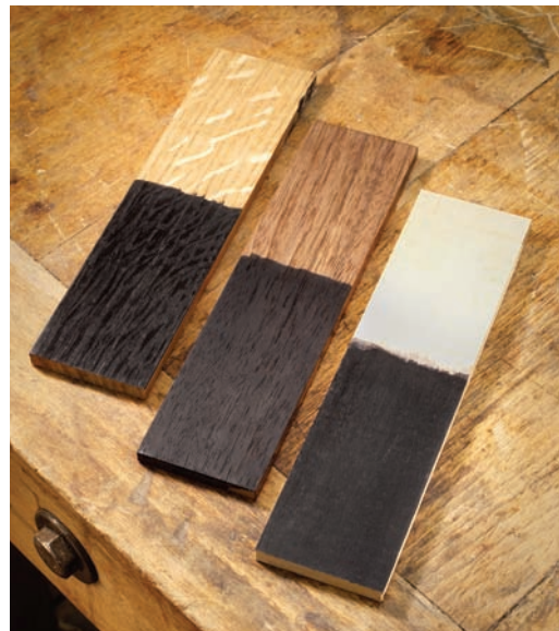
Different woods, same result. Three samples of ebonized wood (oak, walnut and maple) showing color consistency with the stain with the grain variations being prominent.
