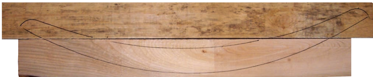
Adding to the curve. To maintain straight grain at the intersection, you may have to add width to your frame stock.
