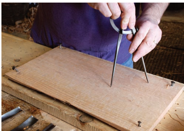
Scratch the arch. The layout requirements for this panel are minimal: a centerline, the margins of the carving and a single arch at the top.
