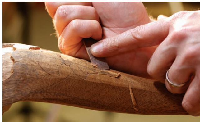
A light touch. Stopped edges help Storb achieve a polished finished surface, but the real key is light cuts.
