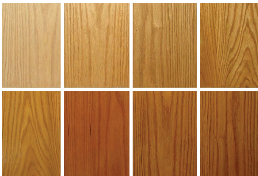
Seven finishes on oak. Top row from left: unfinished, clear paste wax, water-based finish, nitrocellulose lacquer. Bottom row from left: clear/blonde shellac, amber/orange shellac, polyurethane varnish, boiled linseed oil.
