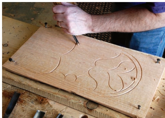
Defining the leaves. Move down to the lower third of the panel and use a V-tool to define the drooping leaves emerging from the urn.
