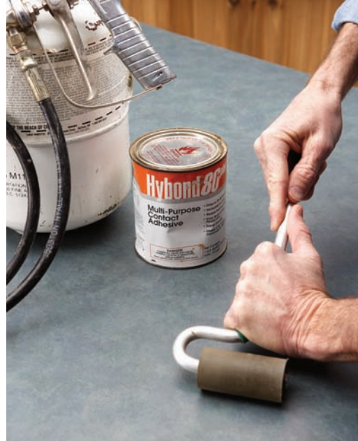
Under pressure. Contact cements grab immediately, but need pressure applied to form a complete bond.
