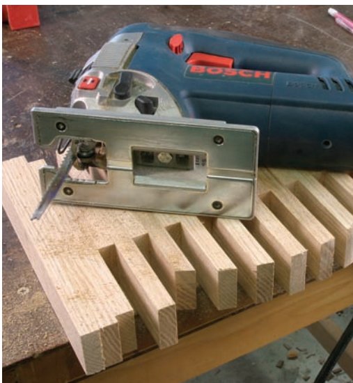
Jigsaw to shape. To keep yourself from having to do too much end-grain sanding (not fun), use a good jigsaw blade to cut down on blow out. (We recommend Bosch “Xtra-clean for Wood” blades.)
