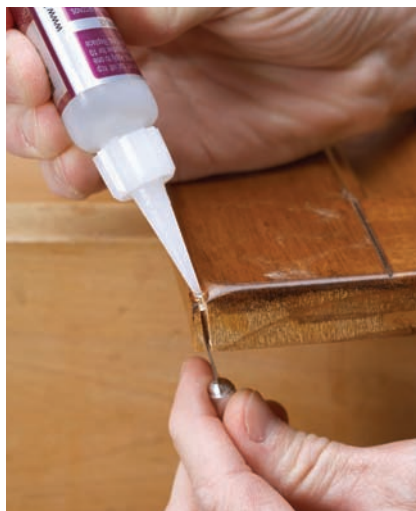
Quick fix. Cyanoacrylates (super glues) don't have much strength, but are ideal for quick repairs.
