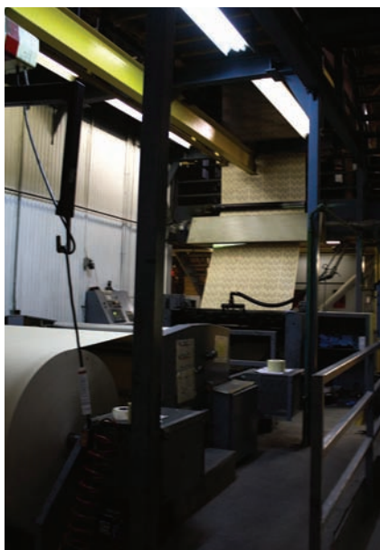
Roll it out. Here you can see the 55" rolls of paper as they are fed into a printer that inks the grit and brand on the backside of the paper.
