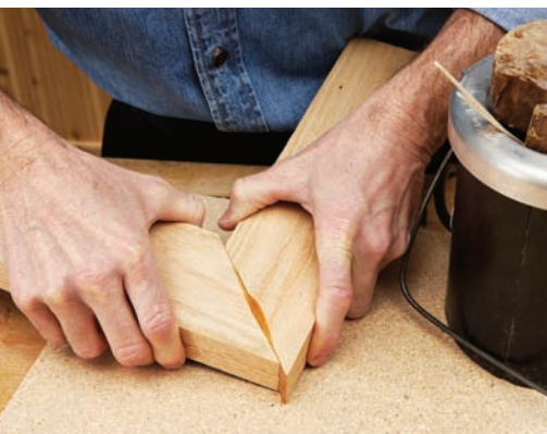
Rub the right way. Hide glue grabs as it cools, making it possible to make complex assemblies without the use of clamps.
