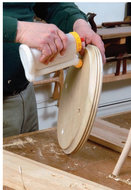
Test-fit, then glue. If the test-fit works out, go ahead and glue the legs into the top, tapping them lightly in place with a hammer.
