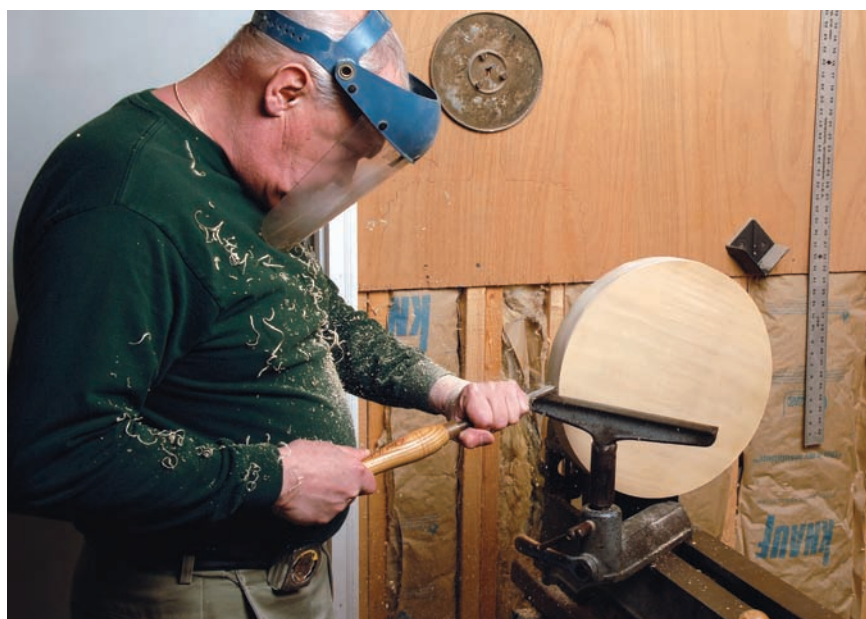
Smooth edge. Turn the blank's edge smooth.
