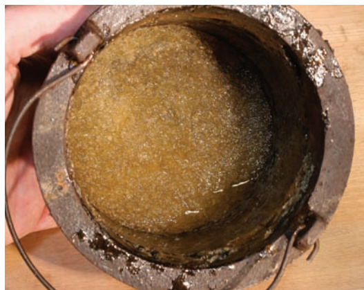
Hot and sticky. I cover the bottom of my glue pot with dry glue. Then I pour in cold water to cover it. The dry glue quickly absorbs the water and becomes a gelatinous mush. Ten minutes later, I look in the pot, and maybe add a bit more water. In an hour it looks like this. The glue has absorbed all the water it cares to. A little excess water is present. Were there a cup of excess water, I would try to pour it off. The glue is gloppy, not runny at this point. Or you could forget about it and cook the water off.
