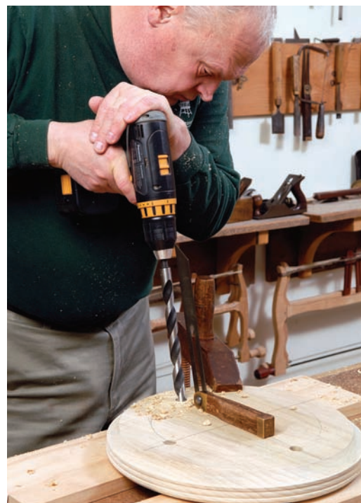
By eye. Use the bevel's blade to get the drilling angle, and sight the bit along the line – no jig needed.
