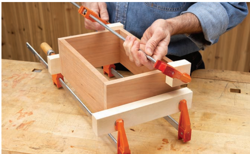
Spread the pressure. Blocks between the clamps and the work prevent damage, and increase the area under pressure.
