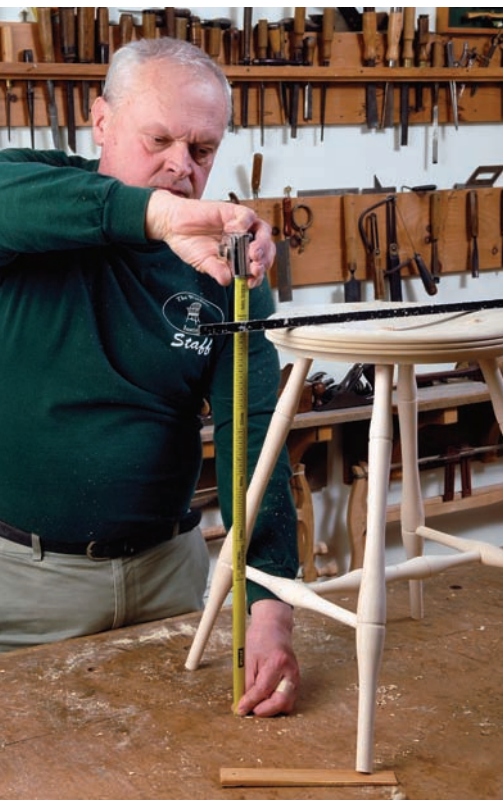
Shim to level. Use shims to level the stool and measure the height from the top of the bench to the top of the stool.
