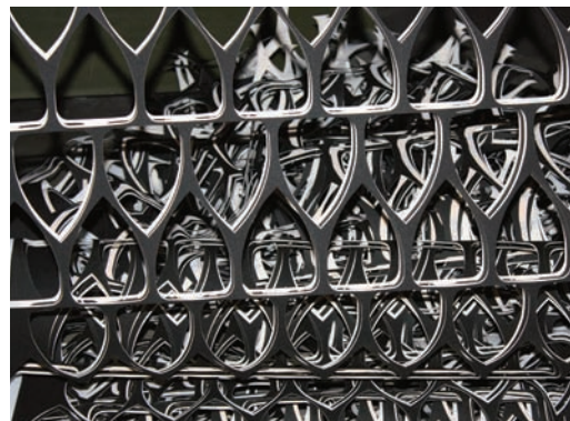
The leftovers. Here’s what the paper looks like after the die-cutter.
