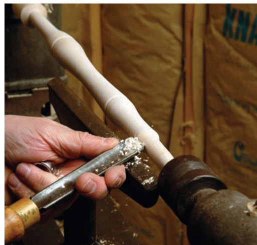
Four legs. Turn the legs to the profile and dimensions shown in the drawings below.
