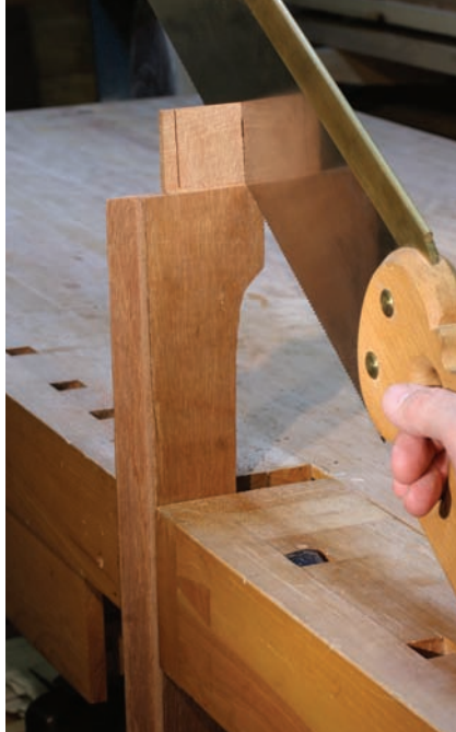
Wedge prep. Repairs and X-rays done at the Philadelphia Museum of Art indicate 18th-century Philadelphia chairmakers sawed their tenons in preparation for wedges.
