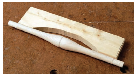
Cradle. This simple cradle keeps the stretchers from rocking as you drill.
