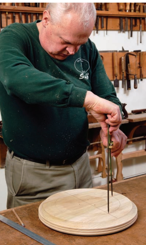
Divide and find. A simple way to find the location for the second diameter is to walk off the half-circle with a pair of dividers.
