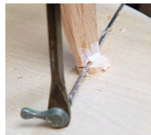
Drive, then cut. After I drive a wedge and cut it off, I whittle the next wedge from the same piece of oak.
