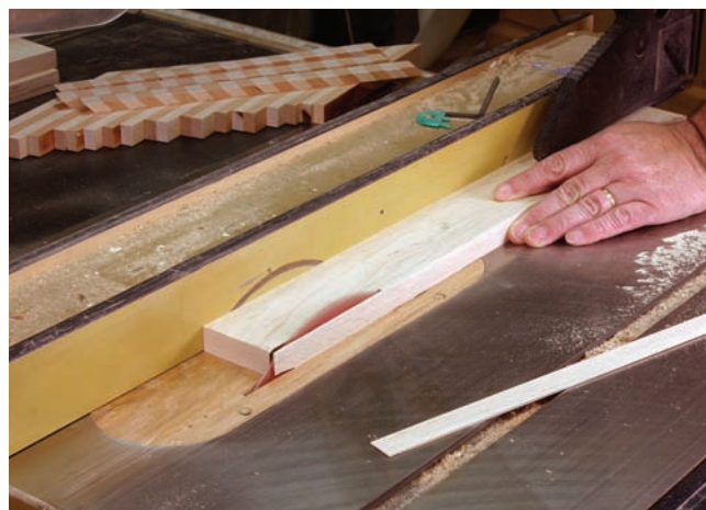
Thin is in. String pieces border the herringbone strips. Set your fence to leave the string pieces as cutoffs—that's the safest method to produce multiple thin pieces.
