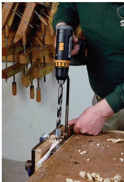
Chairmaker's mantra. Notice that I'm drilling from the top of the leg. To avoid drilling upside down, remember the mantra: "Top of leg to top of leg."
