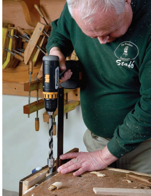
Stretcher holes. I use a \frac{9}{16} " brad-point bit to drill 1\frac{1}{8} "-deep holes for 1" tenons.
