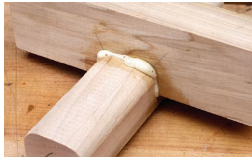
Filled with foam. Polyurethane glues foam as they cure. This adds no strength to any gaps and can be a pain to remove.
