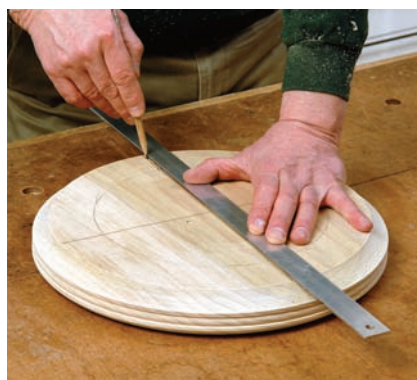
Two purposes. The two diameter lines locate the leg holes and act as sight lines.
