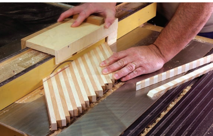
Not a random rip. Sizing the pieces of assembled scraps is important to the overall task. All the parts of the inlay add up to match the width of your groove.
