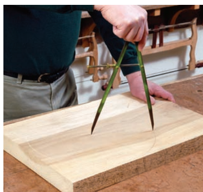
Seat layout. Use a compass to mark a 14" circle for the seat of the stool.
