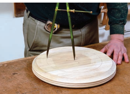
Locate the leg holes. The first step is to mark a 4\frac{1}{2} " radius.
