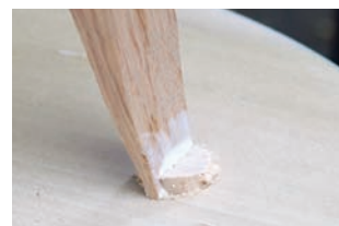
Tapered wedges. Your wedges should taper in both width and thickness.
