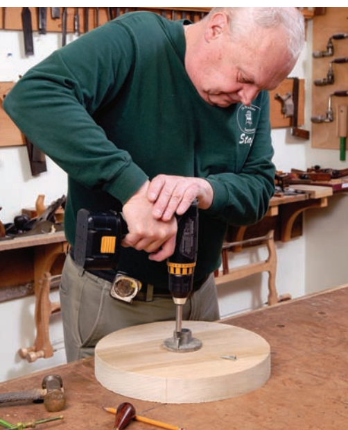
Centered. Mount your face plate so it's centered on the seat blank.
