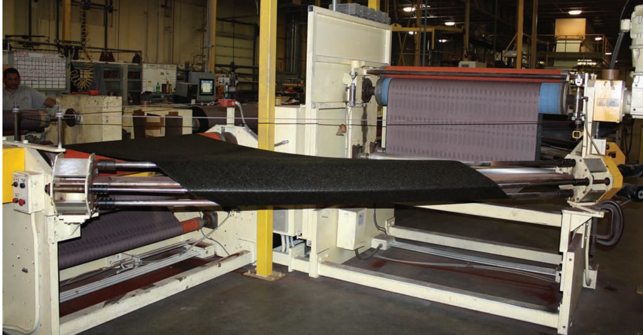
A sharp turn. This machine flexes the finished paper several times to increase its durability. Then the paper is rolled back up.
