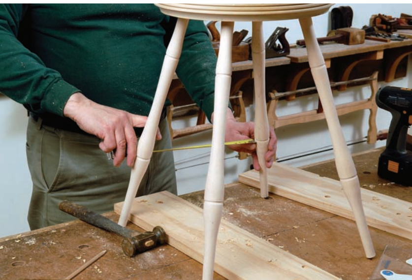
Stretchers. The stretchers will connect at the lower ring locations; turn the stretchers as needed, to fit.
