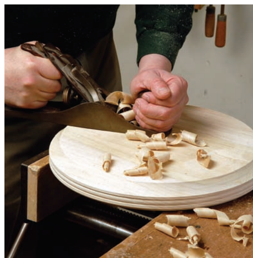
Handplane. Use a handplane to remove the boss (the projecting wood) from the face plate.
