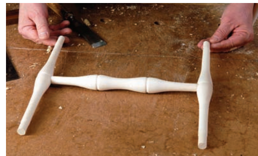
An even plane. Check to ensure your assembled "H" lies all in one plane.
