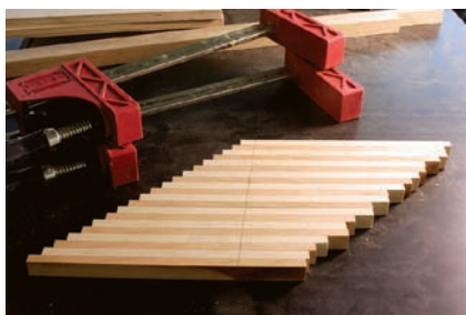
Scraps of design. There's nothing more satisfying than to use shop scraps. Here you see the beginning of the shop-made inlay. Positioning the pieces at a 45^\circ angle as assembled increases the yield of inlay.
