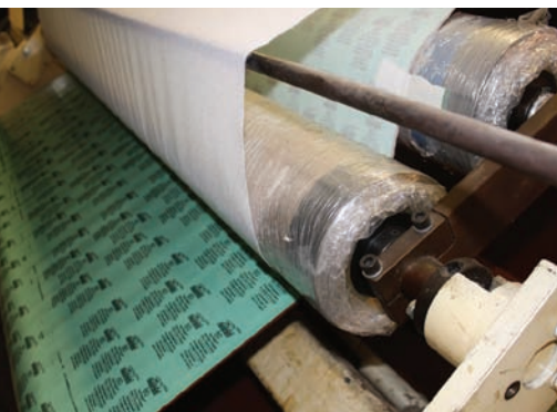
Acres of loops. The white stuff is the “loop” part of hook-and-loop. It’s glued to the back of the paper on this large machine, which also applies the sticky-back glue if need be.
