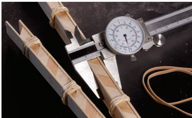
It's good to be strong. Inlay pieces assembled with glue and clamped with rubber bands are slightly wider than the groove size.
