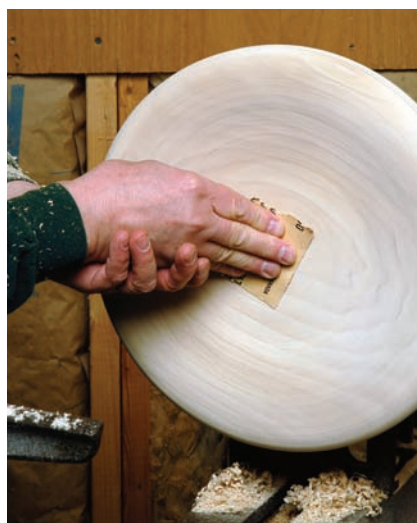
Easier sanding. Sand the seat surface with the workpiece spinning on the lathe.
