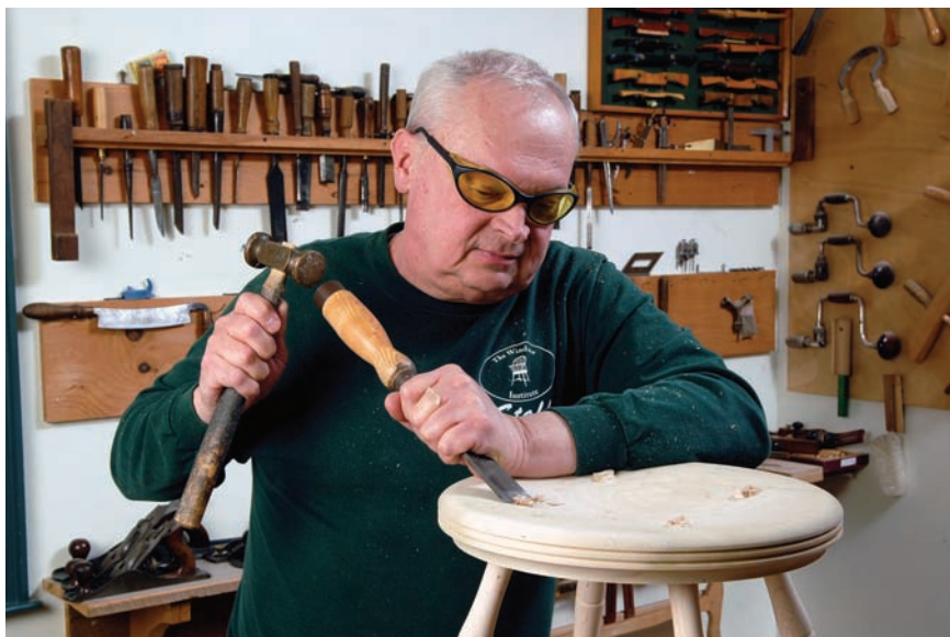
Gouge flush. Use a gouge to trim the excess off the tenons, flush with the seat, then sand smooth.
