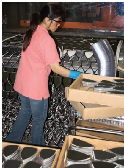
A giant punch. An Ali employee stacks finished sanding pads as they come out of the die-cutter. The cutter can slice through five or six sheets of sandpaper in one swoop.
