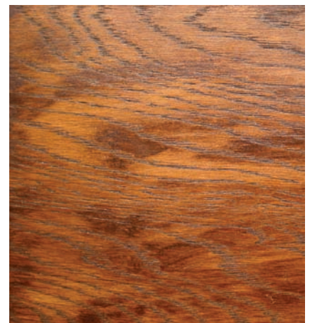
Blotching. The darker spots on this oak panel are areas where the stain dried before it was wiped off. To keep this from happening with fast-drying water-based and lacquer stains, work faster or on smaller areas at a time, or get a second person to wipe off quickly after you apply the stain.
