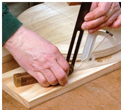
A matter of degree. The leg holes are at 21^\circ off perpendicular.
