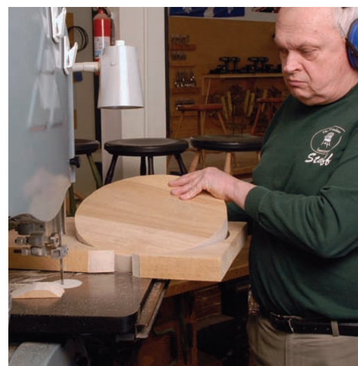
Rough shape. Use the band saw to cut out the seat blank.
