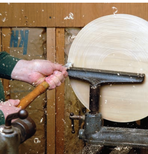
Shape. Turn the outer edge of the seat to match the shape shown in the "Seat Profile" drawing.
