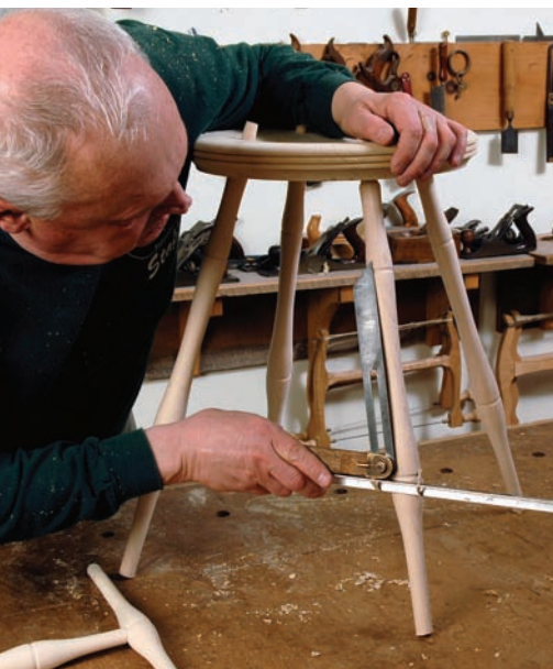
Workpiece determines angle. A straightedge clamped across the legs at the rings will help you find the correct hole angle.
