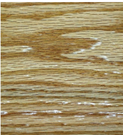
Bleeding. The shiny spots on this oak panel show where an oil/varnish blend has oozed out of the pores and dried on the surface. To keep this from happening, check your project every half hour or so after you apply the finish and wipe off any bleeding before it dries.
