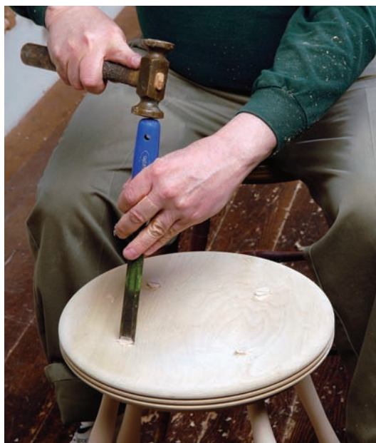
Chisel, not kerf. I split the ends of each leg with a chisel – this takes far less time than moving to the band saw for a kerf cut.
