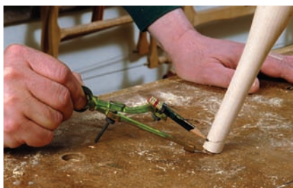
Mark. Mark a line around each leg to locate your cut.
