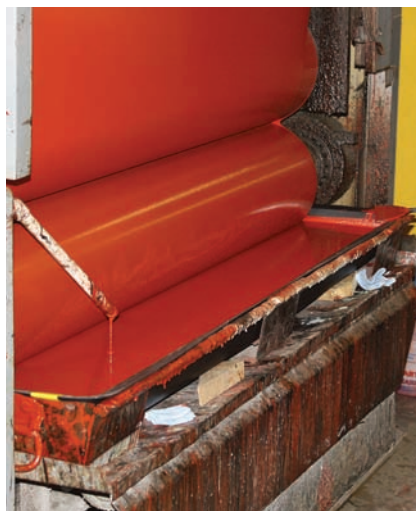
A pot of glue. The red stuff in the tray is the resin. The glued paper travels up out of the tray and into the room where it gets its grit.
