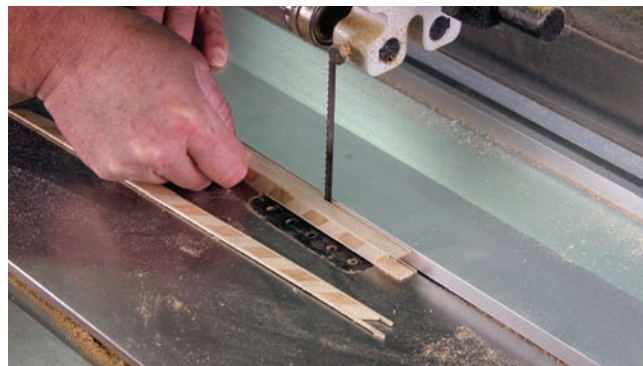
The last step. Strips of herringbone inlay are ripped at a band saw to produce the final pieces. Plane the faces before work at the band saw commences and keep the pieces thicker than the groove is deep.
