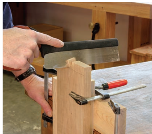
Three clamps and you're ready. With the work clamped to the jig, and the jig clamped to your bench, you can practice making cuts with a handsaw.
