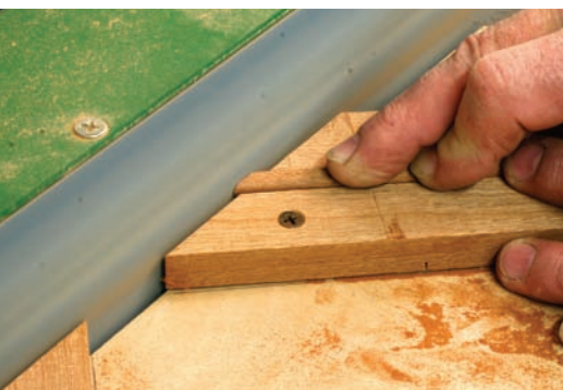
Too close for comfort. The beads on the legs are too small to miter with a power saw. I cut them by hand and created the miters on the horizontal belt sander.
