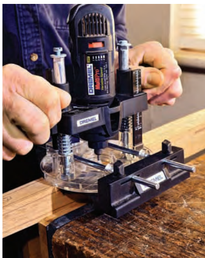
Accuracy is key. A rotary tool makes short work of the straight grooves along the leg's edge.
