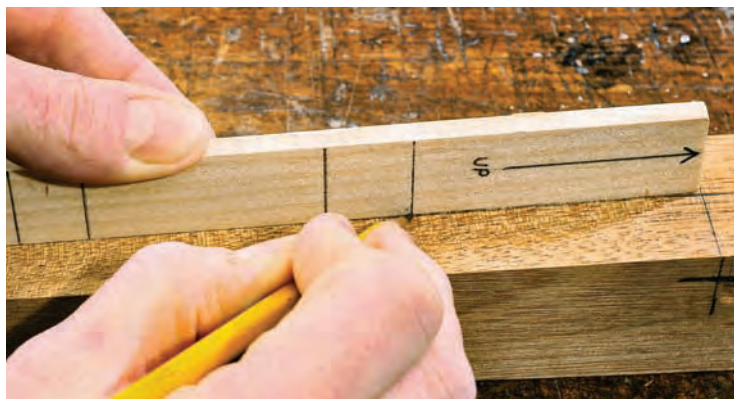
Keep your story straight. A story stick ensures layout uniformity from leg to leg.
