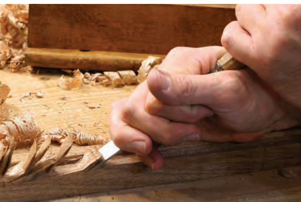
Chiseled rabbets. I cut the rabbets for the seat using my trusty \frac{5}{8} " firming chisel. Because the outside face of the rail is the reference face, no fenced plane will be helpful. No matter what tool I use, I'll have to do some amount of cleanup. So I chose the fastest tool I could.
