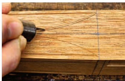
Define your groove. The double-bladed knife, tracking in the line scribed against the template, sets the width of the groove.
