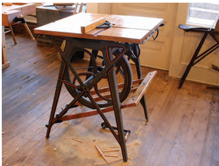
One foot-power. The treadle table saw at the school has both a rip fence and a crosscutting guide. It makes remarkably clean cuts with (just a little) practice.
