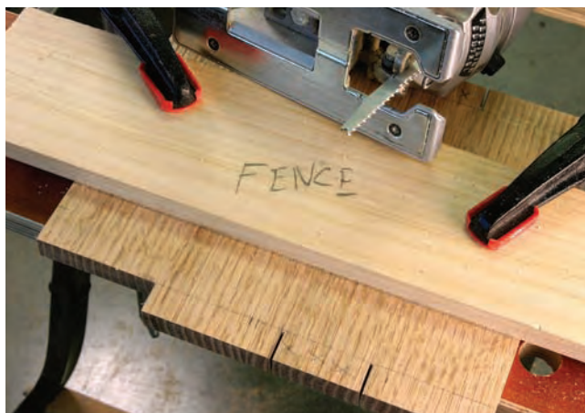
Set the fence. With the fence in place remove the easy bits from the ends.
