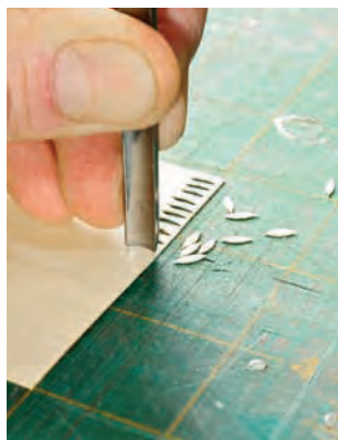
Keep the edge. A quilt cutting mat underneath your work helps to keep a sharp edge on your tools.
