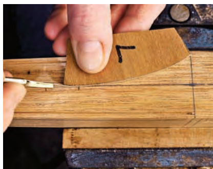
A constant arc. Templates establish one side of the groove for the stringing.
