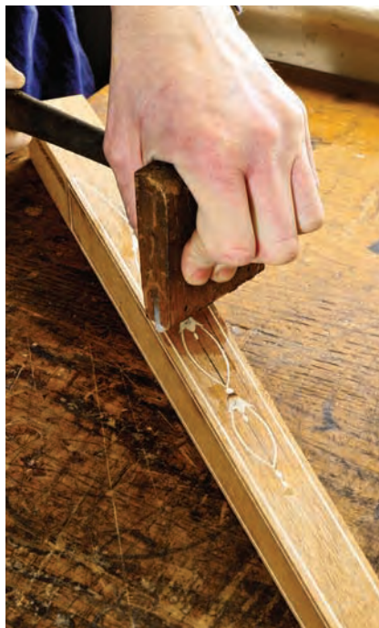
Choice of seating. The veneer hammer seats the bellflowers into position and removes any excess glue.
