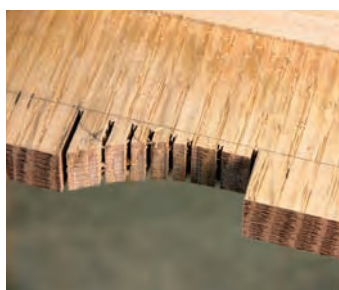
Swoop in. Remove the waste between the fingers in stages. Here's the first swooping cut.
