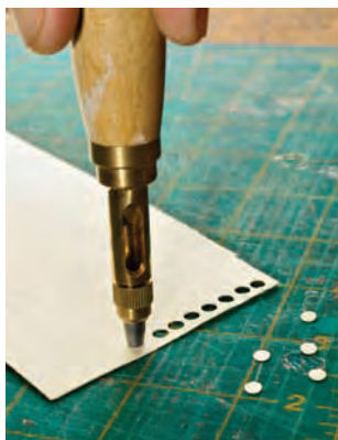
Repetition. A rotating punch quickly produces uniform dots ready for inlaying.
