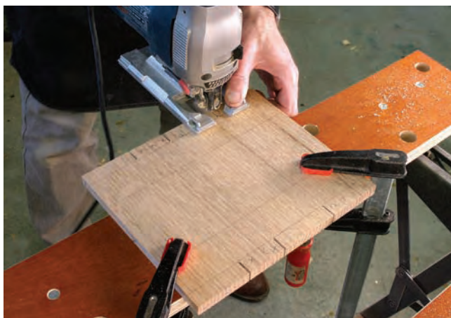
Short cuts first. Define the fingers of the joints with these short rips.
