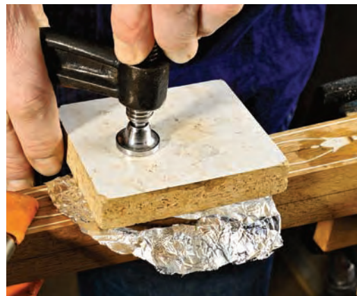
Climate change. Sometimes it's too cold for hide glue to bond properly, so a heated block is clamped over the bellflower, while aluminum foil keeps the block from sticking to the leg. In hot weather, the block is not heated.
