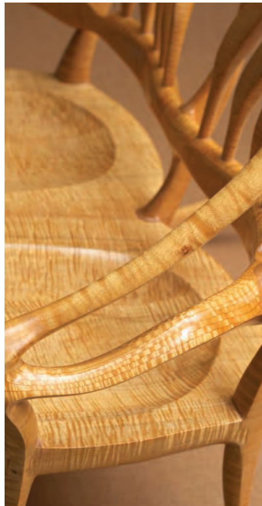
Right glue for the job. Rigidity is most important when working with bent laminations. Avoid glue “creep” by using a thermoset glue.
