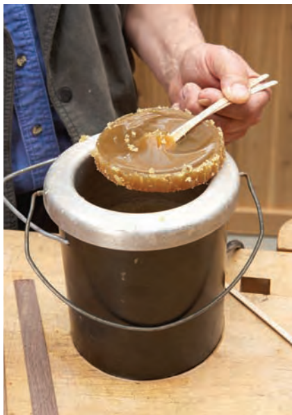
Thermal transformation. Many glues react to heat. Hide glue must be mixed with water, then properly heated before use. Below 110° F, a gelled clump can be pulled from the pot.
