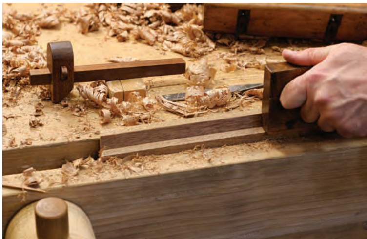
Skewed finish. A simple skew rabbet plane (a rabbet plane with an angled or "skewed" blade) quickly cleaned up the irregular surfaces from my chisel work.
