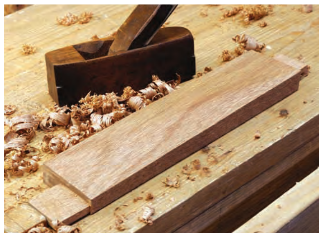
Smooth finish. I finished the outer face of the side rail with my smooth plane. I softened the line between the facets, and finished smoothing and fairing the rail to its adjacent legs.
