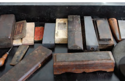
Sharpening station. One of the bay windows of the shop has a table with plenty of sharpening stones and natural light for sharpening edge tools.
