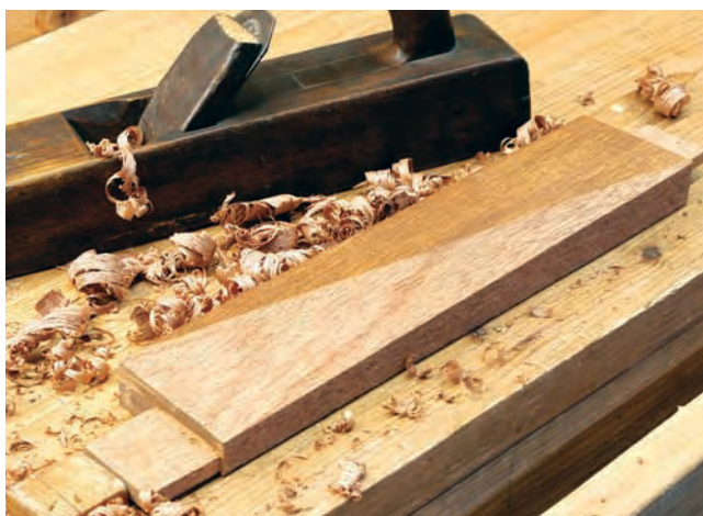
Bad bevels. I planed away the excess material using my trusty jack plane. The result is a beveled seat rail. If I left it like this, the different facets would catch and reflect light differently, drawing attention where I would not like it.
