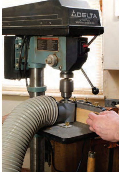
Get it right. A sanding fixture at the drill press produces a precisely thicknessed strip of wood for stringing.
