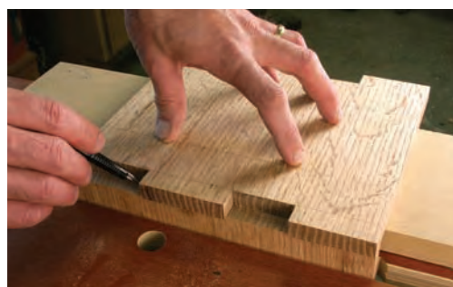
A little tracing. Use the cuts on the sides to mark the shape on the ends.
