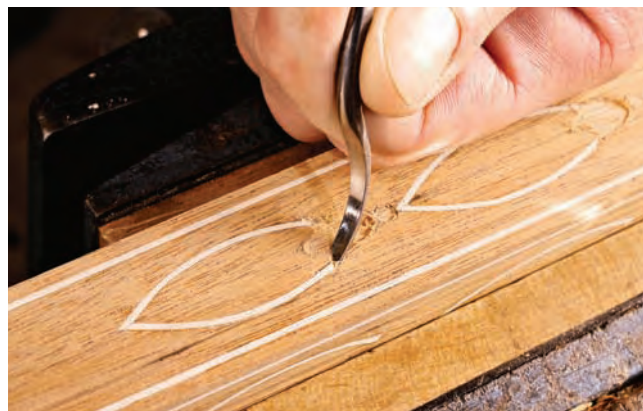
Dig into the corners. A skewed spoon gouge reaches into sharp corners and cleans out the recesses for the bellflowers without damaging an edge.
