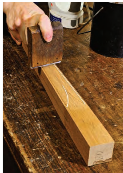
A softer touch. A veneer hammer works stringing into its groove with kid gloves.
