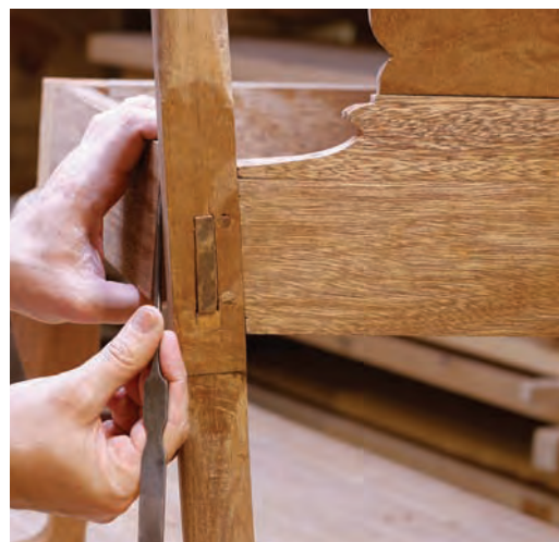
Fair the rail. The plumb side seat rail must be faired into the angled rear leg. I marked the intersection with my striking knife, in preparation for planing the excess material away.
