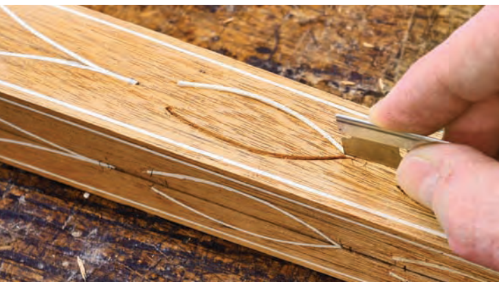
Odd woodworking tool. A razor blade becomes a handy tool to miter the bottom edge of the loops.
