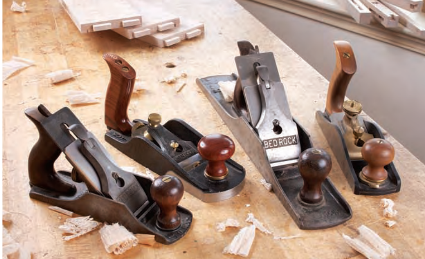
Up and down. Above are two new bevel-up smoothing planes from Lie-Nielsen and Veritas. The vintage tools are the older bevel-down style planes. Both designs flatten and smooth the wood – the differences are in the details.
