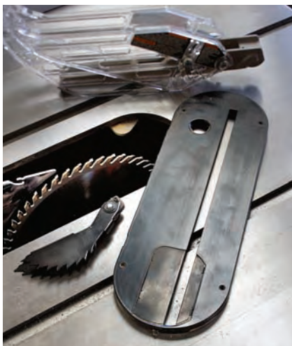
Added strength. The insert plate's continuous rim adds support, but requires that safety gear be pulled before the plate can be removed.
