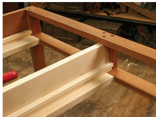
Details make the difference. The drawers ride on the rails of the web frame, and the guides restrain movement from side to side.
