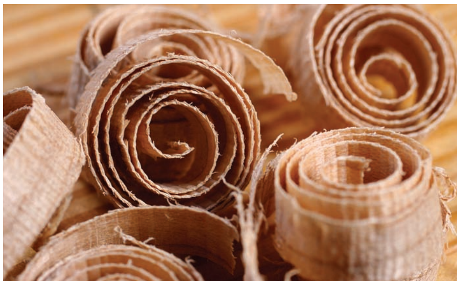
Superb spirals. The proof of the plane is in the thick, spiral shavings that peel off the board. You want to get the work done quickly, so a stable tool that can take a heavy shaving is a must.
