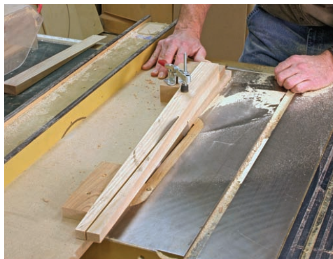
4 Turn for second cut. After the first cut is complete, turn the leg 90° and clamp it back in the jig.
