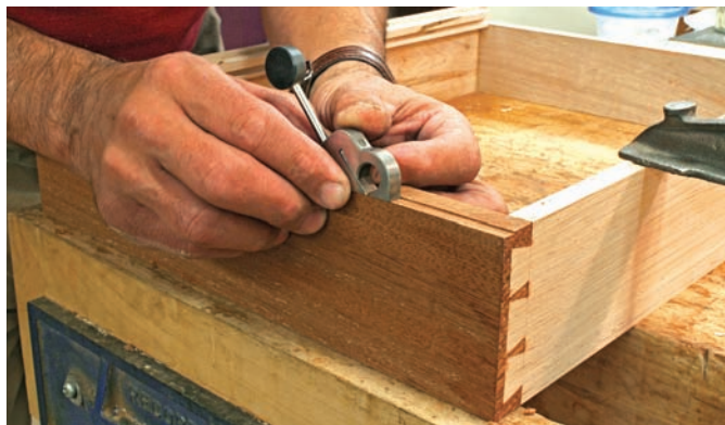
Rabbeted reveal. A small rabbet on the underside of the drawer front provides an even reveal to match the gaps at the top and sides.
