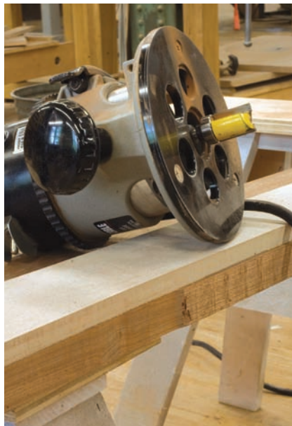
Size does matter. A \frac{3}{4} "-diameter flush-trim bit is perfect for trimming the workpiece edge flush to the curved pattern.
