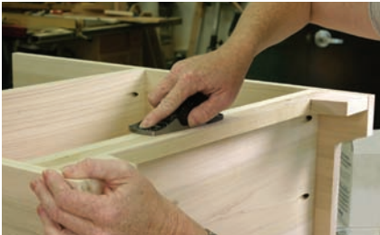
Plane to fit. If your apron and shelf aren't perfectly flush, a few passes with a block plane will even things up.
