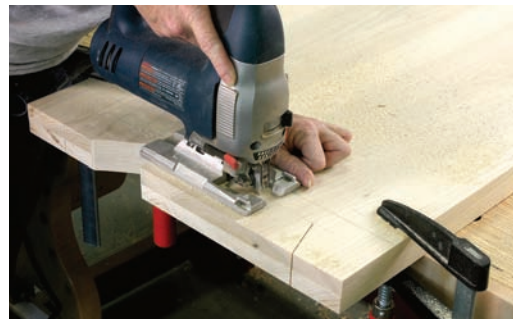
Mark, then cut. After marking out the shape of the feet on one side piece, clamp the two sides together, make a relief cut or two, then cut away the waste. I use my thumb as a guide, but you could clamp a straightedge in place to guide your cuts if you're aiming for perfection.
