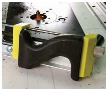
5 Round over. Place the tote blank in a small parts holder and use a roundover bit to shape the edges, then sand smooth.
