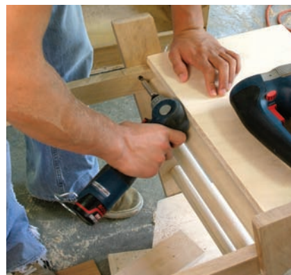
Quick assembly. A few screws in concealed locations hold the pieces securely together.
