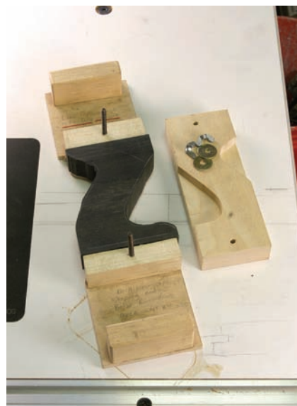
3 Now rout. After you've cut to \frac{1}{8} " outside your marked shape, reinsert the blank and rout to final rough shape.
