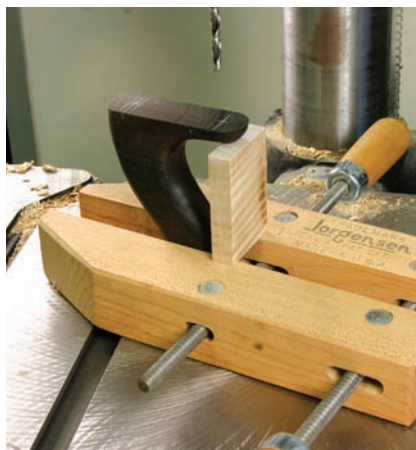
8 Support. Place a support block underneath as you drill the attachment hole in the back of the handle – otherwise, it could break off.
