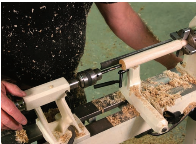
Dead center holes. The addition of a Jacob's chuck allows you to drill holes in the end of a spindle.
