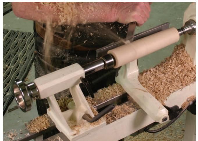
Live center. A live center with a ball bearing is one of the first accessories to get. It will reduce friction at the tail stock end.
