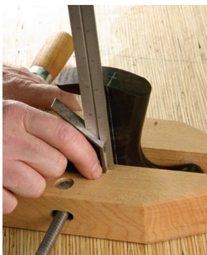
7 Handscrew helper. A handscrew can securely hold the workpiece at the required angle for drilling.
