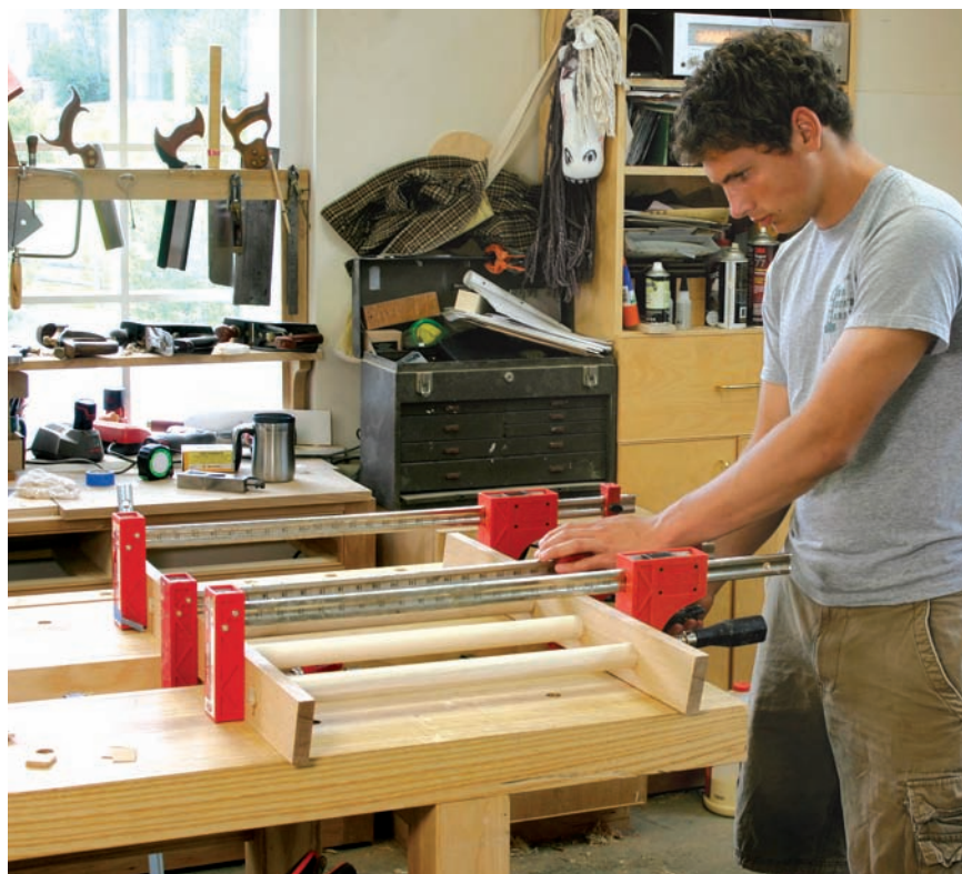
A reason to hide. I used liquid hide glue to allow more time to assemble the rungs and legs.
