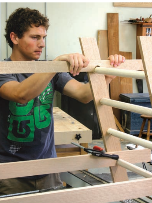
Notches are the key. The semi-circular openings in the bottom of the shelf rails line up all the parts and make assembly a snap.
