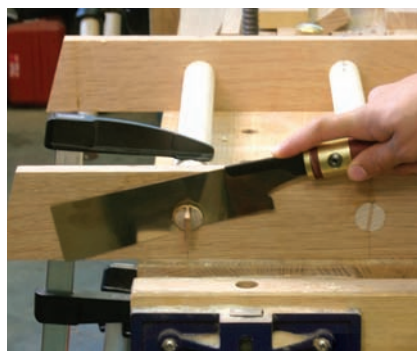
A little off the top. I made the tenons a little long, then trimmed them after assembly.
