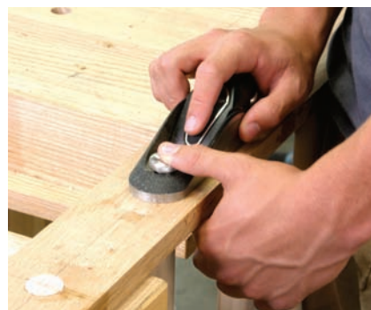
New block for the kid. A few passes with a block plane levels the ends of the tenons and wedges to the surface of the legs.
