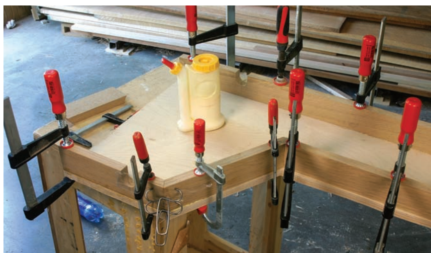
Cutting corners. The angled cutout in the bottom shelf provides some legroom as well as out-of-the-way storage.
