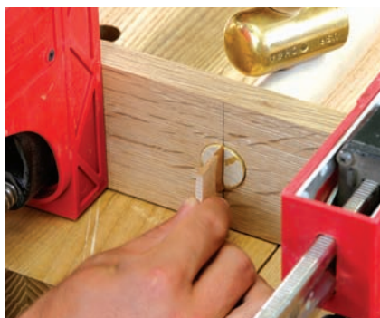
A short drive home. The wedges spread the ends of the tenons, making them tight in the mortises in the legs.
