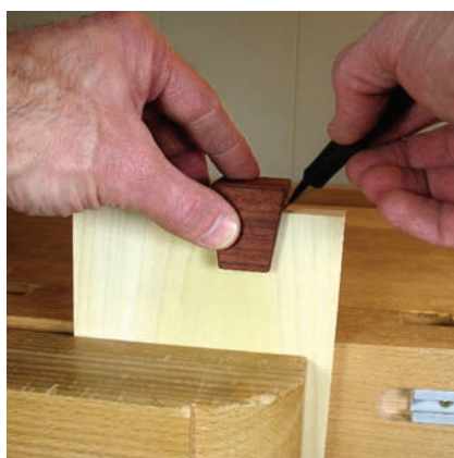
Dovetail marker. I've made dovetail markers in a range of ratios to suit the work I do most often.
