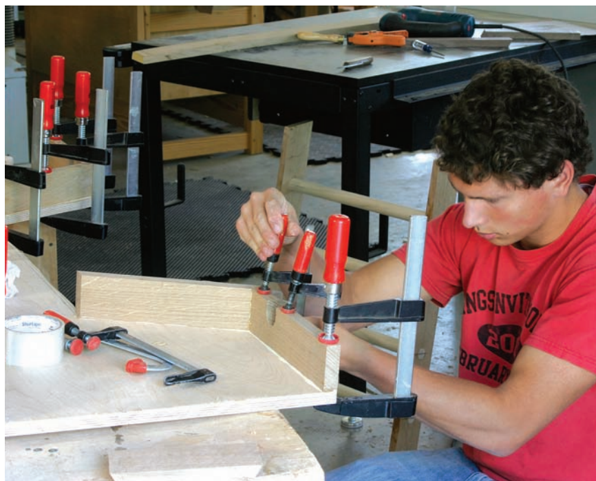
Glue is enough. The connection between the plywood and solid wood is long-grain to long-grain, so a glue-only joint will be solid.
