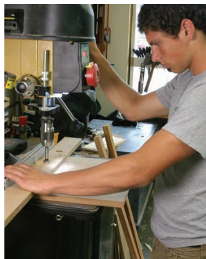
Holes in a row. Careful layout and setup of the holes in the legs makes for easy assembly and sturdy construction.
