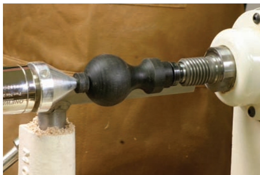
11 Almost done. For a clean look and feel, turn as close as possible on the top without parting it off, then remove the stubs with a fine-toothed saw.
