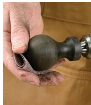
12 Screwed on. Use a ground-down flathead screw through the knob to secure it to the lathe for final sanding.
