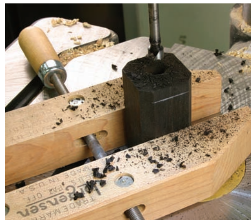
9 Prep your knob blank. Drill a hole that's a bit more narrow than needed – you'll enlarge the hole after turning the knob.
