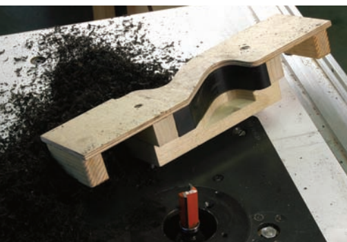
4 Rough but ready. This photo shows the tote after pattern routing is complete.
