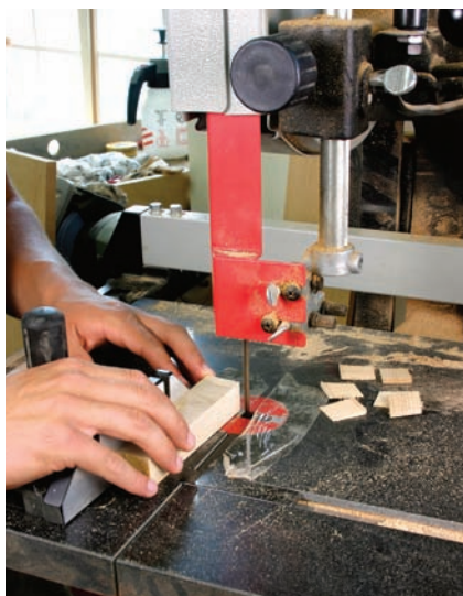
Flipping for wedges. The miter gauge is set at a slight angle, and the wedge stock is flipped over after each cut.
