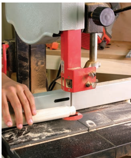
Across the grain. A band sawn kerf is cut in the center of each tenon.
