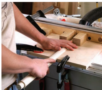
Take it for a spin. Tenons are formed on the ends of the rungs by rotating a dowel over the router bit.
