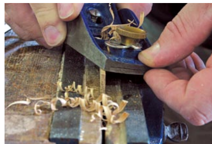
No fastener is required. The edges of the spring mechanism are planed to a dovetail shape to hold the spring in position as it's depressed. As pressure is applied to release the lock, the dovetailed sides push against the channel.
