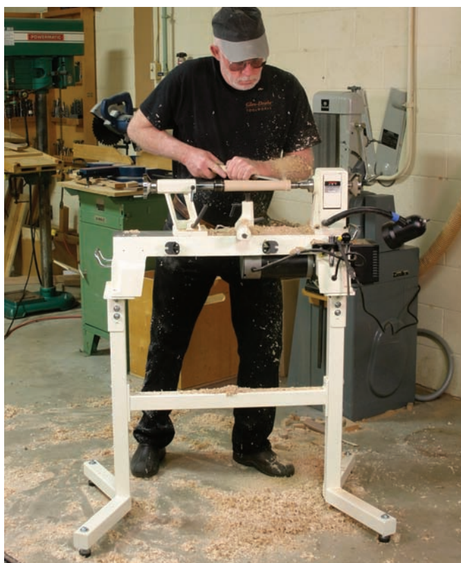
Small is good. Mini-lathes allow any shop to afford (and have room for) a lathe. Without the stand it can be stored below a bench.
