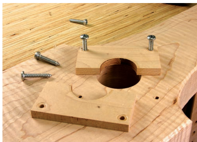
Garter, disassembled. To assemble the leg vise, drop the vise screw through the hole in the chop and fit the garter in its groove. Screw the garter pieces down and you're ready to bust some walnuts with your vise.
