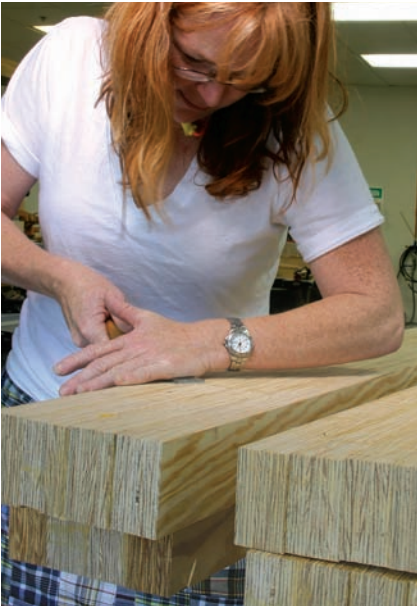
Scraping glue. After gluing up four strips into a chunk, we scraped off the excess yellow glue before dressing the lamination on the jointer. After all, the knives were already taking a beating from the glue between the plies so removing any glue we could was an act of kindness.
