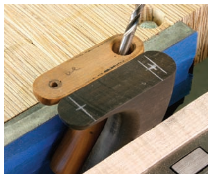
6 Work from the original. Use the original tote to locate the proper angles and holes for attachment.
