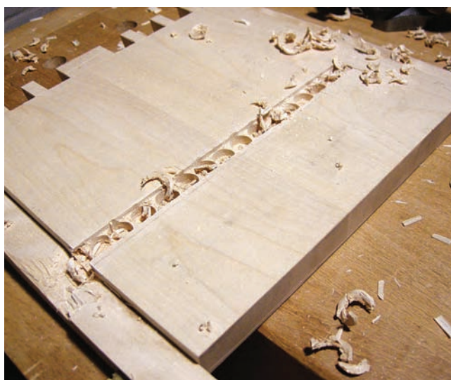
A bit of choice. You can use a bit and brace to remove the majority of the waste in a dado.
