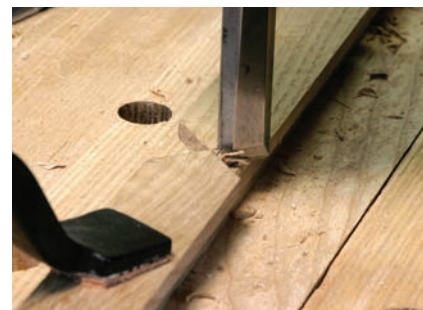
Cutting corners. The router will leave material in the corner, which can be removed with a chisel. The finished edges of the joint have been established with the knife and saw.
