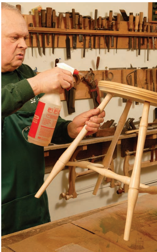
Spray. Moisten your workpiece surface thoroughly (but not so much that the water runs) to raise the grain.
