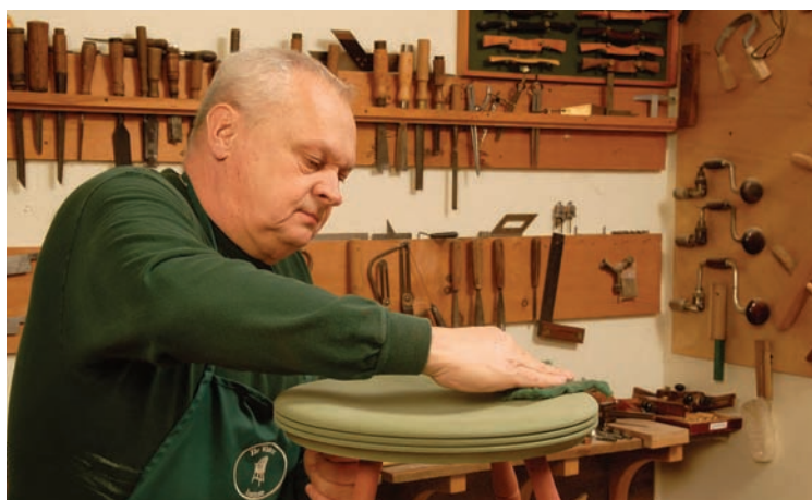
Smooth. If you want a smooth surface on your piece, after the first coat dries rub it down with #0000 steel wool, or a green Scotch-Brite pad.
