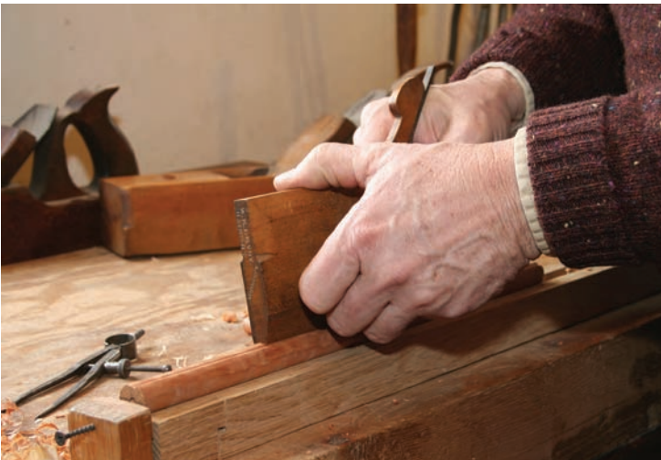
Fair curve. After paring away the bulk with a chisel, use a shoulder plane and \frac{3}{8} " hollow to fair the curve and create the locking shoulder.
