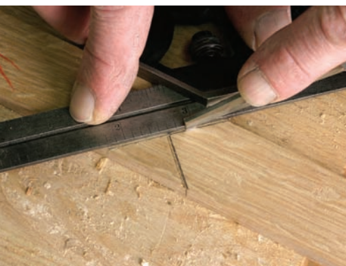
X marks the spot. The joints in the central mullion meet in the exact center. A knife cut along the lines will help to guide the saw.
