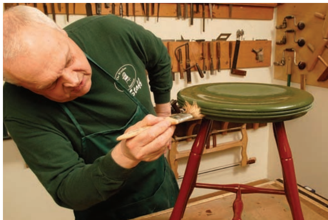
Topcoat. An untinted wiping varnish, applied liberally, will add a deep, rich look and luster, as well protect the paint.
