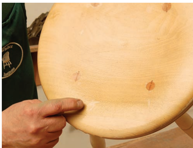
Glue alert. In addition to raising the grain, the water also highlights areas from which glue needs to be removed before painting.
