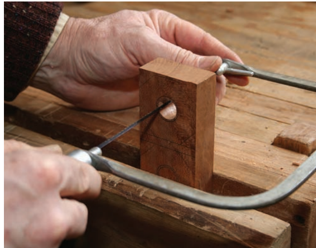
Cope. With a coping saw, make a kerf from 12 o'clock in your drilled hole outward to the marked circle.
