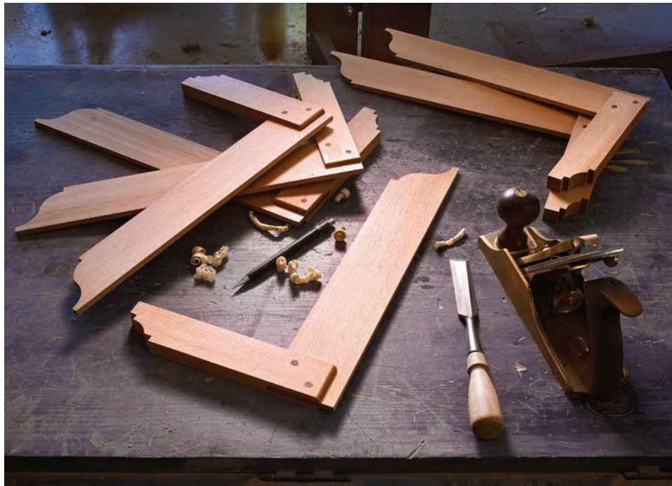
Built-in accuracy. Wooden try squares are more than accurate enough for woodworking. Plus they have other advantages – less weight and more reach.
