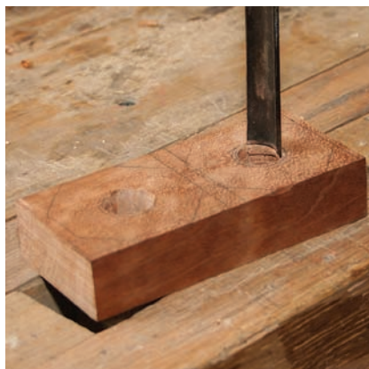
Gouge. Use an out-cannel gouge to create a fair curve from the smaller to the larger circle, to cut the shoulder that locks on the shaft.
