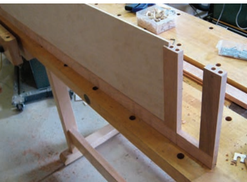
In the process. Here you can see a side panel being assembled. Glue at the joints is common, but a full bead around the panel is only used with plywood.
