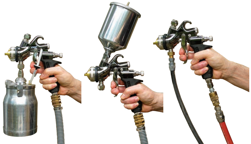
Three configurations. Spray guns are available in three configurations: siphon-feed with the cup under the gun, gravity-feed with the cup on top of the gun, and pressure-feed where the finish is fed to the gun through a hose connected to a separate pressurized pot. To illustrate the three configurations, I'm using the Apollo Atomizer spray gun, which is unique in that it can be set up in all three configurations and it can run off either a turbine or a compressor.
