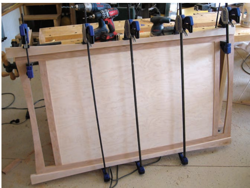
A strong hold. Long-grain-to-long-grain joints have plenty of hold once you get things located. A few well-placed dowels work wonders to align and reinforce the joint.
