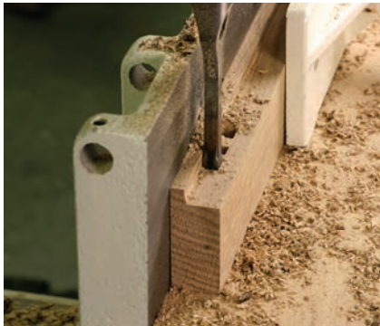
Simple setup. Set the fence on the mortiser by lining up the chisel with the back of the rabbet.
