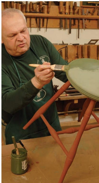
Second coat. The first coat seals the wood, so the second goes on more easily. But again, spread it evenly and thinly to avoid blotching.
