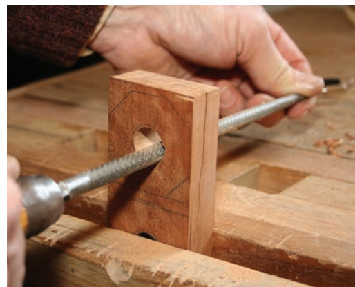
Smooth. Use a smooth-cut round file to smooth the interior of the gauge head so it rides smoothly on the shaft.
