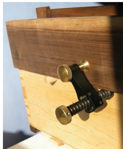
Field jointing. With the surface clamp in one of the front holes and a \frac{3}{4} " dowel in the other, I can edge joint a board up to 24" long!
