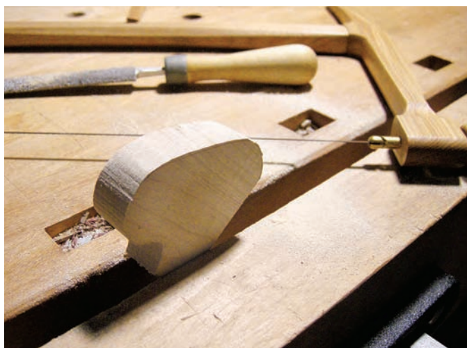
Trace. Here, I'm shaping one of two cleats that will become back saw holders. These were simply traced from my hand saws and cut out.
