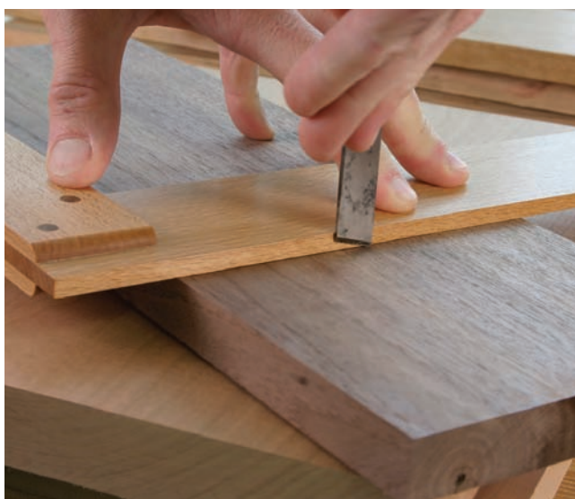
The right angle. The tip of my striking knife has an angle that suits a wooden square. A pointy-tipped knife would more easily slice the square.
