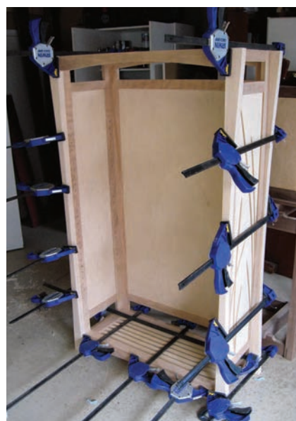
The case comes together. To fit the side panels between the front and back assemblies is not a challenge. But throw the case bottom into the mix and the balancing act begins.
