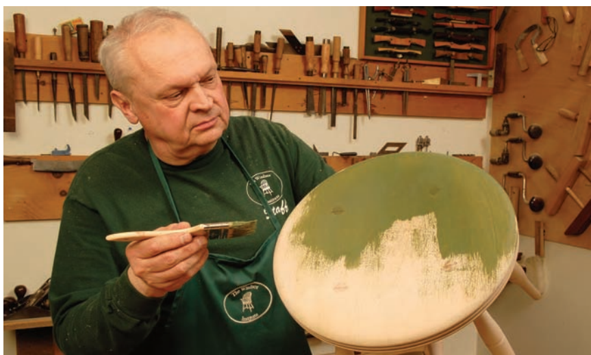
Thin coat. Apply a small amount of paint and pull it with the brush to a thin, uniform coat.
