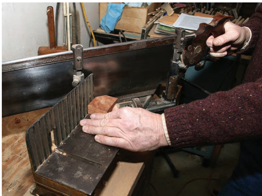
Perimeter. I use a miter box and saw to safely and accurately cut out the head, but a scrollsaw or backsaw also would work.
