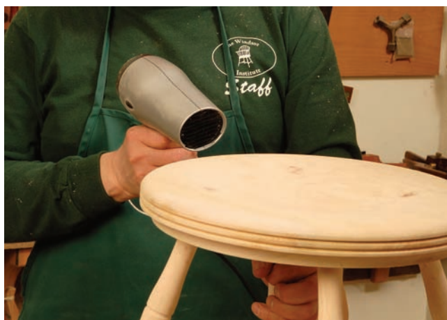
In a hurry. If you don't want to wait for the wood to dry, speed up the process with a hair dryer.
