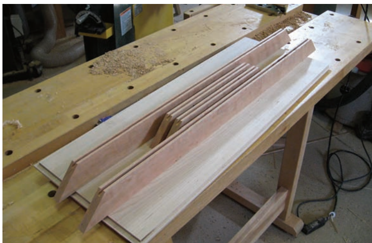
Keep them centered. The key to a perfect fit is to keep the grooves in the middle of the top's frame pieces, and to work with straight, flat material.
