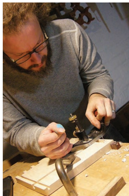
Clean up. A router plane completes the dado and cleans up the bottom.
