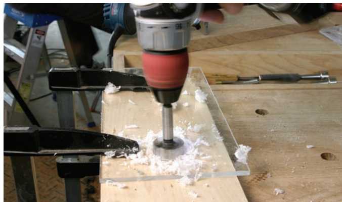
Big bit, same story. The larger bit clearance hole can be cut with a spade bit or a Forstner bit. A drill press is nice, but not necessary.
