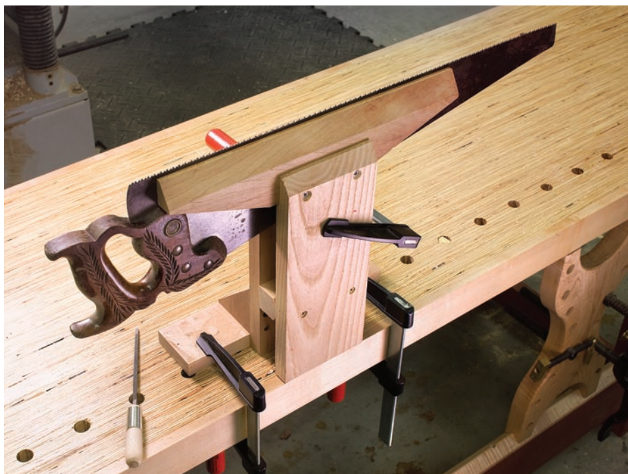
Hold it right there. Scrap wood and clamps, along with an hour or two of your time, provide you with the means to hold your saw steady and quiet while you sharpen.
