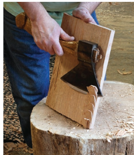
Hewing. Riven boards were further refined in thickness by hewing them with a hatchet. The tool marks are quite evident on period furniture.
