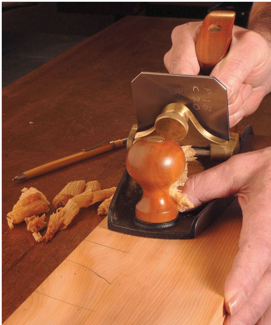
Getting you out of a bad scrape. Scraper planes are able to conquer unruly grain and maintain a flat surface. They are also ideal for dealing with veneer.
