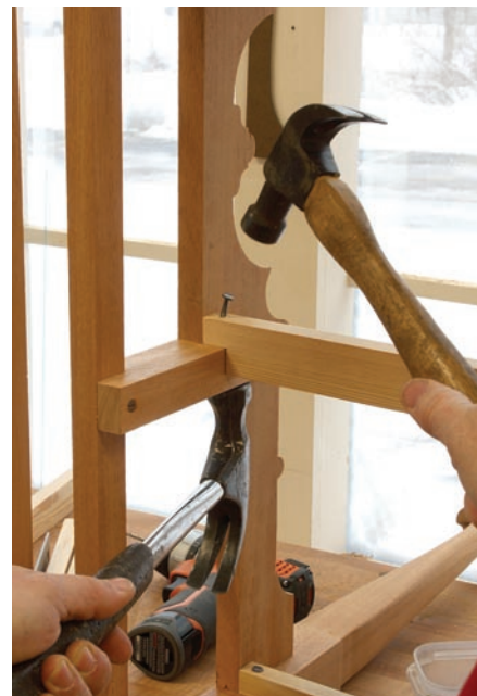
Absorb the blow. A second hammer placed directly behind the nail allows you to attach the runners to the dividers without problems.
