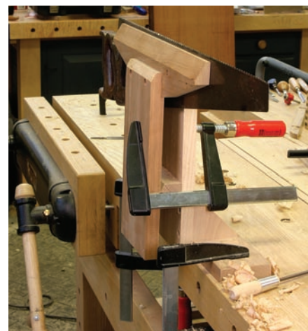
Three clamps. Two F-style clamps hold the vise to the bench, the third tightens the jaws. Keep the handle of the third clamp away from you.
