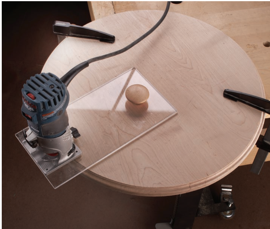
Quick fix. A custom-made baseplate provides a solid base for routing edges.
