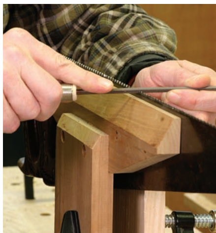
Tight fit. The jaws of the vise hold the sawblade and keep it from vibrating. If you hear an awful noise, the jaws need some work.
