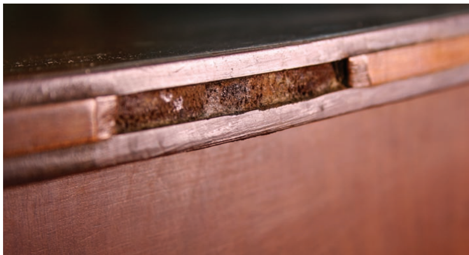
Missing tooth. The edge of this top is missing some of its inlay – a common form of damage seen on tops.
