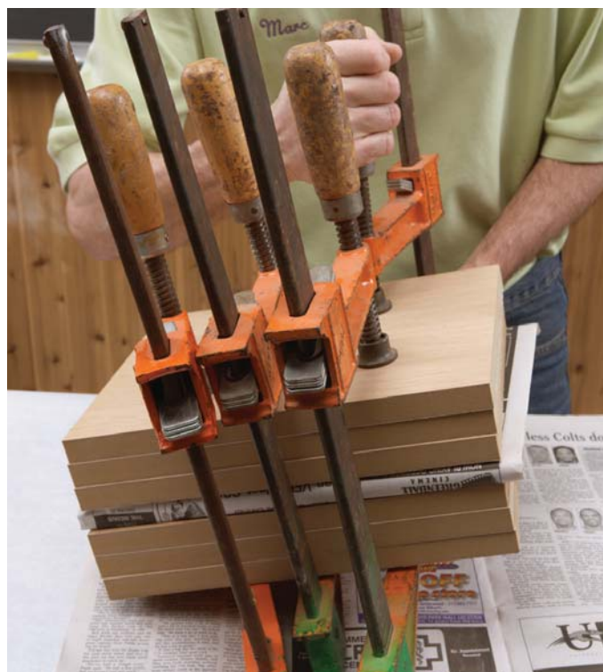
Calling all clamps. Then add clamps around the edges. The particleboard distributes the clamping pressure through the entire stack.
