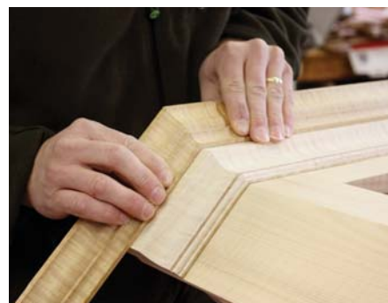
Many happy returns. When running mouldings around a cabinet, it is easier to begin at the front. Install the center piece first, then fit the returns to it.
