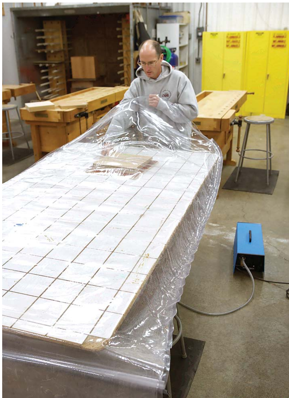
Under pressure. A vacuum press is a time-tested way to more easily make veneer work. You do need to be wary of the fact that the veneer bags suck the oxygen away from the glue.
