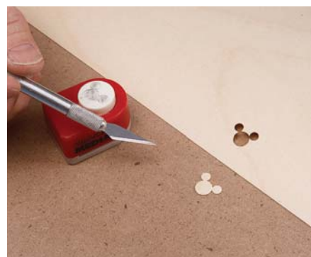
Feeling punchy? You will be surprised what you can do with veneer and a paper punch. It makes both the hole and the piece to inlay.
