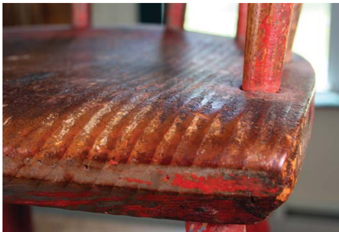
Almost erosion. This seat has seen so many backsides that the finish has disappeared and even some of the soft earlywood is wearing down.
