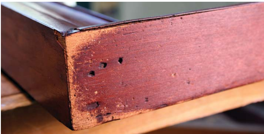
Sometimes you see it. This heavy mirror was occasionally dragged across the floor when it was moved, hence the wear pattern on the bottom edge of its frame.
