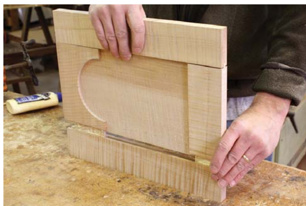
Don't sweat the glue-up. Because everything has been dry-assembled more than once, glue-up should go smoothly. Just remember to avoid too much adhesive squeeze-out on the face. It is difficult to clean up around the panel, which should not be glued to the door frame.
