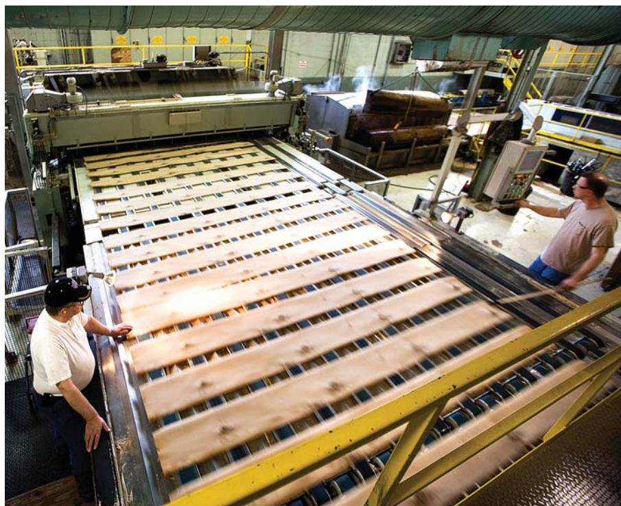
Almost done. Employees at Danzer Veneer in Edinburgh, Ind., inspect the leaves as they travel from the slicer to the be dried.
