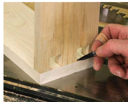
Balancing act. After cutting the first set of fingers, place the end of a side on the drawer front to mark the matching parts of the joint.
