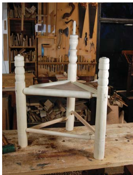
Staggering. While the seat rails are all on the same plane, the stretchers are not. So fitting both the top and bottom of the chair simultaneously can be a challenge (and don't forget to hold the seat panel in place, too).
