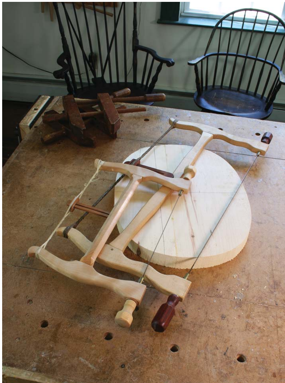
Bowsaws for the bench. Many modern woodworkers avoid bowsaws because they don't understand when or how to use them in the shop.
