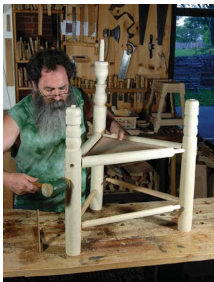
Test-fit. Each rectangular tenon is fully seated in its mortise. Here, I'm holding the seat in place in its grooves as I pound home the round tenons for a dry-fit.
