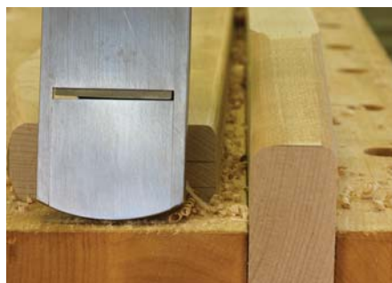
Why this slides. Opening the mouth of the block plane provides room to skew the iron.
