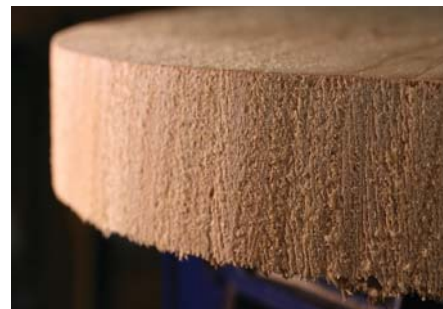
It tracks tightly. While the surface from a bowsaw might be rough, I find a bowsaw is easier to keep from drifting off line than a band saw.
