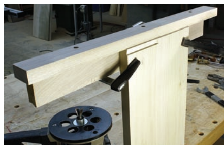
Double duty. This shop-made jig not only dials in a perfect sliding dovetail, it allows you to pull any warp out of your shelves.
