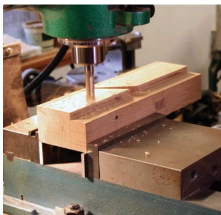
Machines help the hands. Here the Grizzly wood mill is milling out the hole for a depth stop on a moving fillister plane. While machines handle some of the operations, about 80 percent of the work is by hand.
