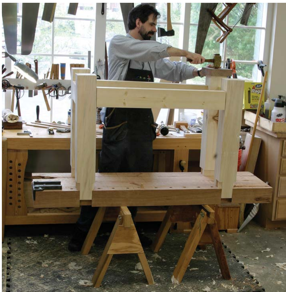
High and dry. When the bench parts finally go together, the result is remarkably stout, even without glue.
