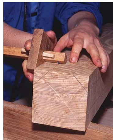
A workable road map. The octagon layout determines your chamfered corners, and the lines set with the marking gauge determine the final surface.
