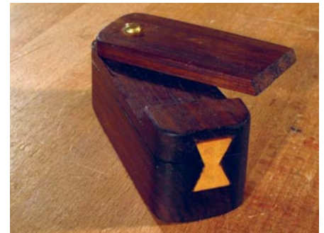
Lid 1. The first lid swings aside, but the inner lid seems trapped by the dovetail ...
