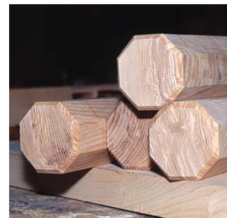
Dressed for driving. Chamfer the leg's bottom edges to receive the pounding commander. By not hitting the edge wood fibers, you will save the integrity of the legs.
