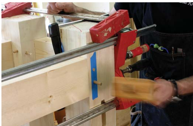
Clamps and drawbores. This might seem like wearing both a belt and suspenders, but it will reduce the number of splintered pegs.
