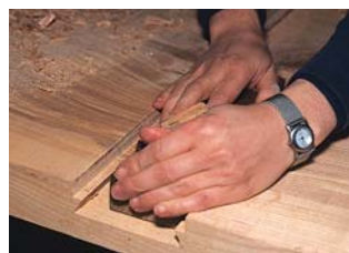
Smooth slides best. The bottom of the tapered pin groove is best flattened with a handplane.
