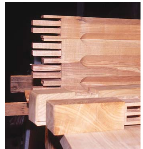
Eye-catching and strong. The mortise work for the leg-to-beam joinery is complex in design but uncomplicated to produce.
