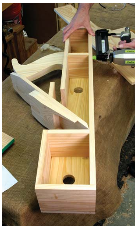
This plane is hollow. Glue and nail all the interior pieces as shown before you screw the second sidewall in place.
