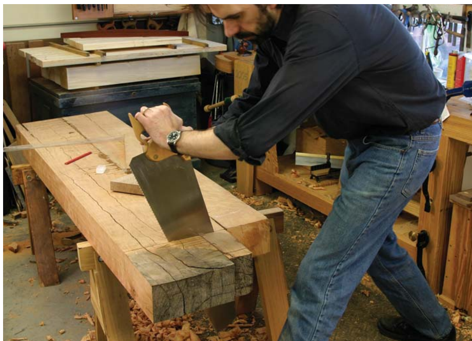
More than one way to cut a board. Handsaws are designed to be held in a variety of positions, including this one. This position uses different muscles than when you are cutting with the teeth facing the floor. Trying different positions will prevent you from tiring out as quickly.
