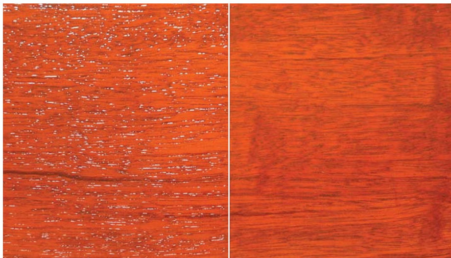
Unfilled vs. filled. The difference on a wood such as this unfilled mahogany surface (left side) and a filled mahogany surface (right side) is striking. The pores on the unfilled side break up the light creating a raw look. The filled side looks richer, deeper and more elegant.
