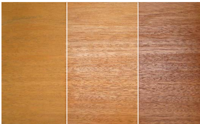
Before filler. The three situations for applying grain filler are (from left) over unstained and unsealed wood, over unstained and washcoated wood and over stained and washcoated wood.
