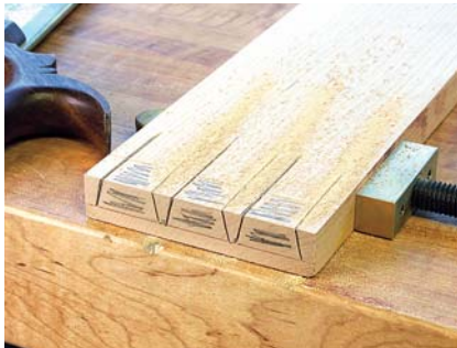
It's OK to miss this line. With the stock lying flat, make the cuts to define the pins for half-blind dovetails. Over-cutting the lines beyond the scribeline leads to easier waste removal.
