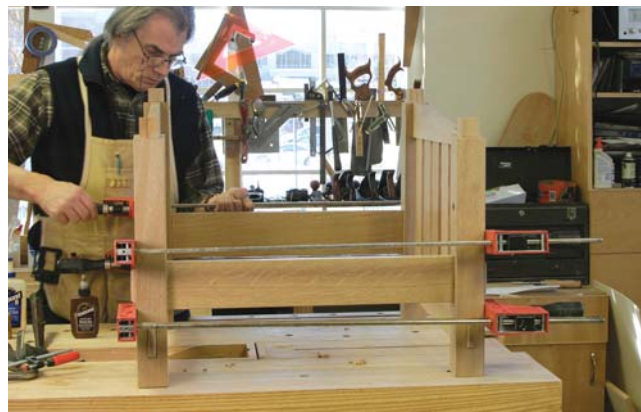
Only if you have to. Because the lower end of the vertical slats are angled, they only fit in one place. They can be adjusted with a tap or two.
