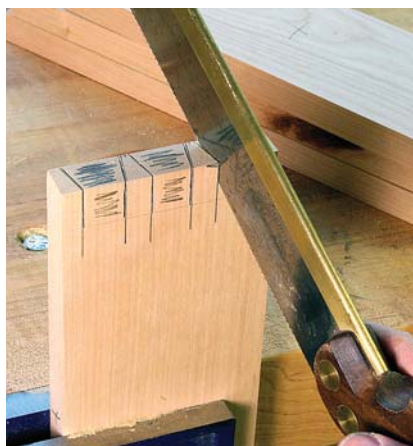
Waste side. The trick to accurate saw cuts is to follow both lines as you cut. Once you reach the scribeline, move the saw to perpendicular and it will follow the already-cut kerf.
