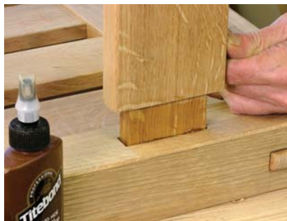
Control the glue goo. Start the through-tenon in the mortise before brushing on the glue to keep the end of the tenon clean.
