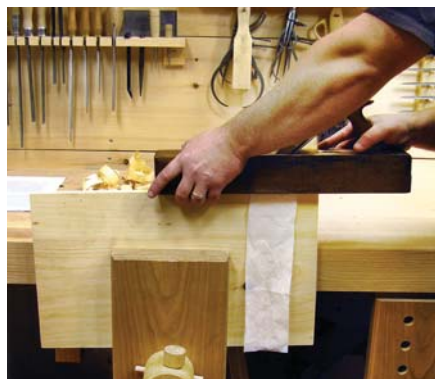
Balancing act. The iron acts as a fulcrum or pivot point because the sole is flat. At the start of the cut, the toe is down and the heel is up (left). Once the weight transfer is complete, the heel is down and the toe is up, as shown by the tissue paper slipped under the toe (right).
