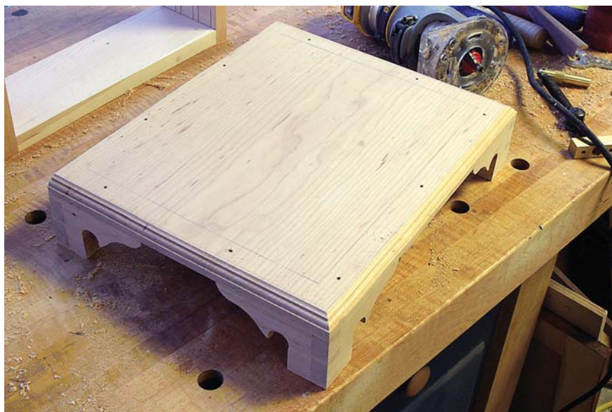
Planning ahead. Choose your edge profile carefully so your box continues to fit the base after the edges are moulded and make sure the pilot holes fit centered in the box frame.
