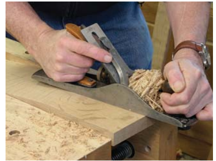
Smooth it over. Planing out the band saw marks leaves a smooth surface on the top and bottom of the arm.
