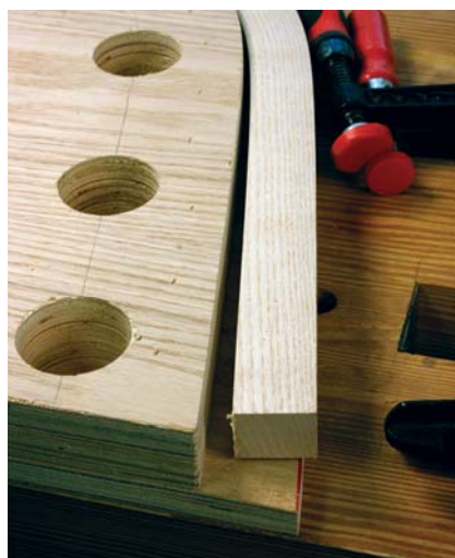
Relax(ed). One of my arm bows sprang out a little after being released from the form before the arm bow was completely dry. Back onto the form for you.
