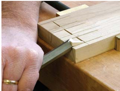
Up and at 'em. Remove small corners of waste to keep the pin corners from being fractured as you clean out the dovetail sockets.
