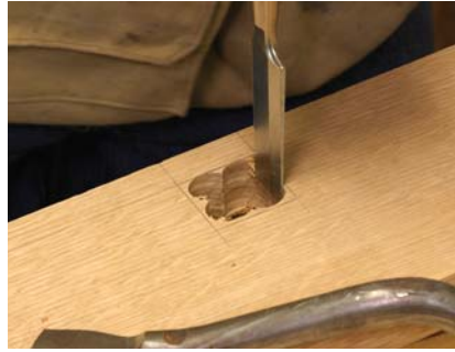
Pare to plumb. The same wedge is clamped between the arm and the bench to pare down the walls of the through-mortise.
