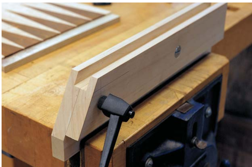
Miter jack. This fixture allows you to perfect the miters with precise control.
