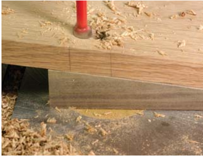
On the up and up. A wedge below the arm provides the proper tilt to keep the holes vertical.
