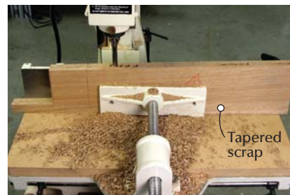
Keep your head straight. A tapered piece of scrap below the workpiece keeps the mortises oriented vertically.
