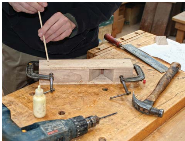
Dowel both sides. Two 3/16" pins on both sides will prevent movement under pressure. While two clamps hold the core blocks to the alignment board, drill 1 1/2"-deep holes for the pins, which are then cut off flush. Final clamping can be done in the bench vise like the 12"-wide one in the background here, or with clamps.
