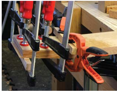
Get to the bottom. The wedge is glued to the underside of the arm, smooth face to smooth face.
