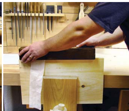
Balancing act. The iron acts as a fulcrum or pivot point because the sole is flat. At the start of the cut, the toe is down and the heel is up (left). Once the weight transfer is complete, the heel is down and the toe is up, as shown by the tissue paper slipped under the toe (right).
