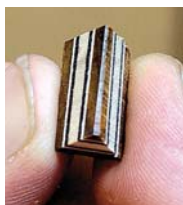
Trim the flat. The narrow band at the top edge represents the amount to be planed off the sawn face to end up with a perfect piece.
