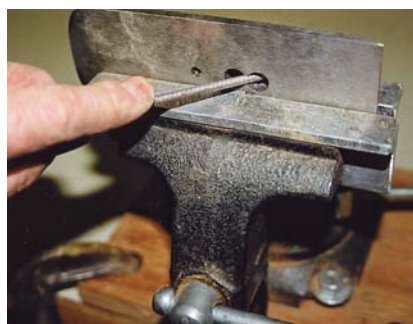
Blade beginnings. Making the blade begins with a \frac{3}{8} " slot and hole for the rest button. The 25° angle is ground and the top rounded.
