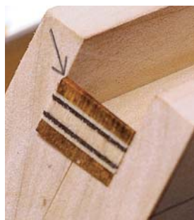
Jack be nimble. Align the inside edge of the flat with the face of the jack. You'll plane wood off the sawn face until you reach this edge. The result is a sharp arris along the top edge of the piece.
