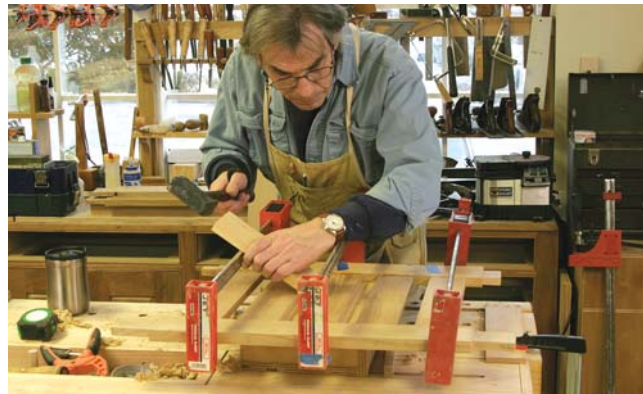
Only if you have to. Because the lower end of the vertical slats are angled, they only fit in one place. They can be adjusted with a tap or two.
