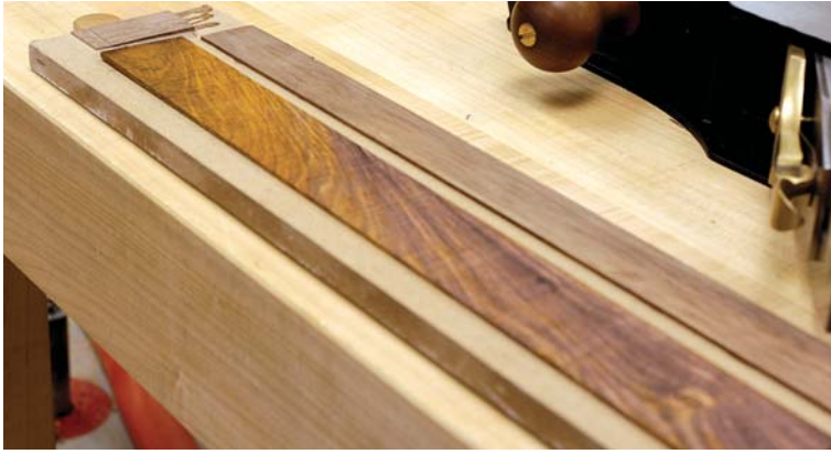
Planing board. A planing board allows you to plane stock down to crazy thinness with insane accuracy.
