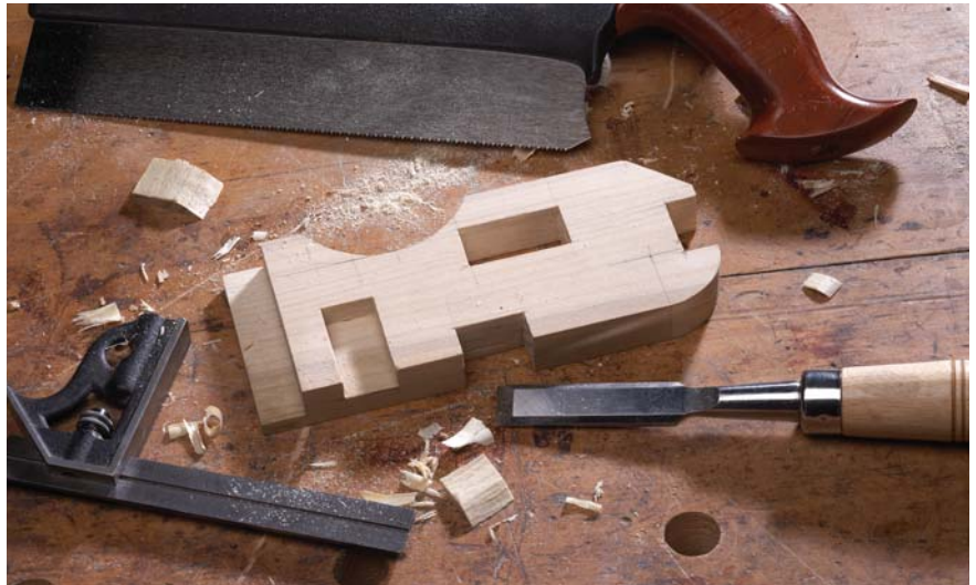
What's it for? This small block of wood has no useful purpose, except as an exercise in layout and cutting joints by hand. As a practice piece, it contains a series of valuable lessons.
