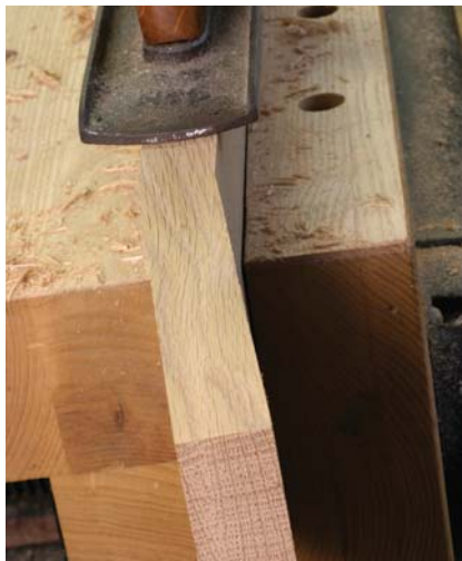
Nothing to see here. The glue line should disappear because the grain and color are the same in both pieces.
