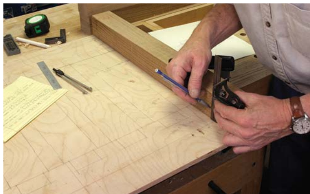
Measure once. A full-scale drawing provides a reference for most parts of the project. It saves time, and prevents measurement and layout errors.
