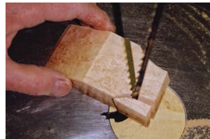
Screw. Cap is sawn and drilled for screw assembly.
