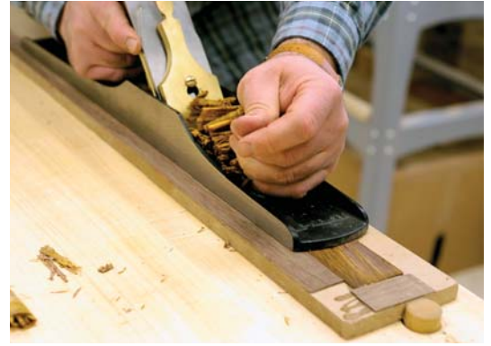
Micro from macro. Use your largest bench plane (here, a No. 7) to keep the thin board held flat while planing the wood to precise thickness.
