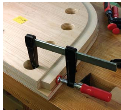
Flexible terms. Compwood can be bent without steam or—in many cases—a bending strap. It also can be bent in three dimensions.
