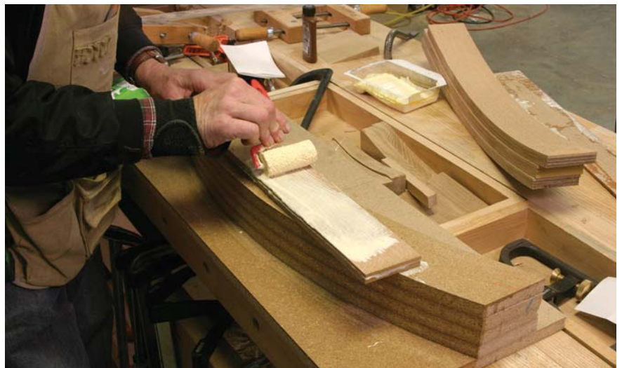
Work fast. Use a roller to spread glue on one side only of the laminations for the back. Keep the pieces in order and the edges will match.
