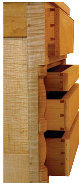
Large and small. This chest of drawers exhibits typical dovetails from American work with large tails and small pins.
