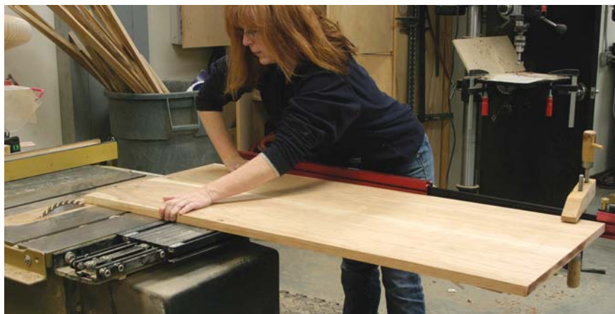
A helping hand. With a panel this long and no roller stand, it's helpful to have another person support the end of the board through the cut. But if another person isn't around to help, a handscrew attached to the crosscut sled will do (though you have to use more downward pressure to keep the piece flat to the saw table to compensate for some sag).
