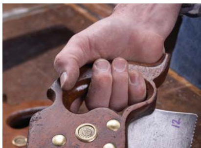
Comfort grip. Three fingers should fit comfortably inside the handle, and the horn should wrap around the heel of your palm.
