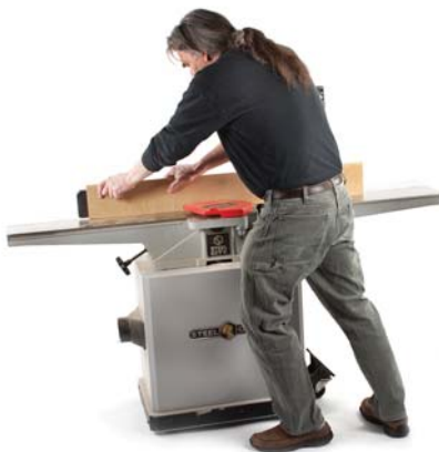
Power tools, too. Shifting weight to provide motion provides consistent control at the jointer, as the feet take a step and walk through milling an edge.
