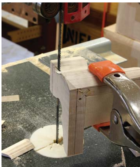
Scrap jig. I raided the scrap bin to build a jig to hold the feet for band saw shaping. The wider pieces at the bottom help stabilize it as you cut.
