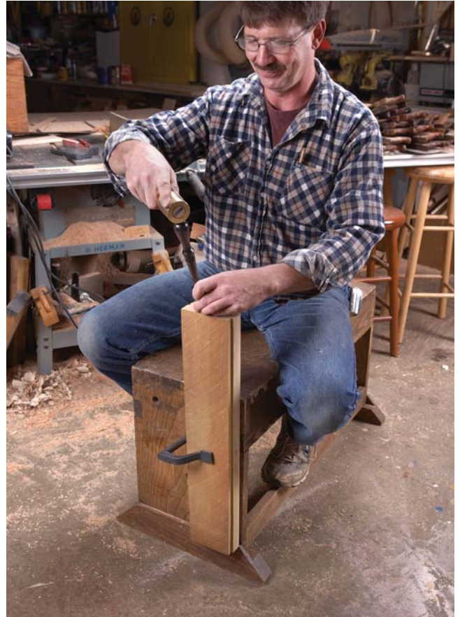
Lip service. With the ends attached in rabbets to the feet, there's a lip at the bottom that I can use to keep workpieces off the floor when I'm working on an end.
