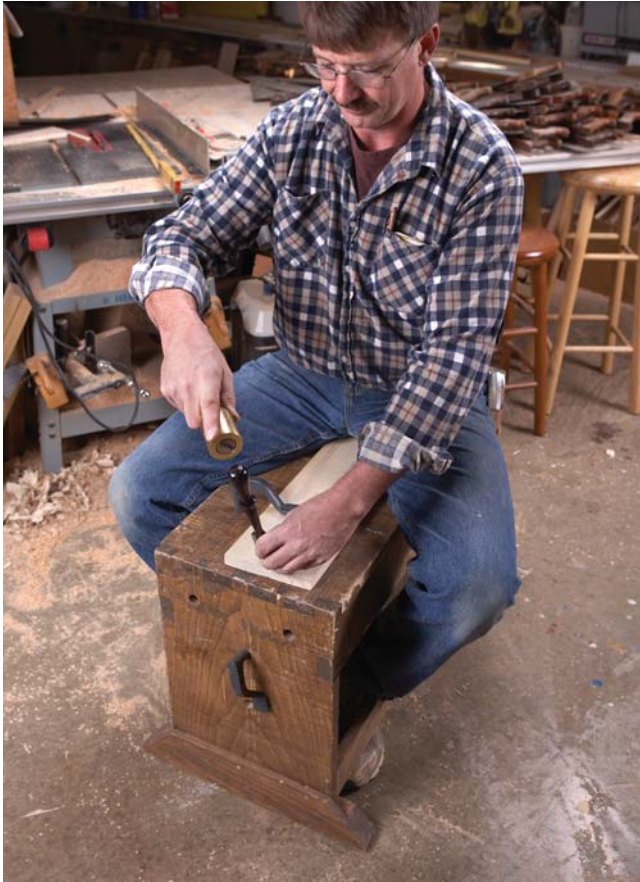
Toe jam. The lower stretchers are at the perfect height so I can jam my toes underneath to help keep my body in place as I work.
