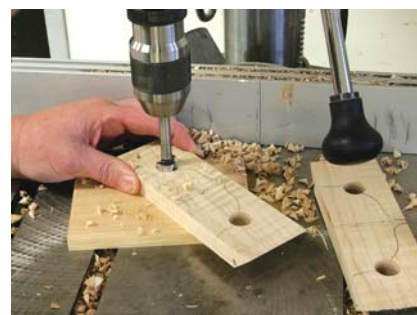
Stay connected. It's best to work on the feet while they're still in pairs. Separation comes at a band saw.
