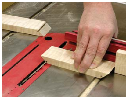
Set to 45°. Hold the \frac{1}{8} "-wide x \frac{1}{4} "-deep slot just off the back of the stock or you could expose the spline as you profile the feet.
