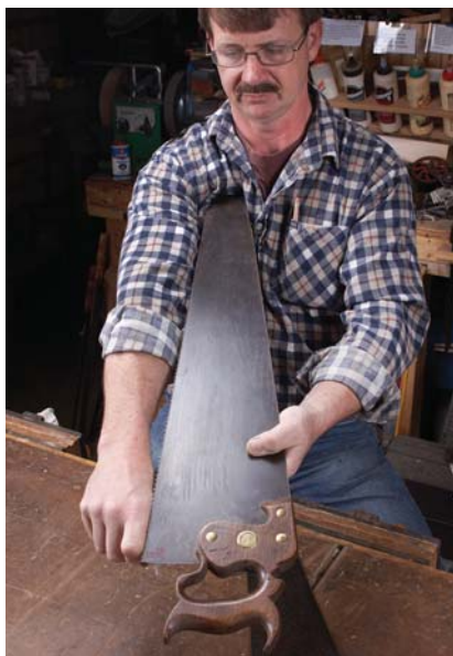
Perfectly sized. This picture illustrates the correct length of handsaw for me (it's 28"). Try this with your handsaws – but do it carefully (I'm assuming your saw is sharp!).
