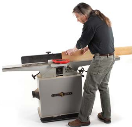
Power tools, too. Shifting weight to provide motion provides consistent control at the jointer, as the feet take a step and walk through milling an edge.
