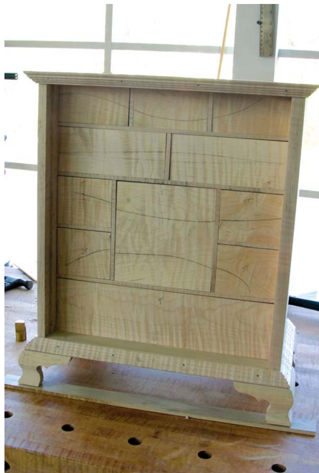
Plan your work. Drawers look best if the grain continues across the entire bank of drawers. Plan accordingly then mark the fronts to keep parts in place.
