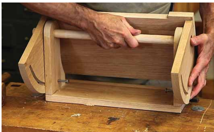
Make your table swing. The trunnion is merely a 1"-diameter dowel and is used to pivot the table on the fixed base.
