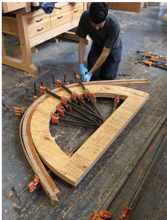
Practice first. Before you add glue, do a dry run to ensure you've enough clamps – and that when the glue is on, you know where to place them.
