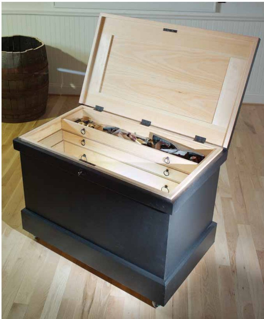
A box chock-full of tradition. This tool chest, which was designed from time-tested examples, holds every hand tool you need, protects those tools from dust, and keeps everything just one hand motion away.
