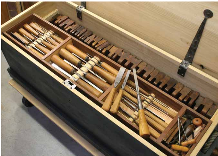
Choice. Eighteenth-century craftsmen typically had different styles of chisels than we do, and in greater numbers. Maybe it's time to reconsider our views on the most basic woodworking tool.
