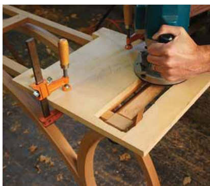
Plane truth. This jig provides a flat surface for the router base, bringing the front-to-back rails and the tops of the wings flush with the aprons.
