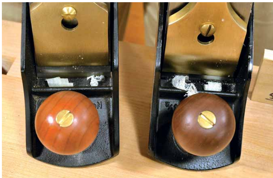
Test. In the plane on the left, you can readily see that the two test shavings are different thicknesses; this tells you the blade is not parallel in the plane's mouth. On the right, the two shavings are the same thickness, which indicates the blade is properly aligned.
