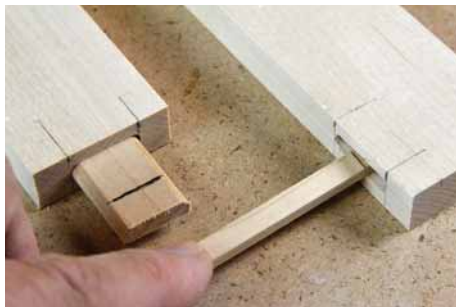
Story stick. Used to probe the depth of the mortise, the story stick is then used to transfer that measurement to the tenon. Cut the tenon a little shorter than the mortise depth.
