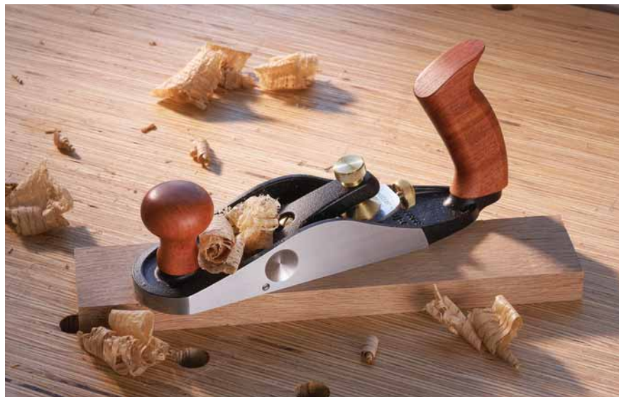
Perfectly sized. Small smoothing planes will get you to the finish line faster than big ones. The new Veritas bevel-up tool is both easy to set up and use.
