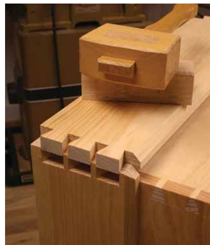
Not mitered. Dovetail your skirt and dust seal to the shell to ensure they stick around. Literally.
