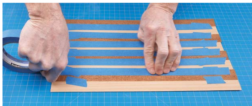
Don't skim on tape. Make sure the seams are tight and that the masking tape covers the entire length of the seam. This will create a packet of several taped strips.
