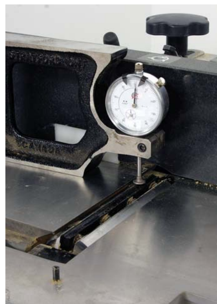
Goodbye micrometer. The tediousness of dialing in the perfect setting as you change traditional knives is eliminated when using a stagger-tooth cutterhead.
