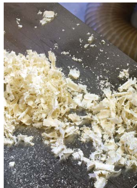
Appears the same. At first glance, shavings from the straight-knife stagger-tooth setup look like those from the shearing cut, but there is no curl in this waste.
