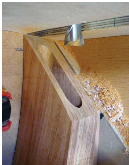
Clean mortises. A two-flute aluminum cutting end mill, when mounted in a plunge router, cuts a clean mortise. These bits are inexpensive (approximately $12) and are available from machine tool supply companies. Avoid three- and four-flute bits – they don't like to plunge cut.
