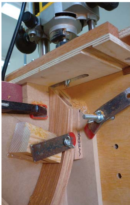
Bottom up. Here is an underside view of the shop-made mortising jig with the miter saw cut-off jig and curved part clamped in place.
