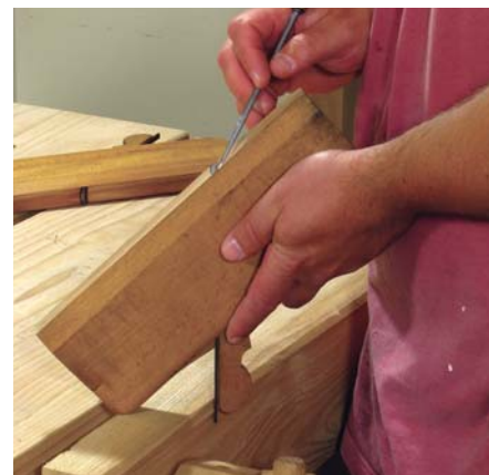
Transfer the profile. I use an awl to transfer the shape of the sole to the layout dye on the face of the iron. Grind the edge blunt down to this line before grinding the bevel.
