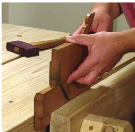
Plane the plane. The hollow is the negative of the matching round, so it can be used to true the sole of the round. Make very light passes to avoid planing too much and recheck the sole of the round often.
