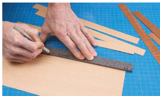
Simple strips. Make sure you are not cutting strips longer than your straightedge. My strips are about 12" long.
