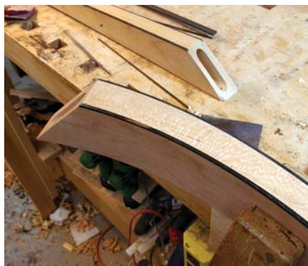
Inside, then out. The inside corners are done first.
