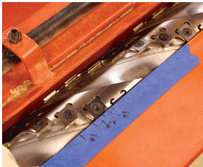
Unique knives. Evaluation of the knife locations on a stagger-tooth head shows no overlap in the cut, but hides the fact that some knives line up.
