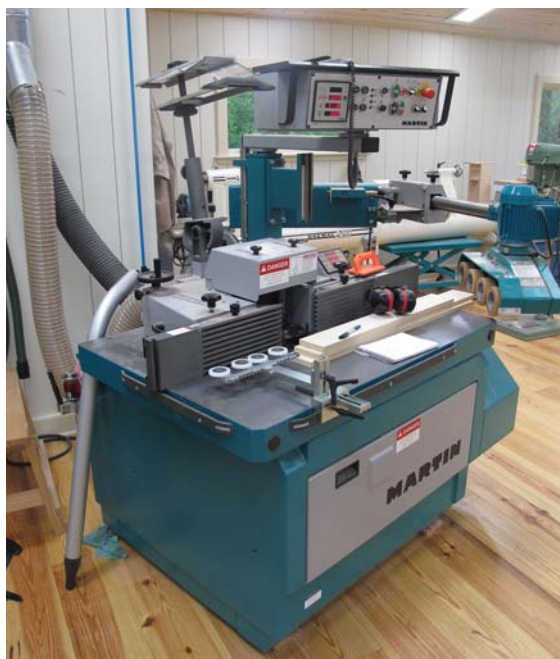
A shapely shaper. This Martin shaper makes smaller machines look like toys. It features a head that can tilt both ways.
