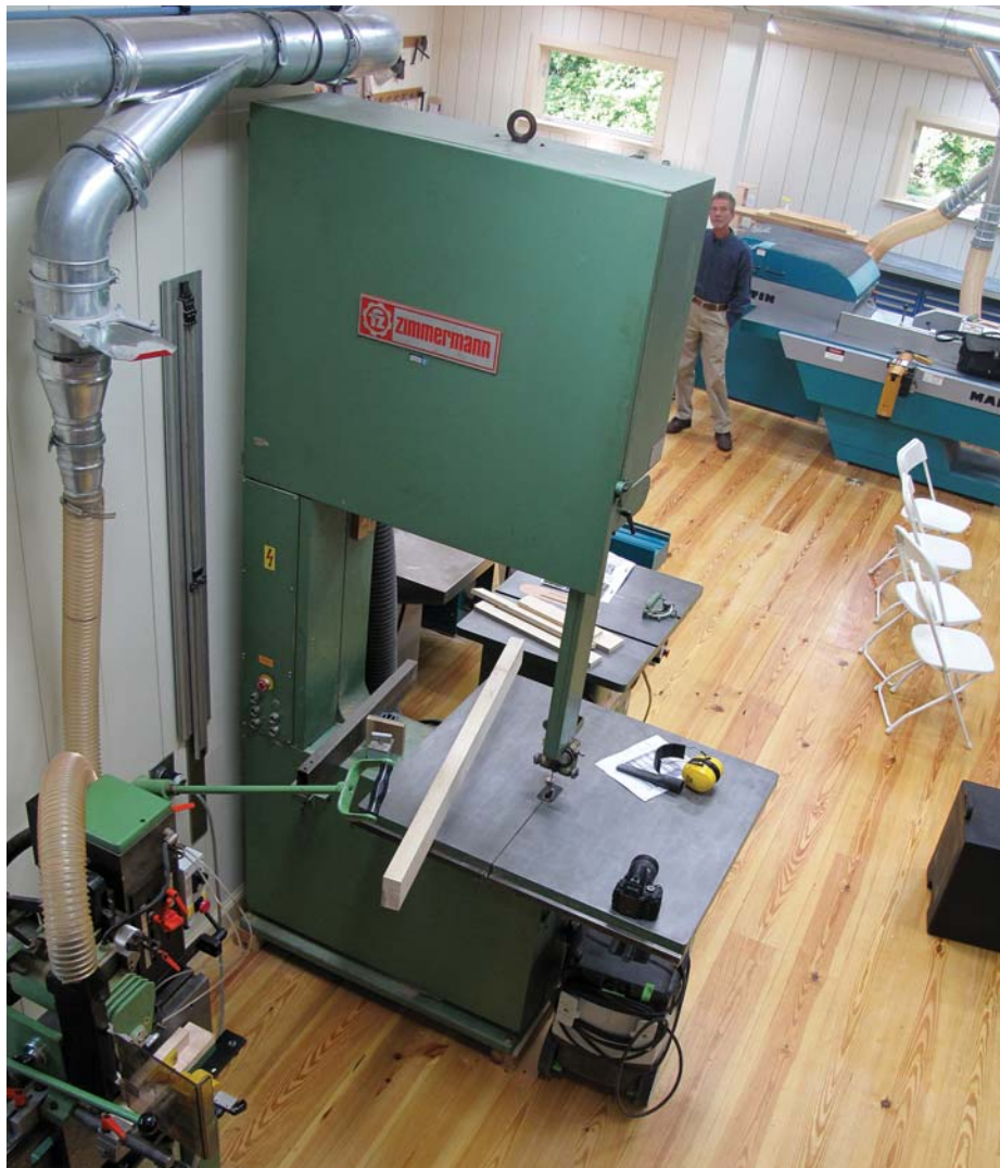
The other green giant. At 9' tall, this Zimmermann band saw has more than twice the throat capacity as a typical 14" home shop band saw.
