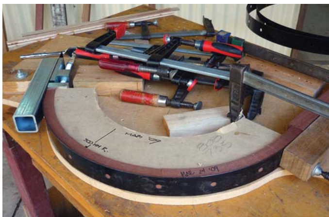
Compression strap. The end stops bolted to this Veritas compression strap stop the wood from stretching and failing. The inside face must be put into compression for successful steam bending.
