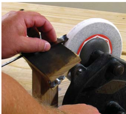
Radiused wheel makes grinding a breeze. I used a wheel dressing tool to round this \frac{3}{4} "-thick grinding wheel to about a \frac{3}{8} " radius. This allows me to grind hollow irons down to about \frac{1}{2} " wide. A \frac{1}{4} "-thick grinding wheel handles smaller irons.
