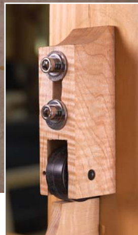
Smooth operator. The Glide is modeled after a traditional leg vise, but the 8" wheel and two roller brackets work in tandem to make it move in and out quickly and smoothly, and cinch hard with little user effort.
