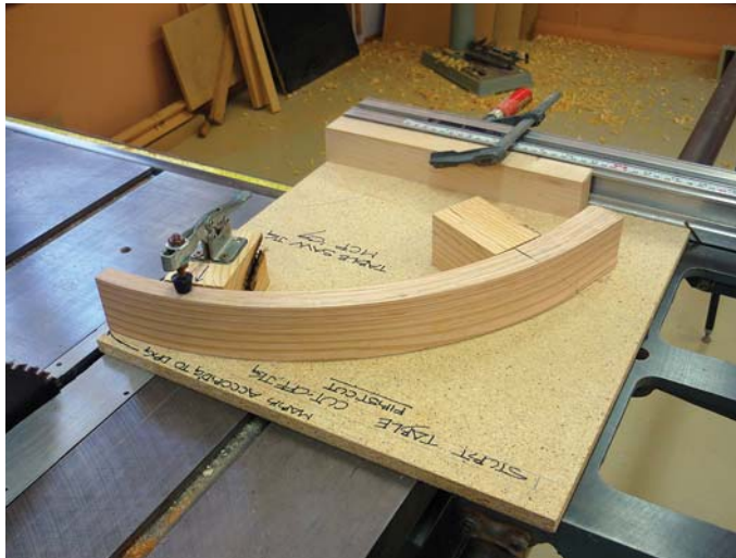
Cut-off jig. This table saw cut-off jig ensures the small end is cut square to the curve where it intersects a second rail.
