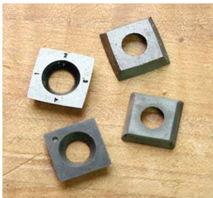
Choose wisely. These knives are different in size and thickness, and the larger knife's edge is sharpened at a curve.
