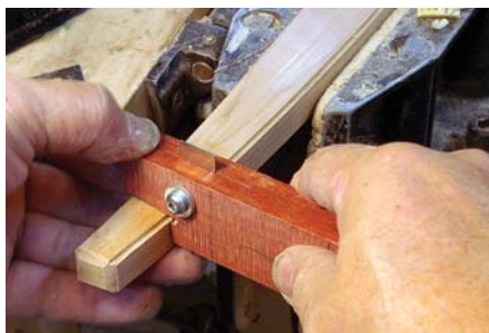
Shop-made rabbetting tool. Some of the edges aren't square where they intersect concave and convex surfaces. I've mounted small pieces of tool steel in hardwood blocks that mimic the angle at these edges to form the rabbets.
