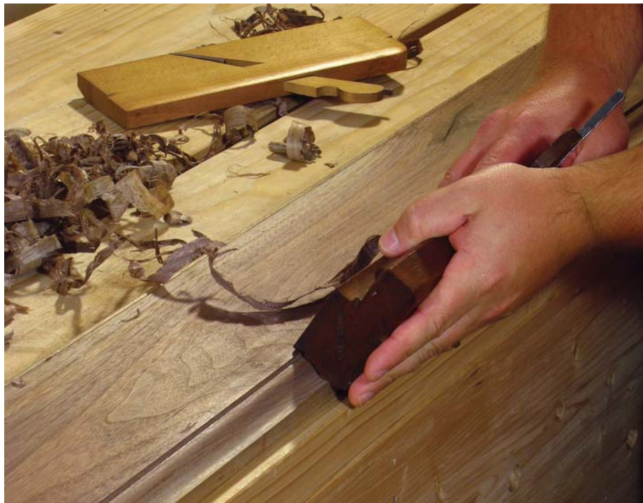
Plane and simple. Make some mouldings with a well-tuned plane and you'll wonder why routers were ever invented.
