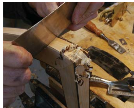
Don't sand. Use a card scraper to flush the ebony. Avoid sanding, as the dust would contaminate the surrounding light wood.
