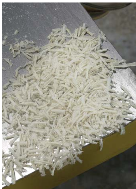
Clog-free collection. Stagger-tooth cutterheads produce shavings that are only as long as the small knives. That's also an indication of why tear-out is minimal at worst.
