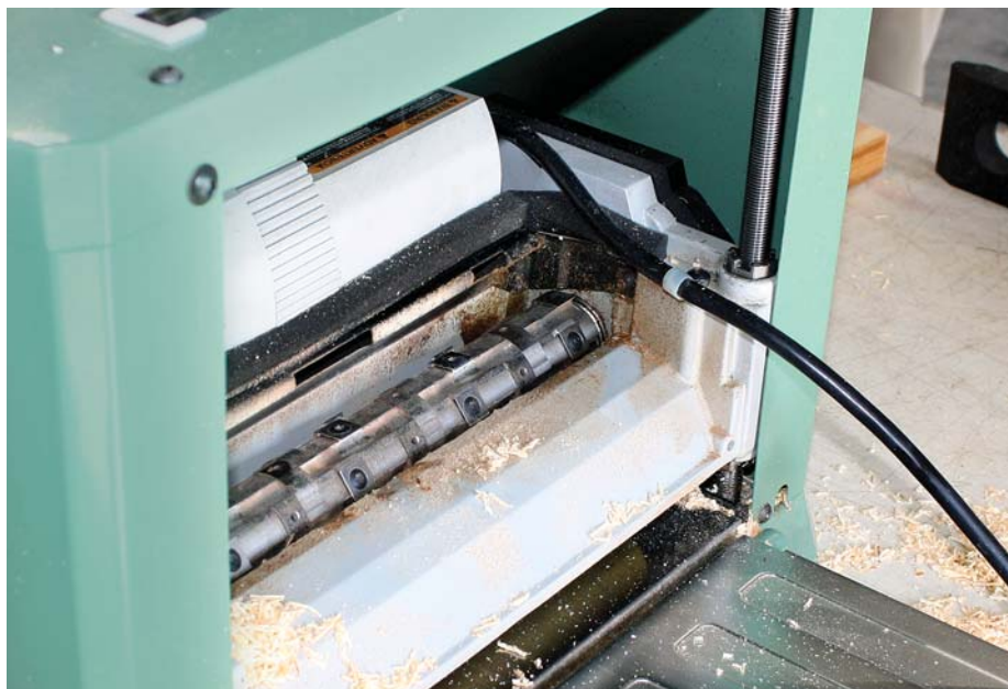
Also a stagger-tooth. This segmented head (the entire head is made up in sections) is another stagger-tooth variation in which the knives meet the workpiece at 90°.
