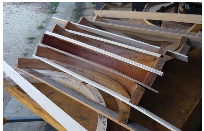
Two parts at one time. The parts are removed from the bending form after sitting for 10 minutes and are restrained with a wooden tie bar. They will acclimate to the curve in about seven days. Here are various air-dried woods that have been steam-bent.
