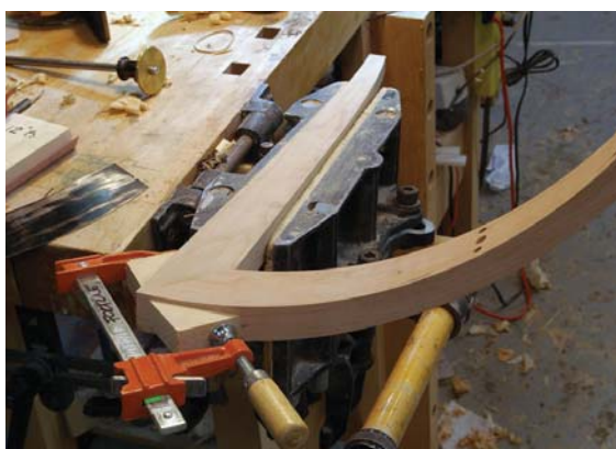
Curve transfer. The concave curve of the apron is transferred over to the leg.
