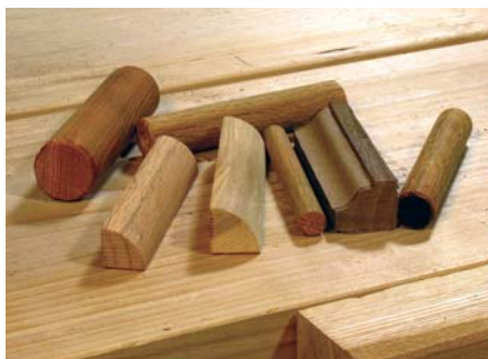
Hardware store fix. I use a selection of dowels and other profiles to correct my planes' soles. This works for hollows and rounds, as well as more complex shapes.
