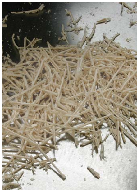
Looks like straw. Shavings from a three-knife head can be as long as your workpiece is wide. That's a surefire recipe for clogged dust collection.
