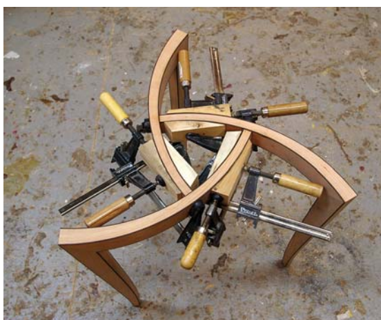
Cauls. Clamping cauls faced with #100-grit sandpaper are clamped to the curves. The clamping pressure must always be perpendicular to the glue line.
