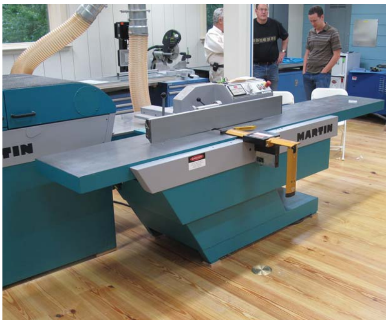
How wide? This Martin jointer can handle boards up to almost 20" wide.
