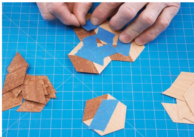
Tape it tightly. Tape at least three Louis cubes together and set that aside. Do not use veneer tape yet, because the water will cause each piece to curl which would affect the next few steps.
