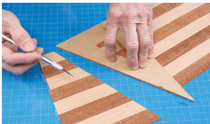
One angled cut. This cut will be across the grain of the entire strip packet and will require several passes with the knife.
