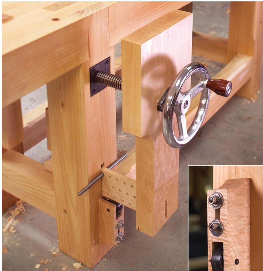
Smooth operator. The Glide is modeled after a traditional leg vise, but the 8" wheel and two roller brackets work in tandem to make it move in and out quickly and smoothly, and cinch hard with little user effort.
