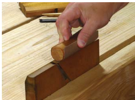
No bananas please. Use light pressure and check the profile and straightness often to avoid making the sole convex. Pencil lines help gauge your progress. The finished profile should match the dowel curve and be straight from heel to toe.
