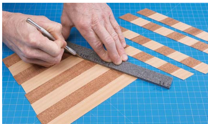
Back to the straightedge. Cut several strips with your knife and straightedge. Take care to ensure the strips are the same width as your straightedge.
