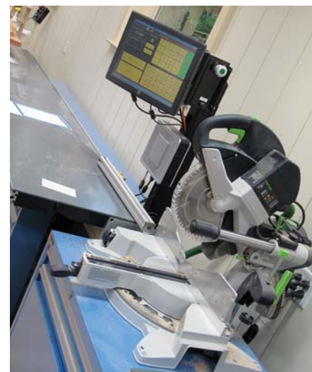
Finely chopped. The computerized RazorGage stop system on this Festool miter saw setup makes cutting stock to length a breeze.
