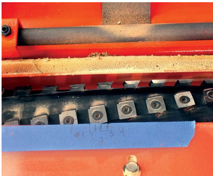
Single-effective. The Byrd head has the knives set so that each takes a slice of wood. Overlapping of the cuts is about one-third.
