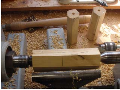
Pin hole. Drill a 9/32" hole in one end of each handle blank.
