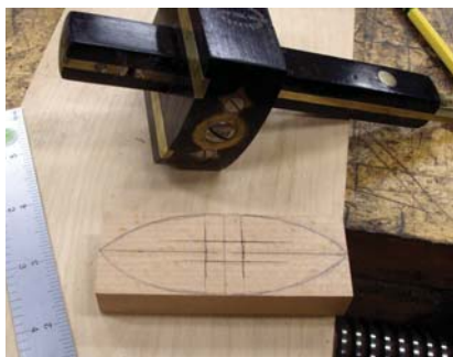
Whorl. To lay out and cut the mortise on the whorl, start with square stock and draw centerlines on both faces, then use a gauge to define the mortise on both faces, and chop in from both sides with your chisel.
