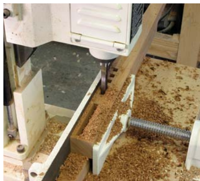
Added strength. The solid area between the two mortises is 1" long. In a rail this wide, split tenons should be used for strength and rigidity.
