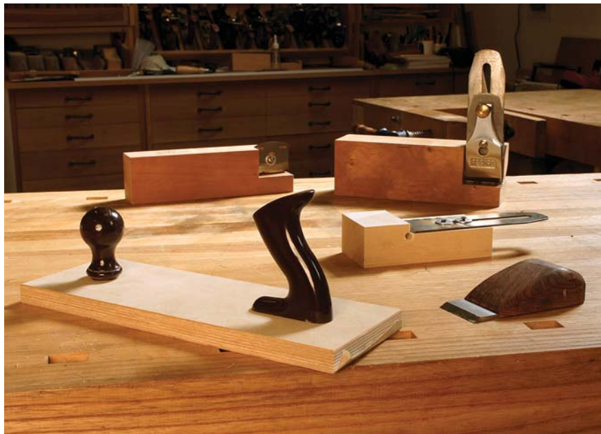
New tools from old. Don't let those old planes just sit and gather dust – the parts can be used to make some clever new tools (clockwise from left): a sanding block, a simple string inlay thicknessener, an adjustable string inlay thicknessener, a dowel-making jig and a chisel plane.
