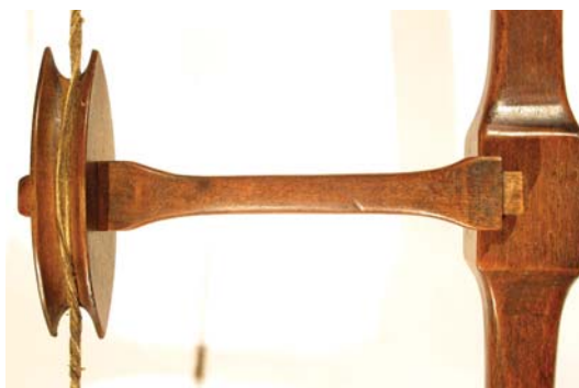
Add tension. This picture shows the detail of the windlass, which is used to apply tension to the bowsaw blade.
