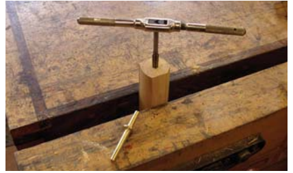
Ream. Before turning each handle to its final dimensions, use a hand reamer to ream the holes so that the brass pin is just shy of fully seating.
