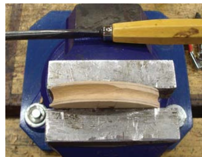
Groove. To cut the groove on the whorl that holds the string in place, use an 11-sweep 10 mm gouge to define the depth, then switch to an 8-sweep 11 mm gouge to shape the curve up the groove's sides.
