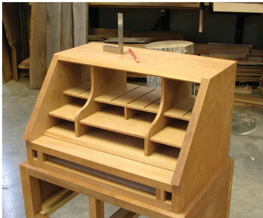
Again for accuracy. After the \frac{3}{16} "-wide letter dividers are routed in the upper shelves, transfer the layout to the underside of the top using a small square.
