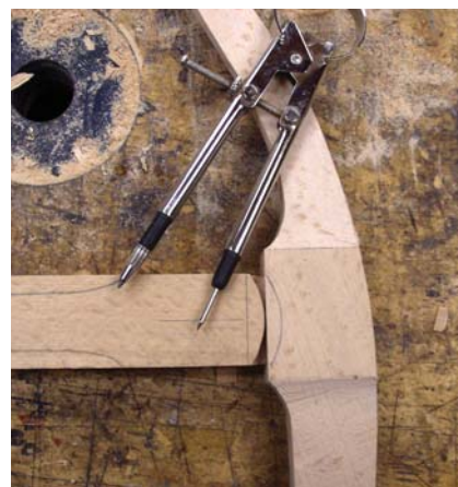
Play. The ends of the stretcher are rounded to allow a little play in the joint. You can lay out the curve from the template or set a pair of dividers or compass to scribe the curve.
