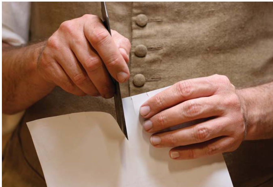
The paper test. During a day in the shop, I periodically perform two tests on my edge tools using scrap paper. When they fail a test, I know it's time to hone.
