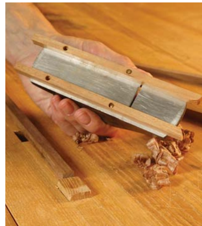
Perfect strips. Attach reference strips to a block plane to produce precise stock.
