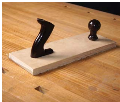
Sanding block. Attach the knob and tote to a piece of plywood and you have an instant sanding block (attach sticky-back sandpaper on the bottom of the plywood before use).
