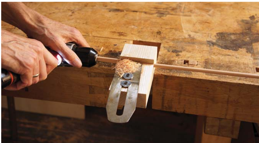
Custom dowels. With this jig, you can make your own dowels – and you can customize the jig to fit your dowel-diameter needs.
