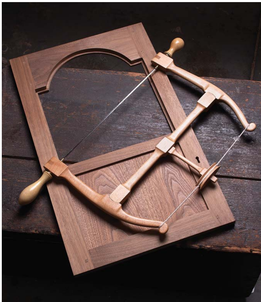
Curvaceous. This bowsaw, a reproduction of a mid-19th-century example with exuberantly curved arms, features traditional tapered pins – unlike modern commercial bowsaws.
