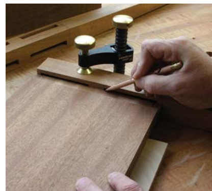
Not so tight. A small space between the tenon and mortise allows you to adjust the rail up or down to fit flush with the top of your legs.
