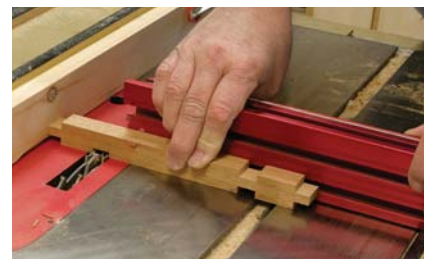
Save your fingers. A dado stack and a long workpiece quickly becomes two small, ready-to-use loper dividers, given a bit of creativity.
