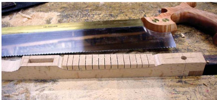
Shape the arms. You can cut the shape with a coping saw or bowsaw, or make a series of crosscuts and chop the waste with a chisel.
