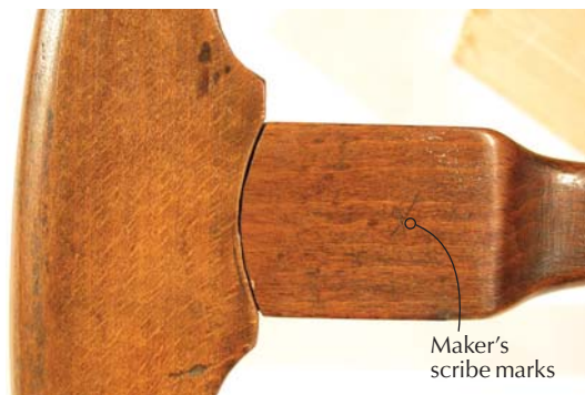
Period marks. Note the crossed scribe marks on the stretcher made by the original maker and used to lay out the arc of the tenon shoulder.
