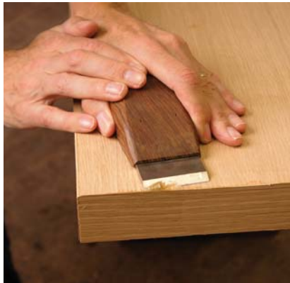
Chisel plane. Rare earth magnets hold the blade tight to the handle in this chisel plane.
