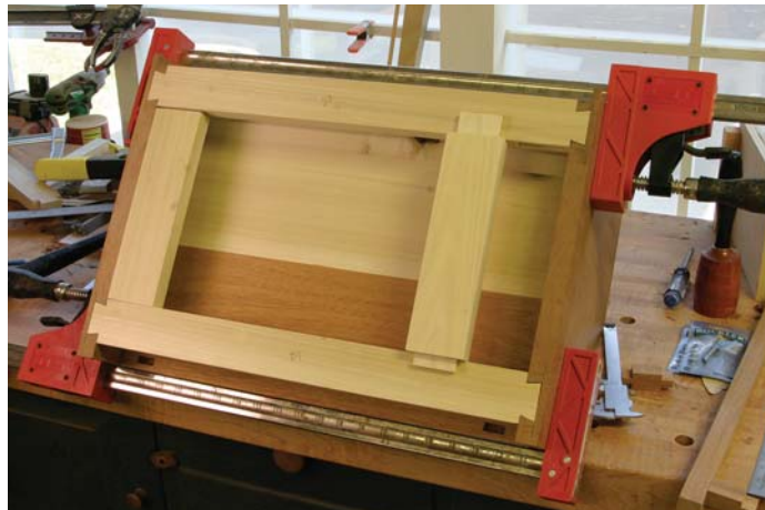
Both fixed & movable. The frame rails fit into \frac{1}{2} "-deep mortises at the front (they are glued for strength) and into 1" mortises at the rear. The back mortises are free to float to accommodate seasonal movement.
