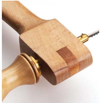
Spline. While the tool I was copying didn't have this spline, I added it to reinforce the tapered hole for the handle.
