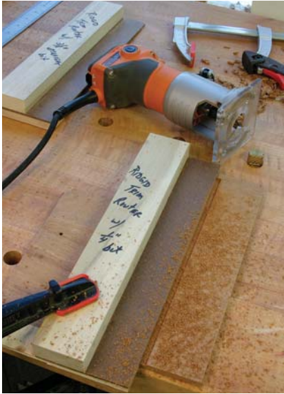
Shop workhorse. Router jigs are used to make dados throughout the inside of this desk. They are so simple to make that you should have one for each different router bit diameter.
