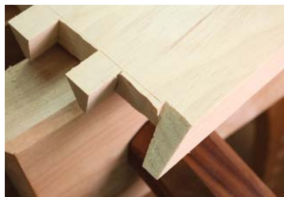
The pin board result. This board looks a little more straightforward than the tail board. It's basically a standard-looking pin board with a miter cut on its front edge.
