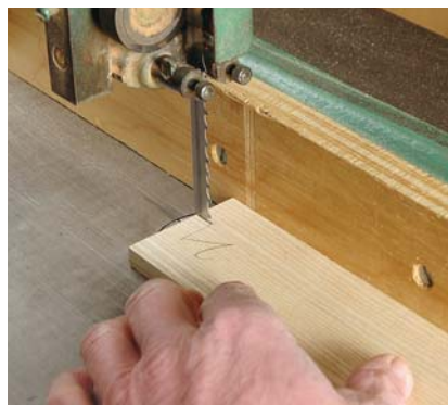
Notch test. With stock at the ready sized in width the same as your actual pieces, set your band saw fence to make the first cut for the center notch, then flip the board and cut the second side of the notch. Make sure your shims fit the slots tightly and check that your chisel will fit just inside the waste.
