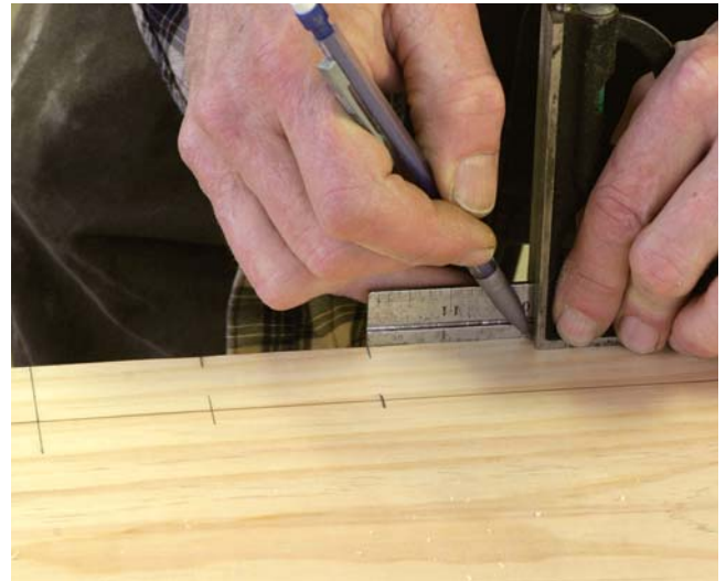
Fast & precise. Make a series of accurately spaced marks by lining up the end of the blade with the last mark made.
