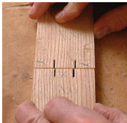
End-to-end match. If your cuts are set up and shimmed correctly, the inside edges of your kerfs should align.
