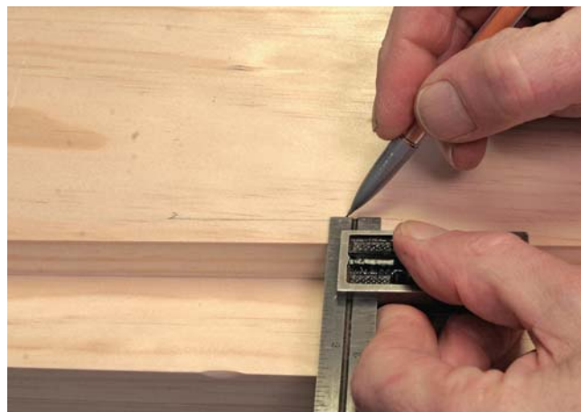
Pencil's partner. Make a parallel line a precise distance from an existing edge by sliding the head along the work and holding a pencil to the end of the rule.
