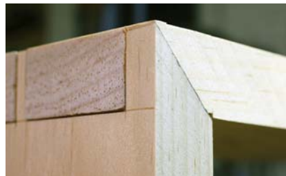
Needs a fit. You can see how the tail isn't fully seated in its socket. The way to fix that is to saw through the miter.
