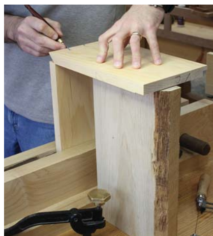
Tails, meet pins. I have my tail board resting on a scrap to keep it in position as I press its shallow rabbet against the pin board. Knife in the joint. Use light strokes at first, followed by heavier ones.
