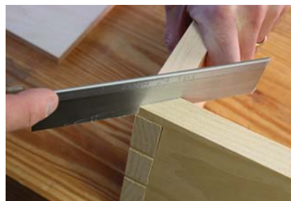
Saw right through. Use a thin-kerf saw and cut right through the miter. The joint might pinch the blade a bit. That's OK. It means the process is working.
