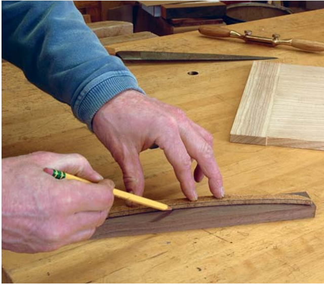
Template. Mark out the handle shape onto your blank. A template made of MDF or masonite allows for quick transfer of the shape.
