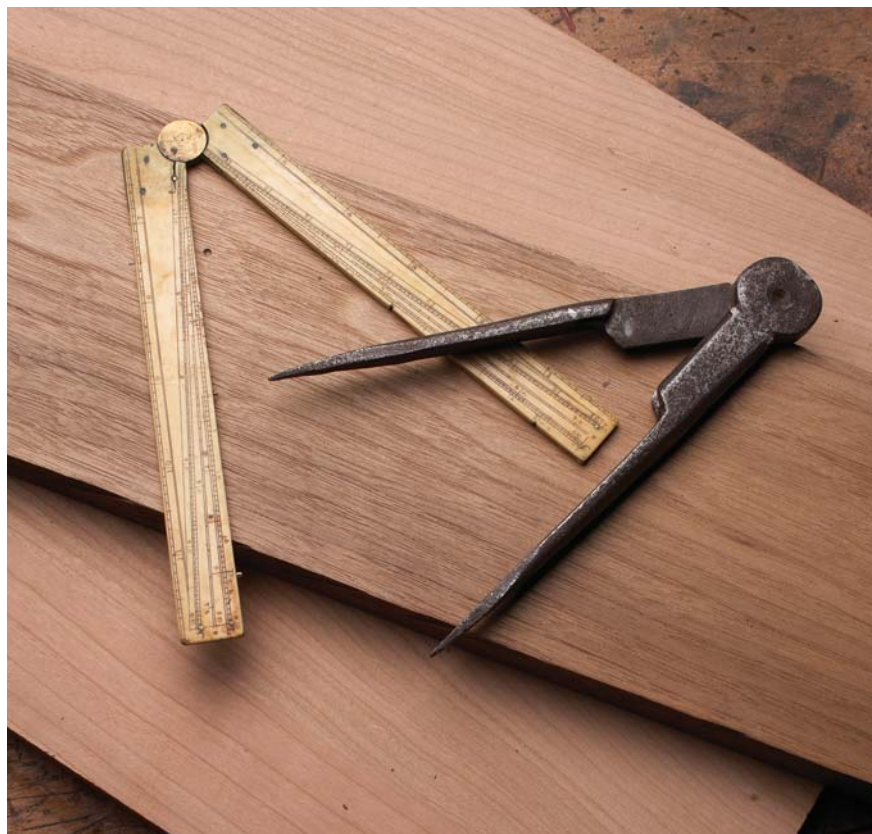
The traditional tools. Here's an ivory sector and traditional dividers. While original sectors are rare, you can make your own with scraps in an afternoon.
