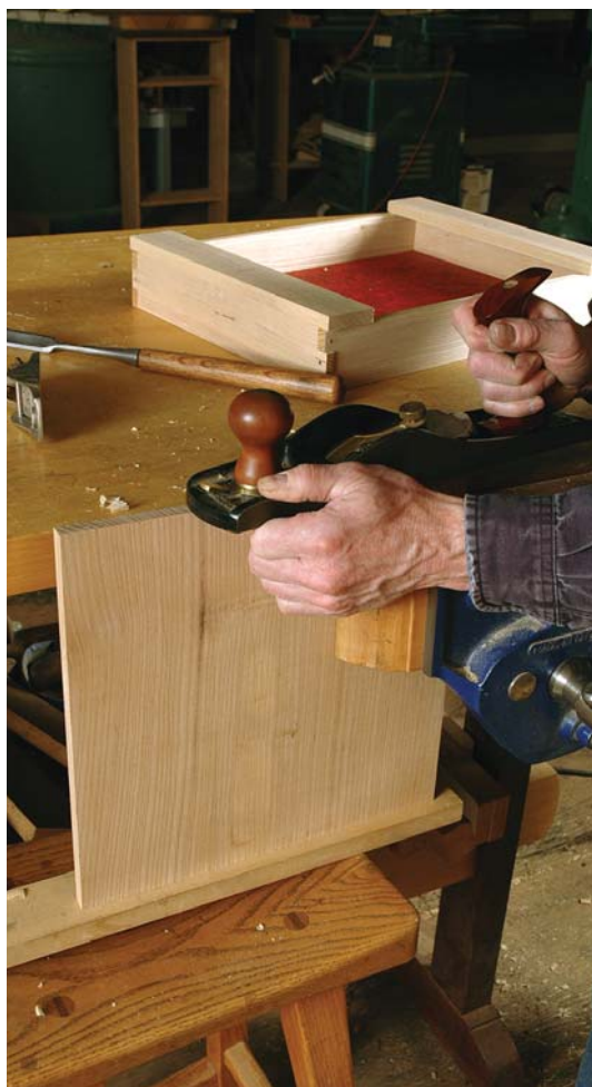
Dead flat. Before you start the joinery for the breadboard ends, plane the top's end grain so the end is dead straight.
