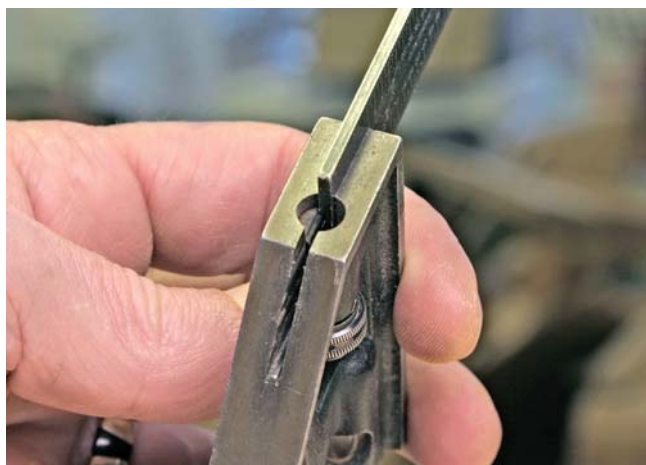
Remove & reverse. The groove in the rule slides in a tongue at the end of the spring-loaded reversible lock bolt. If you remove the rule, you need to line them up.
