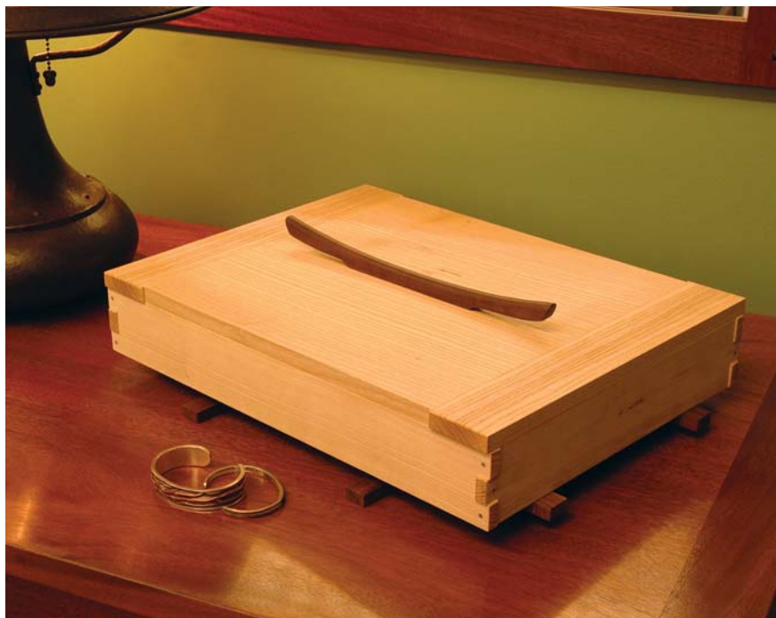
Ashtastic. This ash, finger-jointed jewelry box is simple to build with just a few tools: A band saw, chisel, handplane and router are all that's required.
