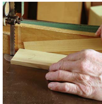
Fit test. To cut the matching part of the joint, slip the end of the shim between the fence and your stock, and make the cut with the shimmed stock held tight to the fence, then flip the board and make the second cut.
