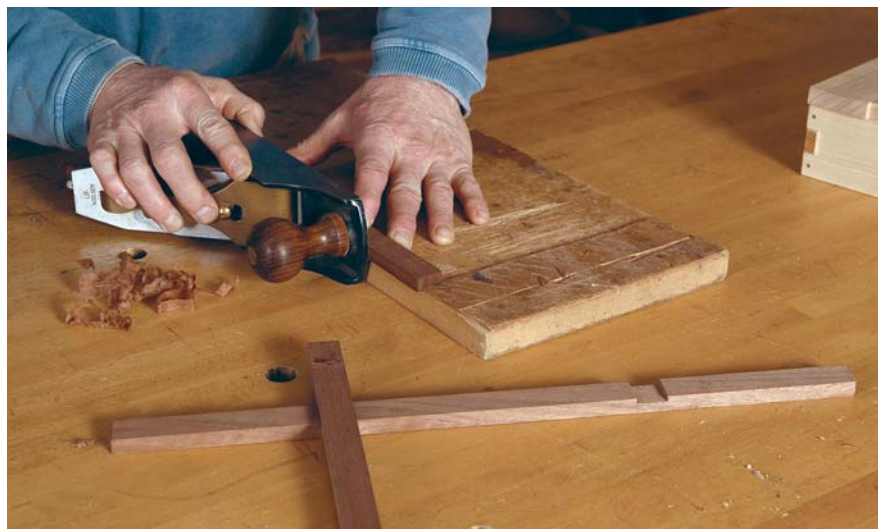
Plane to fit. Fit the base boards together using a bench plane with a bench hook or shooting board. Plane the long-grain edges of the short boards until they just fit into their notches.
