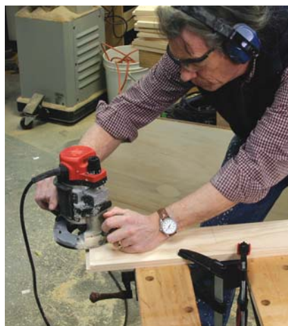
Router rules. Clamp the work securely before routing the rabbets and keep the base firmly on the surface.
