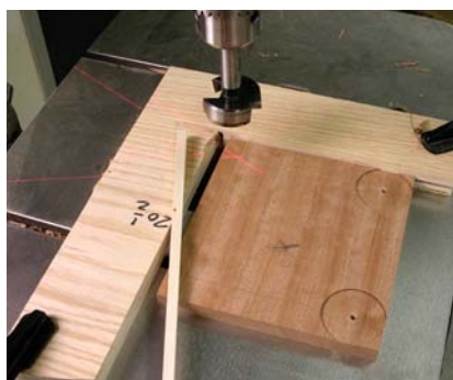
Proper spacing. A spacer, to compensate for the \frac{1}{4} " added when the box top is attached, moves the box parts into the proper position.
