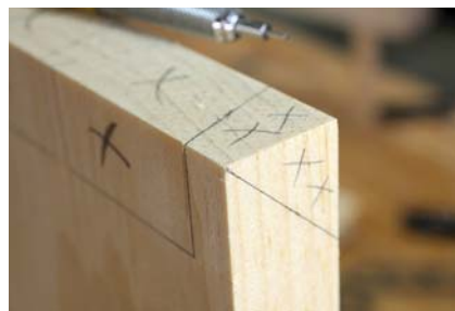
More wacky miters. Here's the completed pin board layout, with the waste marked with "X"s. Clear out the waste between the pins, then cut the miter.
