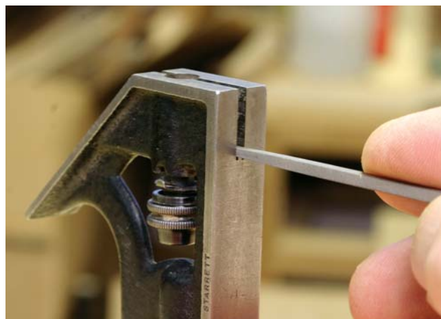
There is a solution. The rule rides on two nubs inside the head. If it isn't square, filing one nub or the other will bring it back.
