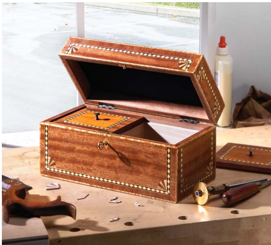
Inlay outside the box. Think differently about inlay as you slice and fit fans – assembled from wedges – into recesses created at your drill press.
