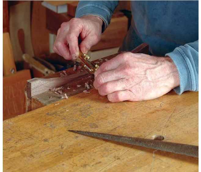
Cleanup. Clean up the first band saw cut on the handle with a spokeshave or rasp. Work downhill into the hollow to avoid tear-out.
