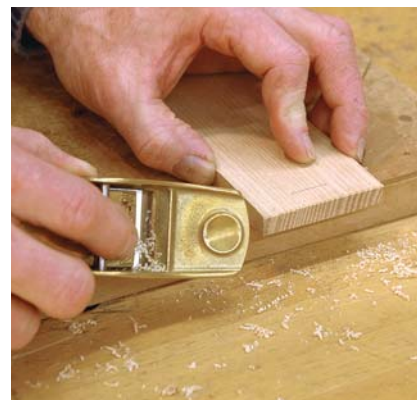
Ease the edges. Use a block plane to chamfer the ends of your stock now, before you make any cuts.
