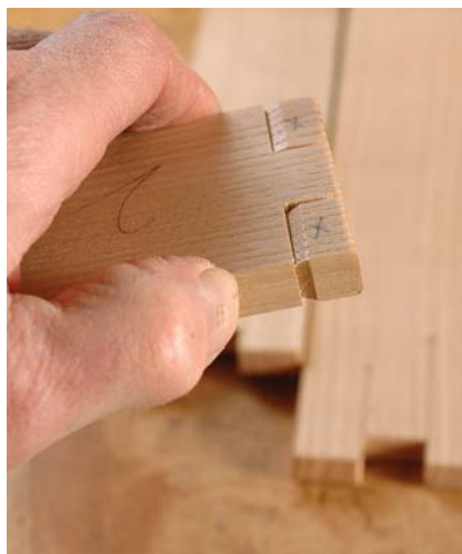
Establish the cut. Use your chisel to establish your cuts and help guide the band saw blade.
