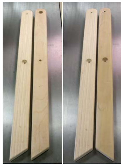
Identical legs. The only difference between the legs is where the holes are drilled (left). You will need two sets of mirror-image legs (right) per table.
