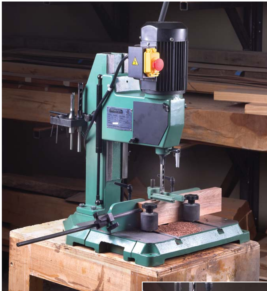
Lots of cast iron. General's mortiser base provides much of the machine's weight. Its extensions provide 35" of overall side-to-side support.
