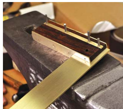
18 Only slightly proud. The rivets should be only .0625" longer than the handle thickness. Insert rivets into the holes as shown.
