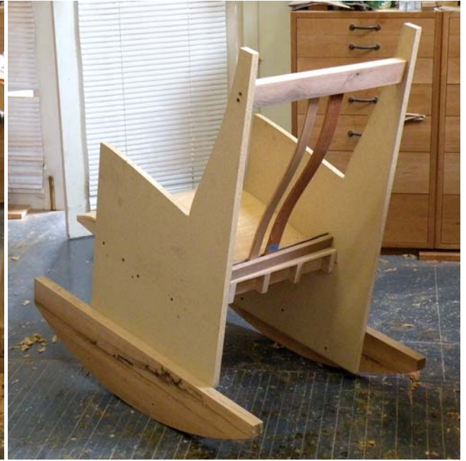
Mock you to sleep. This mock-up of my rocker design allowed me to quickly change variables and immediately feel the outcome.
