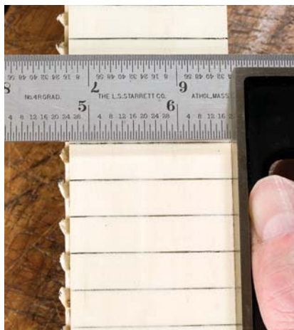
Keep it square. The peaks of the ebony, must be square to the edge before the second set of V-grooves are made.
