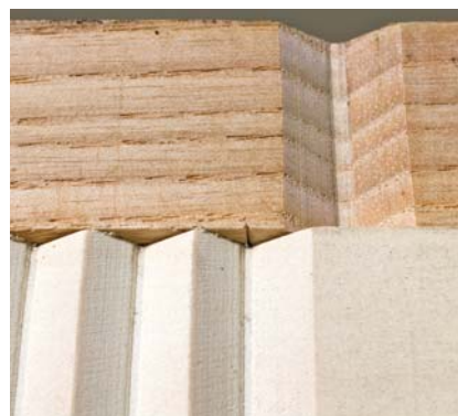
Indexing. Spacing the V-grooves is critical and the index mark makes for foolproof accuracy.
