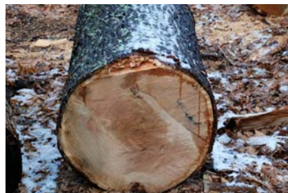
Search for perfection. A dead-straight and perfectly round log, free of branches, will give you the best results when riving.
