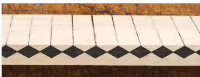
Make a sandwich. Holly and black dyed veneers enclose the diamond banding, giving it extra strength and visual interest.
