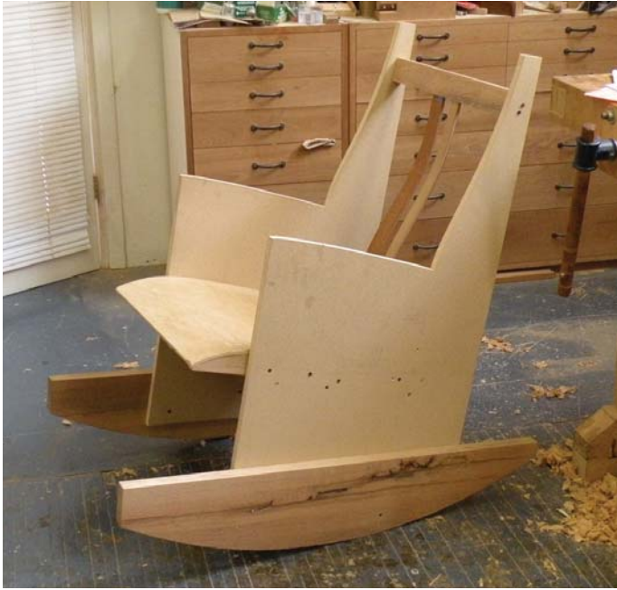
Mock you to sleep. This mock-up of my rocker design allowed me to quickly change variables and immediately feel the outcome.
