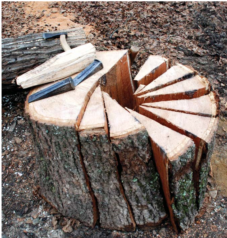
Start with a log. For my style of woodworking, “green” is best. So, I always split my own oak planks from a freshly felled log.
