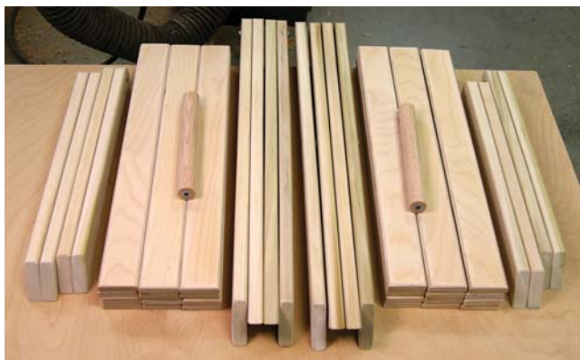
Round the legs and arms. Use a disc sander to round the pivot points on the legs and arms.
