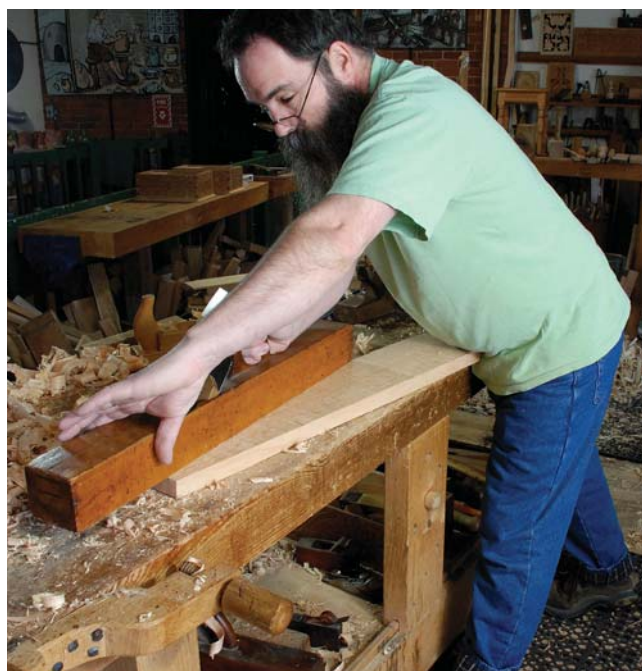
Fore plane. The convex iron in this fore plane (you may know it as a “scrub” plane) takes big bites to quickly remove stock from a rough board.
