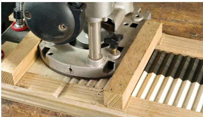
Flat out. The V-gouge removes the flat left by the router bit. Note the difference in the groove bottom, to the right of the gouge.
