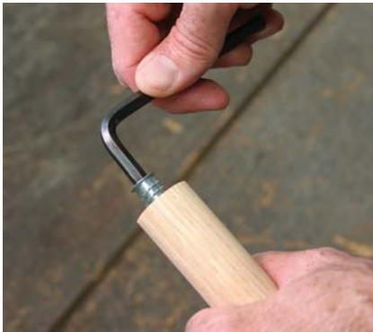
Threaded insert. Use an Allen wrench to drive the insert into the oak handle.
