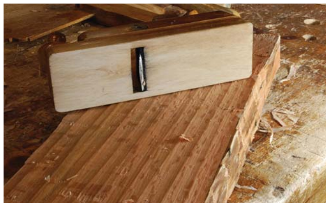
Fore plane. The convex iron in this fore plane (you may know it as a “scrub” plane) takes big bites to quickly remove stock from a rough board.
