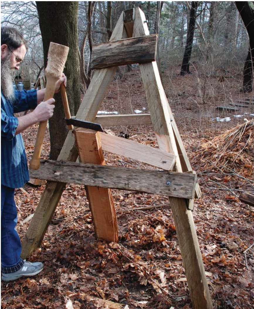
Riving brake. This shop-made appliance allows me to exert more or less pressure to direct the path of the split – to a point.
