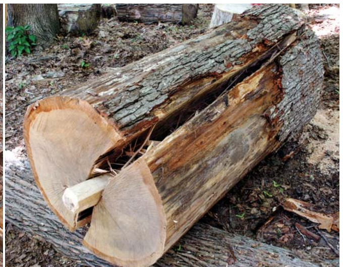
Split. After starting the split with steel wedges at the outer edges of the log, drive a wooden wedge at the center. With the end wedge holding open the split, drive steel wedges along the side.
