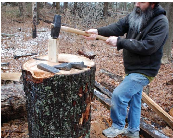
Split. After starting the split with steel wedges at the outer edges of the log, drive a wooden wedge at the center. With the end wedge holding open the split, drive steel wedges along the side.
