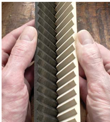
Closing the book. Sawn apart and folded together, the banding starts to take shape.
