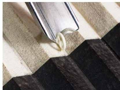
Flat out. The V-gouge removes the flat left by the router bit. Note the difference in the groove bottom, to the right of the gouge.
