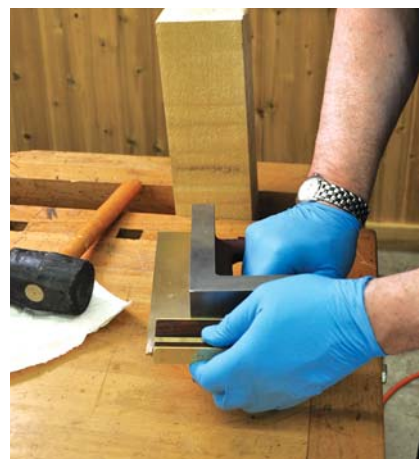
16 Victory. The square is now light-tight to the reference.
