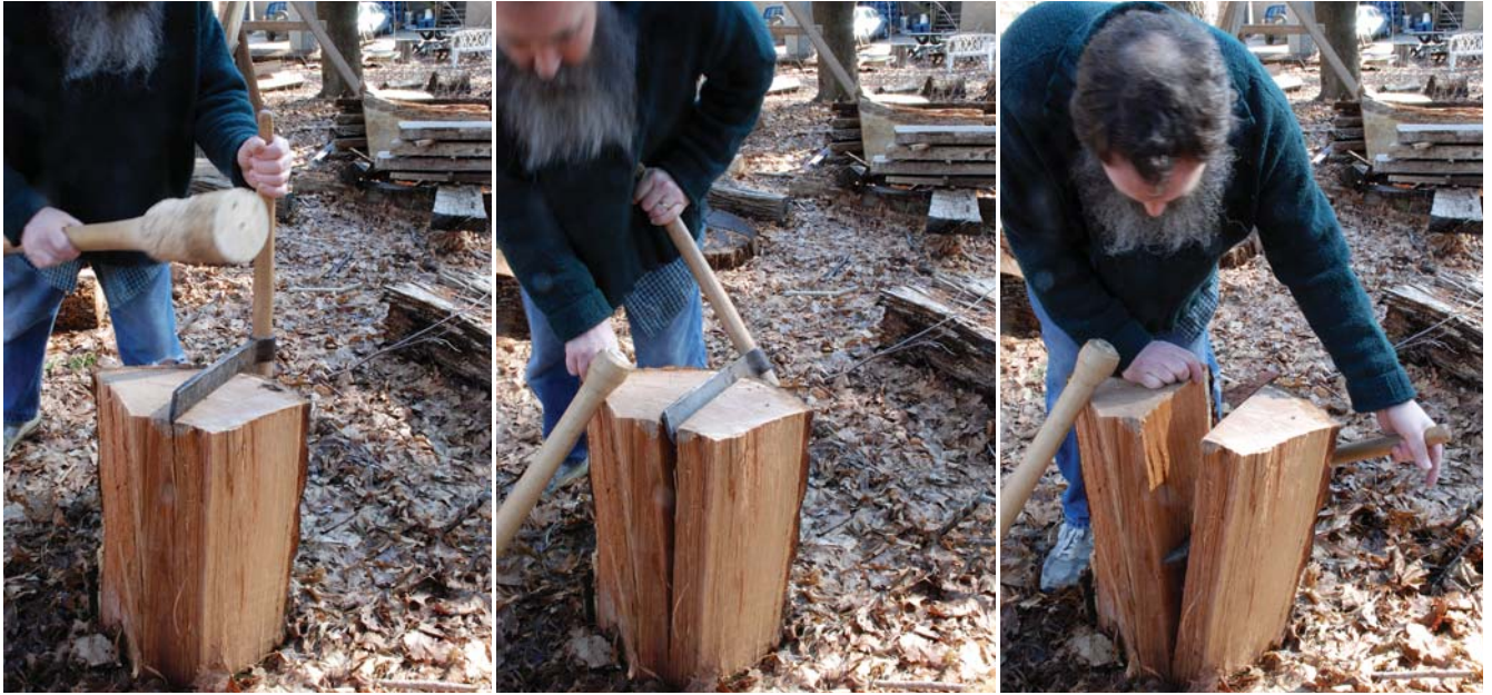
Riving. To rive a section of a log instead of split it, use a mallet and froe. Start the work by knocking the blade of the froe into the top of the billet, then push (or pull) the blade parallel to the ground, and continue working down the split in that manner until the two pieces separate.
