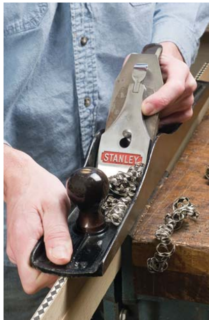
Gluing surface. Before sawing, each strip of banding is planed to provide the best glue surface for inlaying. Note that the components fit so precisely that the shavings hold together.
