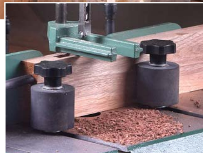
Adjustable rollers. Bumpers push material tight to the fence yet allow pieces to slide.
