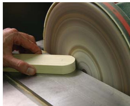
Round the legs and arms. Use a disc sander to round the pivot points on the legs and arms.
