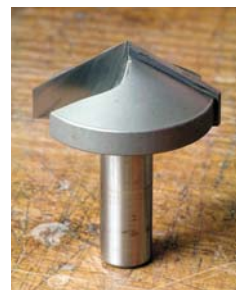
Choices. The 120° V-bit shown here is only one choice; other angles also make interesting bandings.
