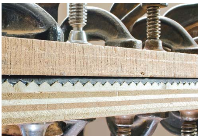
Keep it square. The peaks of the ebony, must be square to the edge before the second set of V-grooves are made.
