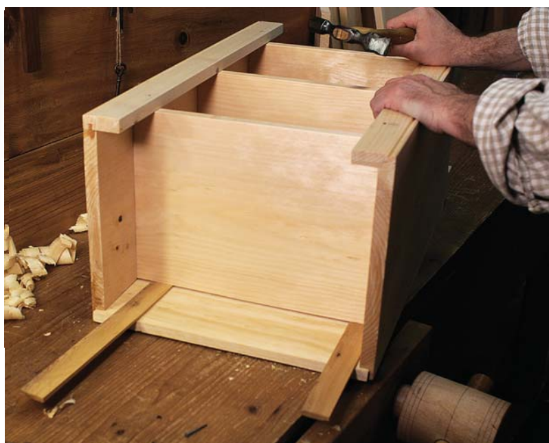
Tighten up. Shims force the shelves tight against the face pieces for nailing.
