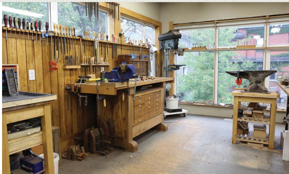
For metalwork. This small bench is where most of the metalworking occurs. Sauer files dovetails for the shells of his planes and bends the curved sidewalls on the anvil behind.
