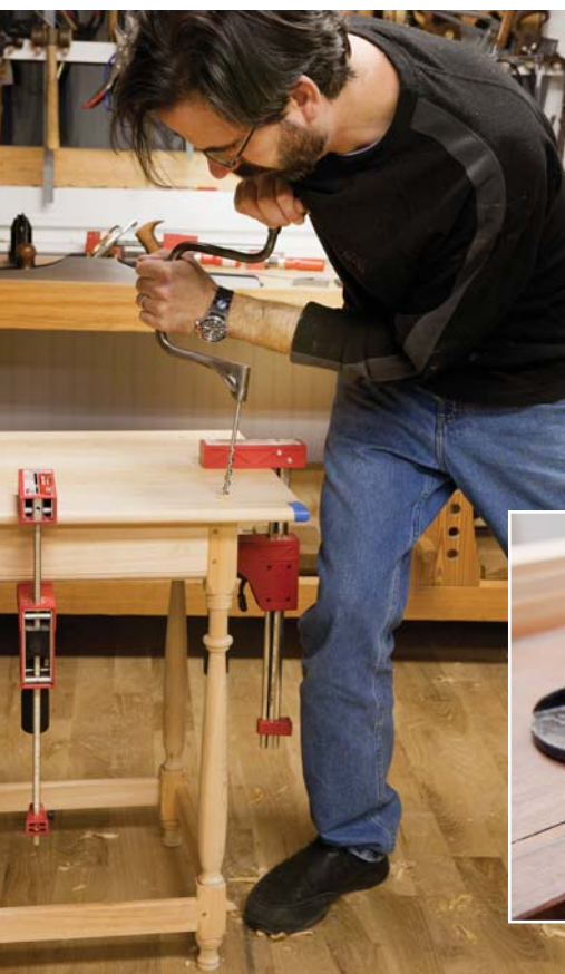
Finish the holes. Clamp the top to the base and finish the holes. The final depth is about 3".
