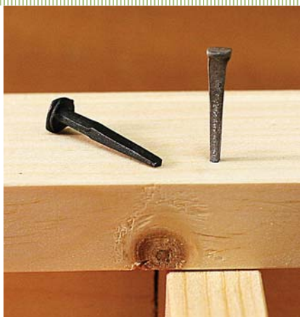
Align right. Period nails are rectangular in cross section and tapered. They must be aligned carefully so that the taper crushes end grain fibers. If you align the taper across the grain, you risk splitting the wood.
