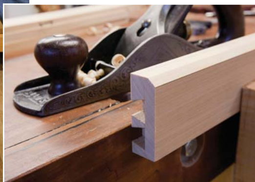
Chamfer then round. As on the rest of the table, make a chamfer on the bottom corner of the drawer front, then finish the job with a No. 8 or No. 10 hollow plane.
