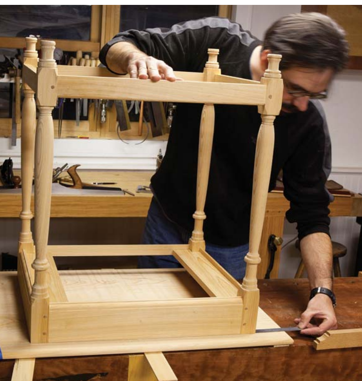
First trace. With the whole table upside down, and the base centered on the top, trace out its shape – both the outside of the base and the inside.
