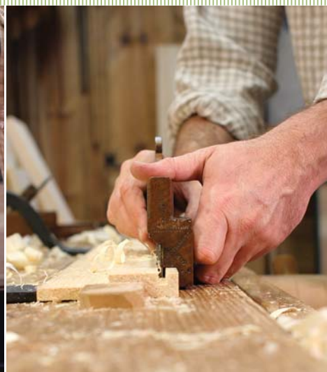
Tongue-and-groove. “Match” planes cut perfectly matching tongue-and-groove joints. Though they may have been designed to produce wide panels, you can apply the groove to a face instead of an edge to make a right-angle joint. This is of great use to the boarded furniture maker.
