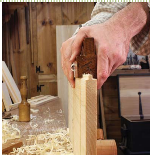
Tongue-and-groove. “Match” planes cut perfectly matching tongue-and-groove joints. Though they may have been designed to produce wide panels, you can apply the groove to a face instead of an edge to make a right-angle joint. This is of great use to the boarded furniture maker.
