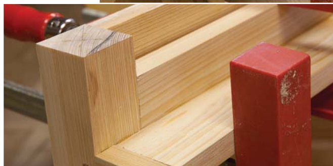
Guide from the side. Glue the drawer guides to the runners and take care to make sure that they, too, are flush to the inside surfaces of the legs. A little attention here saves a lot of headaches later.
