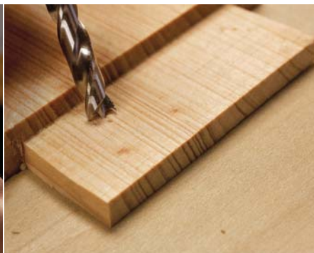
Shift the hole. Then bore the hole about 3/32" closer to the shoulder. This offset will pull the joint together when the peg is driven through the two holes of the joint.
