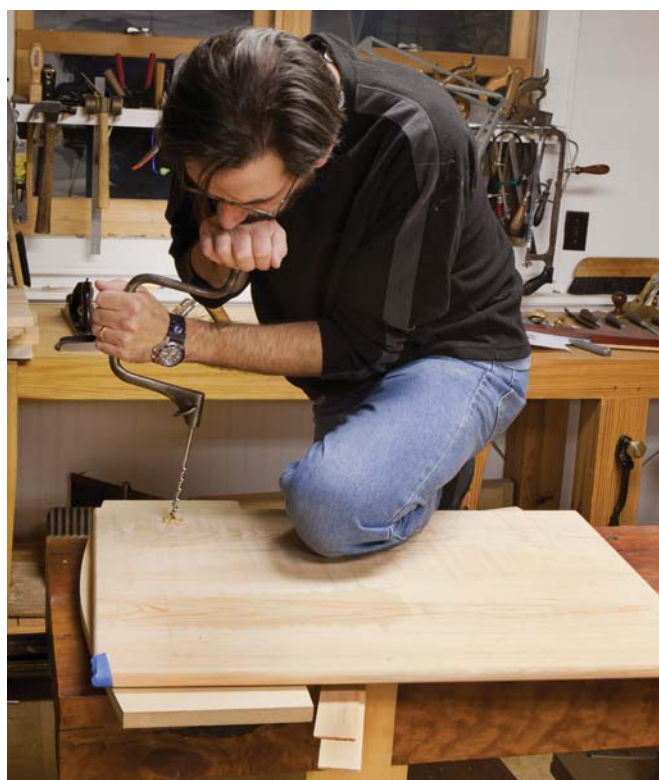
Bore from below. Now bore the holes through the top. Note that the bit is angled. The exact angle isn't important – just add a little lean to it.
