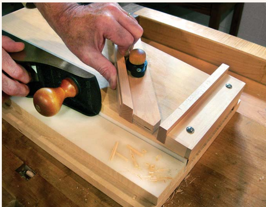
Simple work; great details. Small parts such as bead mouldings are a cinch to trim to perfection with a shooting board and sharp plane.
