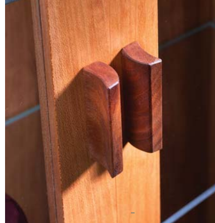
A comfortable pull. A departure from Krenov's original, the gently curved walnut pulls emphasize the vertical lines of the doors.
