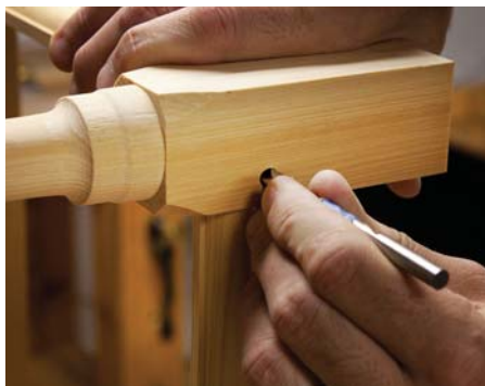
Marking the bore. With the table dry-fit, use a 1/4" brad-point bit to mark the centerpoint of the hole on the tenon cheek.
