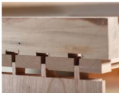
Custom caul. To make sure the dovetail joints seat completely, make a clamping caul that applies pressure on only the tails.
