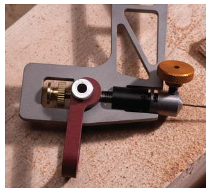
Cam action. The blade is tensioned by setting the brass screw appropriately, then flipping the cam lever. Once the screw is set, it's quick and easy to flip from tensioned to not.
