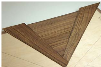
3. Pattern matching. After each glue-up, match the workpiece to the pattern on the substrate to determine where to plane the next pieces to fit.
