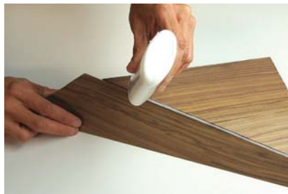
1. Glue. After taping the seam on one side, fold the pieces open just enough to run a thin bead of glue down the edge.
