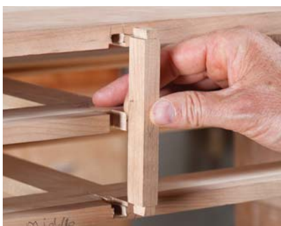
Upper drawers divided. A vertical partition divides the case for the four narrower upper drawers. It is dovetailed like the divider fronts at the ends, and it is let into the middle of the top drawer divider with a simple notch.
