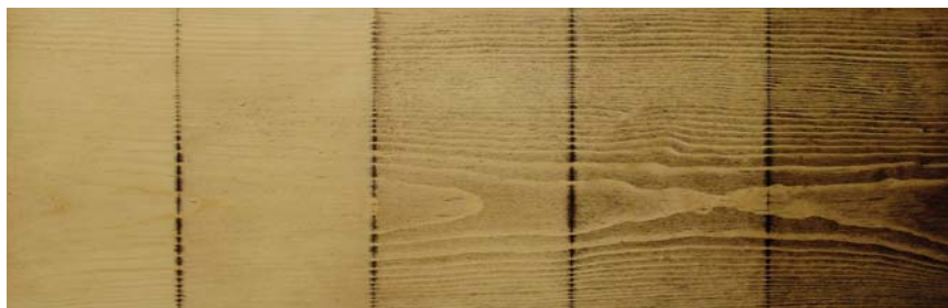
Washcoating. This blotchy pine board shows the impact of thinning a washcoat to various degrees before applying a stain. Left to right are sprayed full-strength lacquer, lacquer thinned 1-to-1 with lacquer thinner, 1-to-2, 1-to-3 and finally 1-to-4. It's clear that getting the mix optimized for maximum color and minimum blotching is no easy matter.
