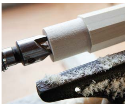
Tenon the legs. Turn a 1\frac{1}{2} " long by 1\frac{3}{8} "-diameter tenon on the top of each leg after you've finished planing the octagons.
