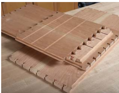
Ready, set, assemble. When all the case joinery, including dovetails, dados and rabbets, is completed, the toolbox is ready for glue-up.
