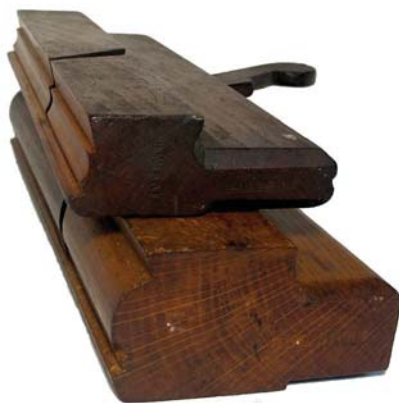
One-trick ponies. Moulding planes with complex profiles are limited to cutting only the one profile for which they're designed.
