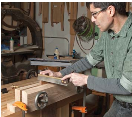
The right working height. A Moxon-style vise (this one is from Bench-crafted) can hold boards for dovetailing (and other work) at the perfect height.
