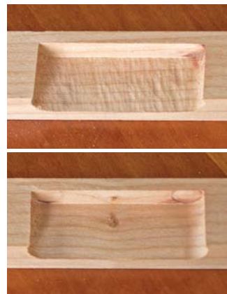
Too fast? If you cut too aggressively with a router, the results suffer. In the mortises above (which are sliced in half lengthwise), you can see chatter on the top. On the bottom is a mortise routed at an appropriate speed.
