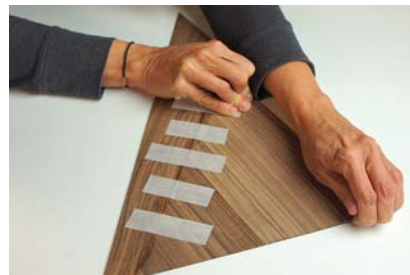
2. Tape. After the glue is applied, apply pieces of tape across the seam and move on to the next edge joint while this one dries.
