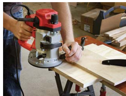
Rabbets & fences. Set up a fence to keep the router perfectly straight.
