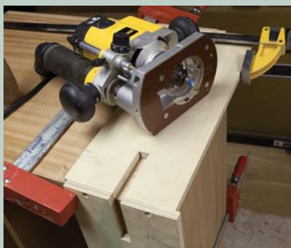
In two dimensions. For the L-brackets, an L-shaped template is clamped to the carcass to guide the router.
