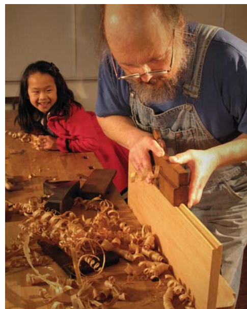
Or use dedicated planes. Matched sets of table joint planes cut perfectly matched profiles – simply work to a scribed line.
