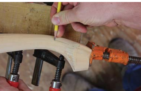
Finger guide. Use your finger to extend the toe line up through the ankle of the leg.
