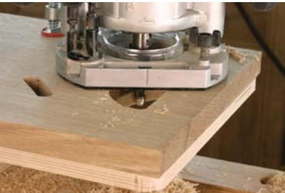
Saw first, then trim. Cut close to the lines with a jigsaw and use the router to trim the opening at the top.
