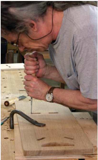
On top. Positioning your shoulder over the chisel allows you to use your body weight to pare the end of the mortise.
