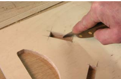
Score first. Prevent tear-out by scoring around the openings before cutting with the router.
