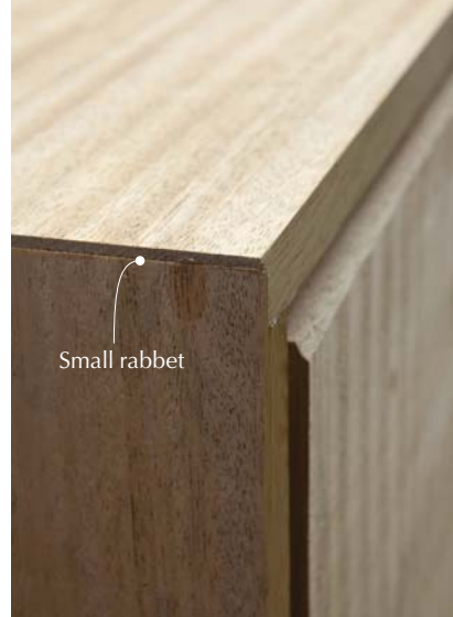
Full blinds. Here are the dovetails for the secretary's top. Note the small rabbet at the end. When the joint is assembled the rabbet is the only part of the joint that shows.
