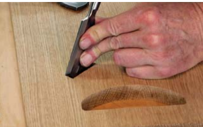
Swing it. Press the back of the chisel against the mortise wall, then rotate the edge down to the corner to maintain a straight edge.
