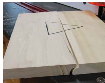
A perfect fit. When set up correctly, a matched set of table-joint bits guarantees profiles that will mate and work smoothly.
