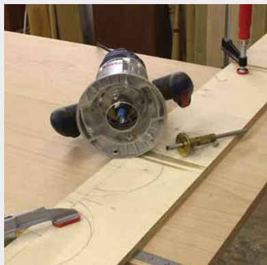
It's all in the setup. A plywood straightedge guides my router in the first step to forming a tenon for the breadboard ends on the countertop. A 1½"-long tenon is the result.
