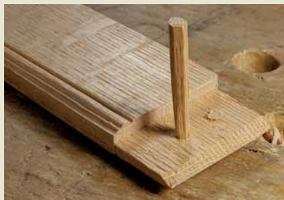
Second chance. This is how you get a second chance on the mis-bored tenon. One pin has been trimmed with a saw; the other is as it was driven. Once they are both trimmed, use a chisel to pare them flush. Then test-fit the joint, mark it and re-bore it.
