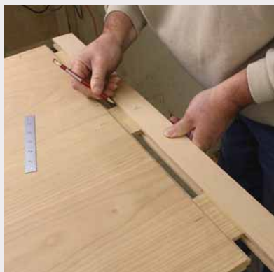
Mark for movement. As you transfer tenon locations to the ends, add a little wiggle room (⅛" or less on either side). There is no need for tenons to fit tight side to side.
