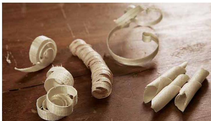
As thick as possible. As you gain confidence and strength, you'll be able to rip off enormous curls with your tools. Until then, try thinner shavings or softer wood.
