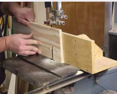
Band saw justified. Tapered drawer sides and backs are quick work at a properly set up and tuned band saw. Tilt the table and use a fence for accurate cuts.
