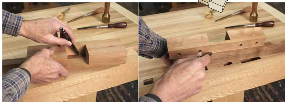
Mortise layout. Hold the positioning strip against your reference edge and scribe the far side and two ends of your mortise. Then flip the jig around and scribe the near side.
