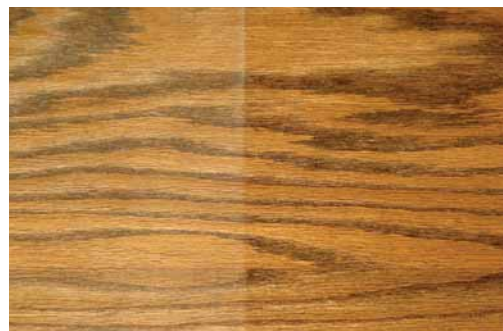
Two coats necessary. To develop the full sheen of a finish, a minimum of two coats are necessary, with the first sanded after it has dried. The contrast between one coat (left) and two coats (right) shows the difference.
