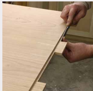
Small & mighty. The long tenons of your breadboard end hold pieces to the top, but it's the ¼" tenon that runs the width of the top that keeps things flat and level.
