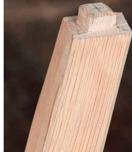
Tenons with a twist. At the top of the front legs, the tenons are set at an angle to match the arms.
