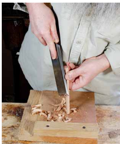
Posture counts. It's easy to think you just trim the pins, but there's more to it than that. Body posture makes a difference. The left hand is braced against the torso, helping to hold the stock steady. The right hand has the chisel tucked against the body as well. Very smooth and powerful movements guide the chisel.
