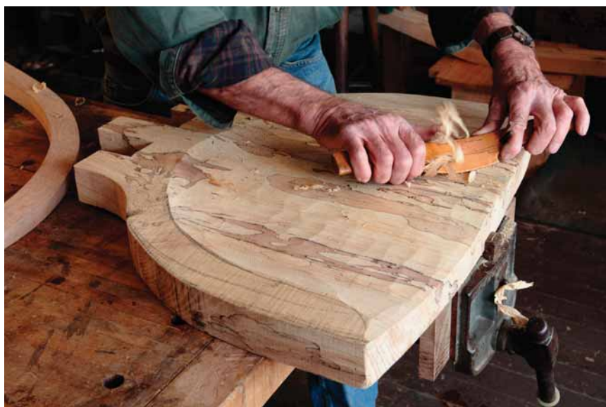
Smooth bottom. A travisher removes the adze marks and refines the shape of the seat.
