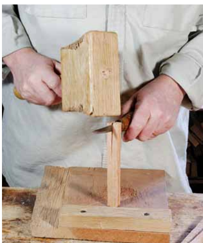
Follansbee rives. Riving principles apply here, just as on larger-scale stuff. Split in halves. Straight-grained stock is key. Never throw out any perfectly straight off-cuts, and keep a large supply on hand. The pins are the driest stock in the whole stool.
