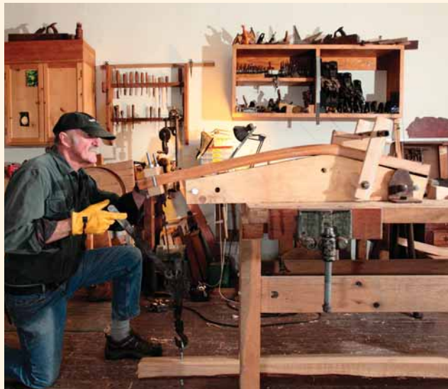
Hot potato. A come-along rigged to a 4x4 below the bench provides the power to bend the thick back just out of the steam box.
