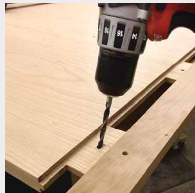
Plan to expand. Holes in the outer tenons are elongated to keep pegs from splitting the top during seasonal movement.
