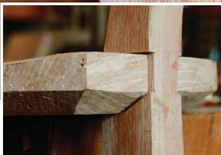
Match play. The notches in the front legs match the bevel angle on the bottom of the seat.
