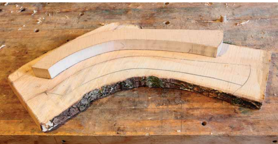
Natural fit. The arms are cut from a curved branch; avoid short grain where the arm bends.
