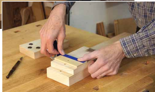
Drill with care. Position the parts to align the holes in all pieces. A leftover piece of spacer holds the work level.
