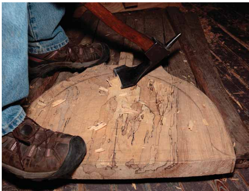
Quick work. An adze is used for the initial hollowing of the saddled seat.
