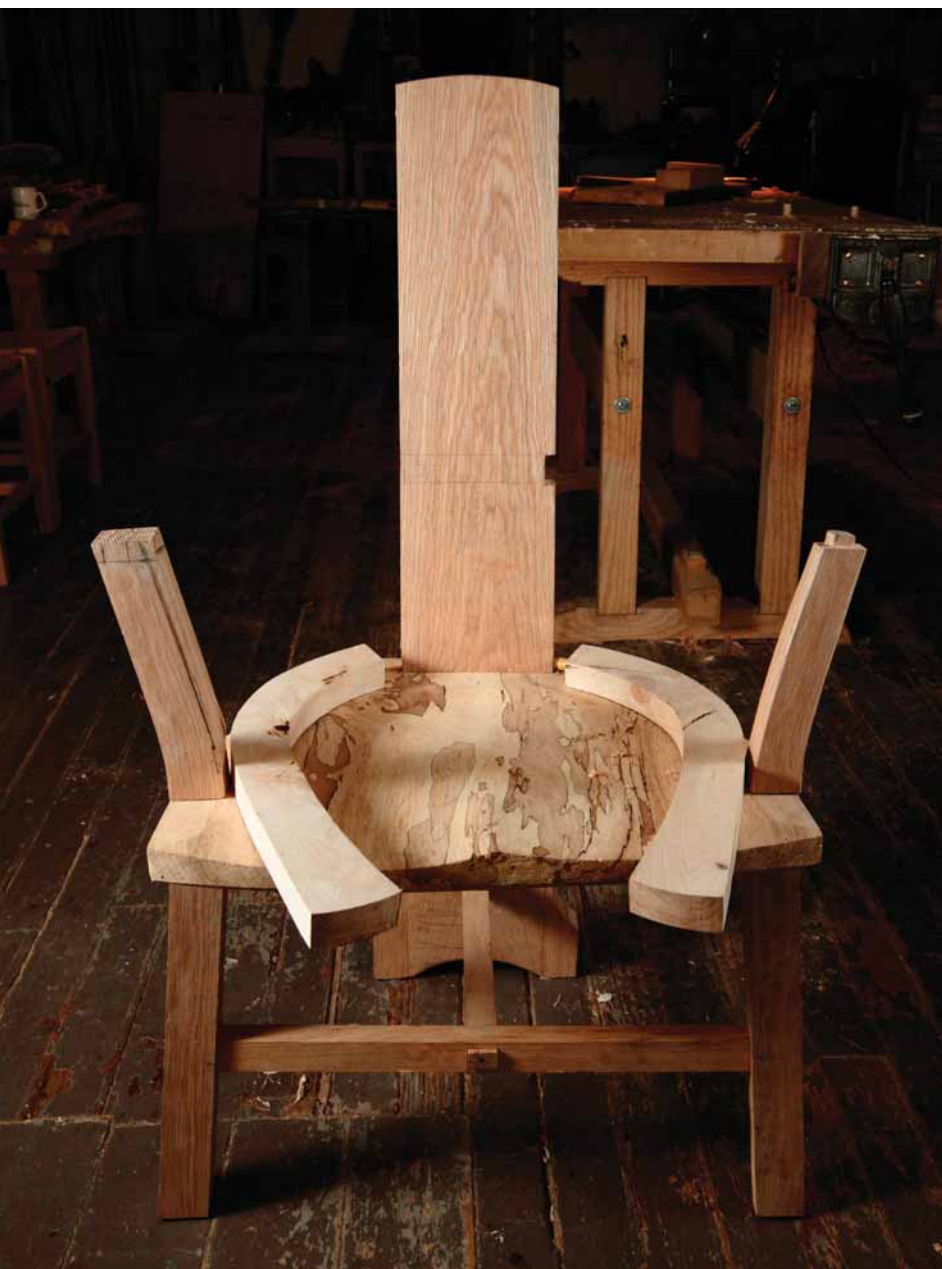
To a T. A single stretcher connects the front legs, and an additional stretcher joins the center to the back.
