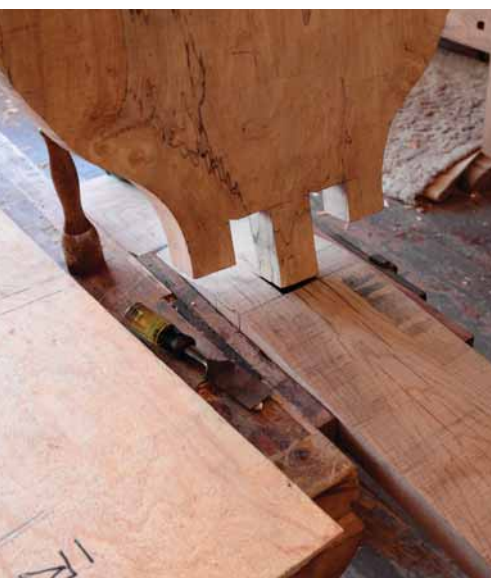
Strong back. A through-tenon connects the seat to the back of the chair. The back will be notched to capture the edges.
