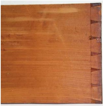
Hand-cut dovetails. Hand-cut dovetails indicate the furniture was made during the 19th century or before – as long as other clues don't point to a more recent time period.
