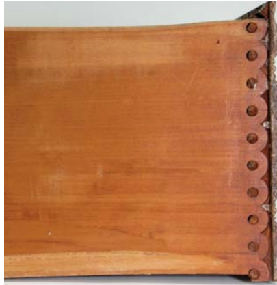
Pin-&-scallop joint. The pin-and-scallop joint was used from the early 1870s to the end of the 19th century. It's easy to date furniture containing this joint.
