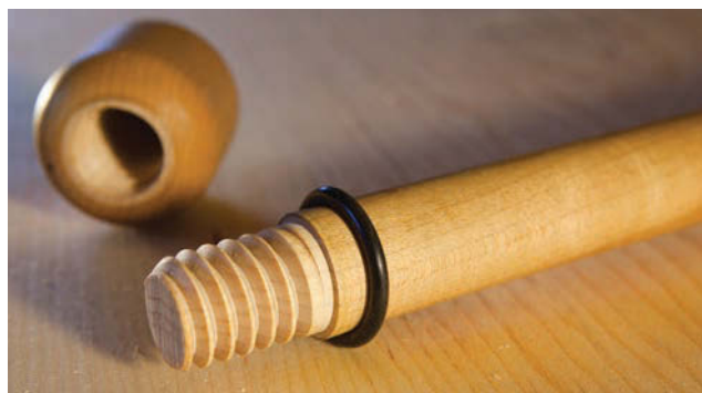
Lake Erie Toolworks tommy bar. Caps on tommy bars tend to come off – no matter how many screws or nails you drive through them. Lake Erie has fixed this problem with a screwed-on cap.
