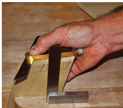
Tail end. Lines across the end grain are parallel to the top and bottom of the sides and ends. Placing the piece in the vise with the cutlines vertical will aid in sawing the tails.
