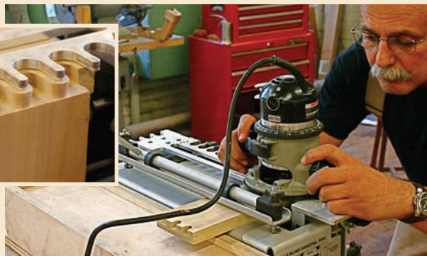
Simple dovetail jig. Easy to use, these jigs cut dovetails of a single size and rout both tails and pins at the same time.
