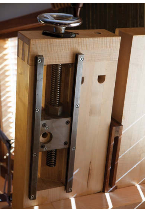
Benchcrafted Tail Vise. It doesn't look like much from the benchtop, but the engineering underneath this vise is impressive. I have this hardware on my bench and wouldn't trade it.
