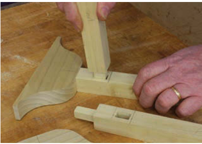
Not so square. To gain a bit more strength, tenons on the crossbar have smaller edge shoulders and larger cheeks.
