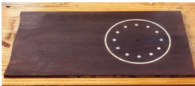
Inlay-safe. The solution has no effect on the mother-of-pearl inlay. Residue from coloring is removed with a non-woven abrasive pad, then the panel is ready for assembly.
