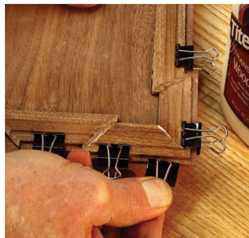
Happy ending. The outer corners are the last to be fit (and are the easiest to adjust) to complete the cornice moulding.
