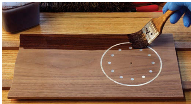
Nothing yet. The ebonizing solution won't change the color immediately. The chemical reaction between the rusty vinegar and the tannic acid in the wood takes a few minutes.
