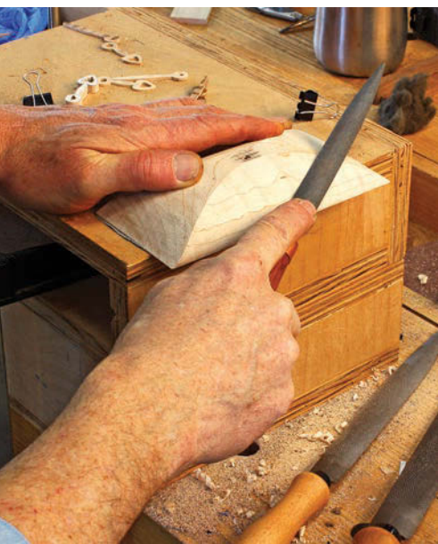
One, two, three. Rasps remove the band saw marks, refine the shape and smooth the surface of the dome.
