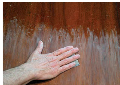
Sand to remove problems. Sanding removes surface crazing and other problems. Use the finest grit that will do the job efficiently. Here I’m using #600-grit sandpaper.
