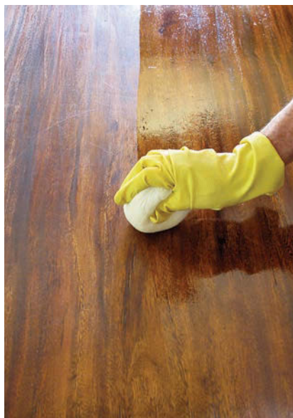
Thin finish. Applying a thin coat of finish avoids the fish-eye problems caused by silicone furniture polishes having been used. Padding wiping varnish, as I’m doing here, can be done on site.
