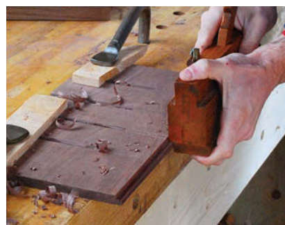
Rabbets. A moving fillister plane makes quick work of rabbets of many sizes, both with and across the grain, thanks to its retractable “nicker” and movable fence.
