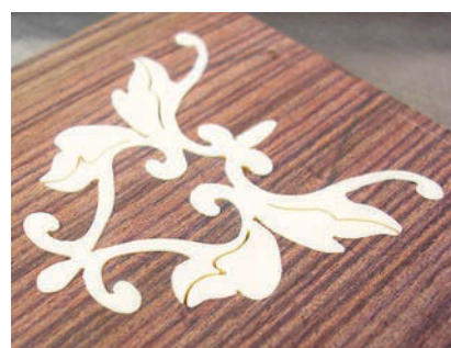
Flush. Now press the inlay firmly in place until it is flush.
