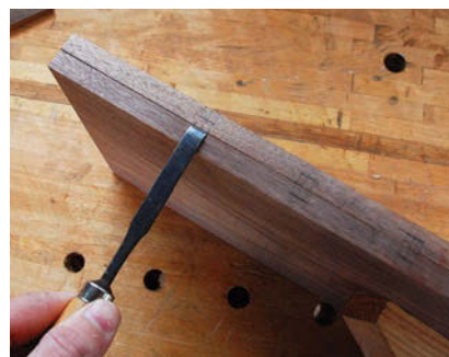
Size to fit. I use the same \frac{3}{8} " chisel I'll use to cut the dados to define the dado shoulders. That way, I know I have the perfect-sized tool for the job.
