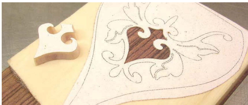
Tight fit. If you have the bevel on your saw table set correctly and make a good cut, the background piece will fit flawlessly.
