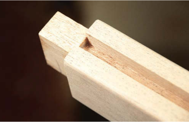
Protect the tenon. The groove in the rails is deeper than the tenon shoulder, so stop short with the router and square the end with a chisel.
