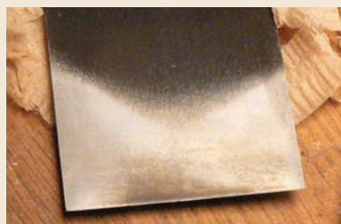
Flat back. The back is the most important surface to address when sharpening an edge tool. Notice the wear bevel at the cutting edge.
