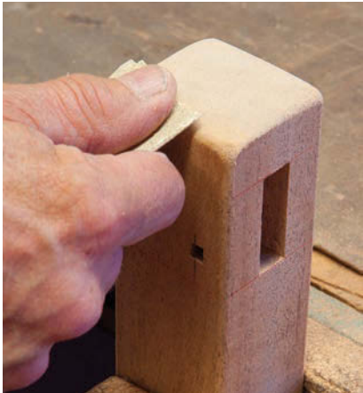
Soft touch. The tops of the legs and edges of the legs and rails are gently rounded.
