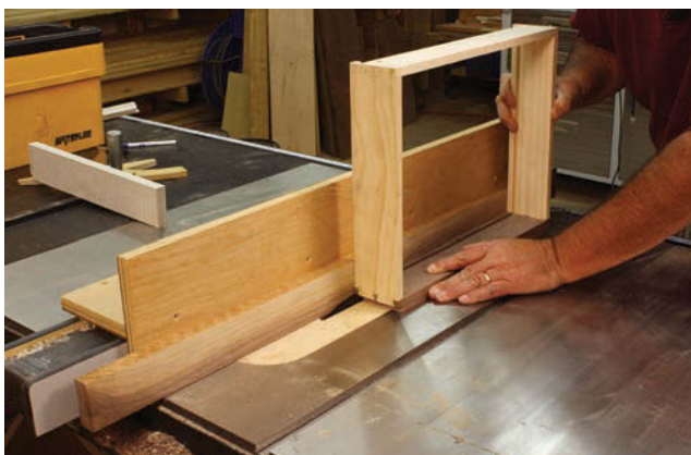
Hold tear-out at bay. Rabbets cut using a dado stack are less apt to tear-out, but you should still plow the two ends before the sides.
