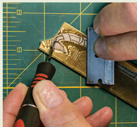
Use epoxy for metal inlays. Once the pattern is set in place, use a razor blade to squeeze out the epoxy underneath and keep the pattern flat.
