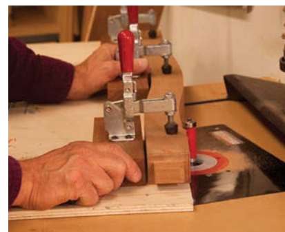
Ramp down. The extra width of the pattern provides room for placing clamps and keeps your hands a safe distance from the bit.
