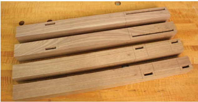
Flush fit. The 1/4"-wide x 1"-deep mortises are positioned so the rails fit flush to the outside face of your legs.
