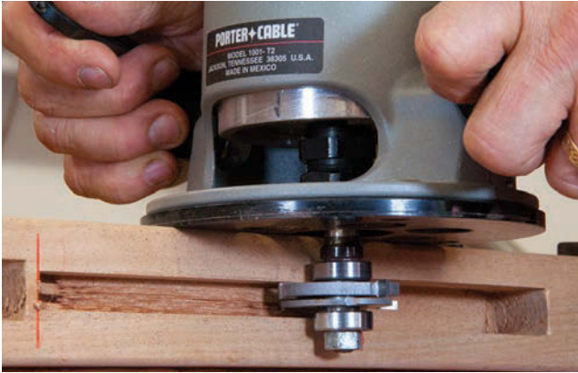
In between. The ends of the veneered plywood lower panel in the headboard fit in this slot between the mortises in the legs.
