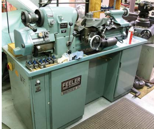
For turning parts. One of the more impressive machines on Chris' shop floor is his Feeler tool-room lathe (left) and the chucks he has collected for it (right).
