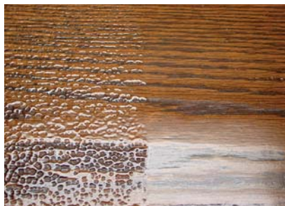
Shellac sealer. A sealer coat of shellac (right) will provide a barrier so another finish will go on top without fish eyes unless the contamination is very bad.
