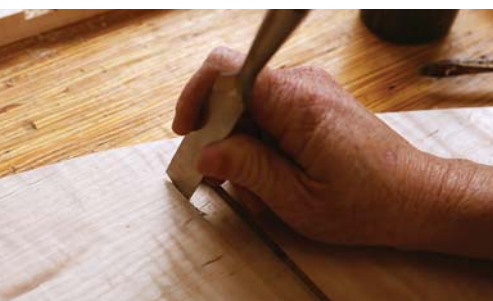
Square 1. Register the flat of the chisel off the flat of the end of the router cut, and rock it up to mark the remaining shoulders of the dado; try not to cross the penciled-in line of the dado's end.
