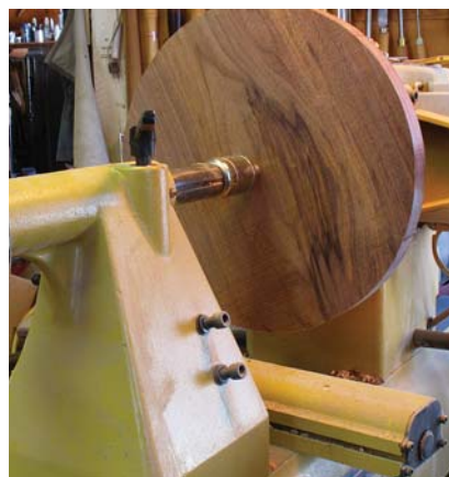
Double strength. While the face plate primarily holds the work, bring up the tailstock on the outboard side. Because you'll be leveraging pressure when truing the rim and face of the work, the extra holding power of the live center adds another measure of safety.
