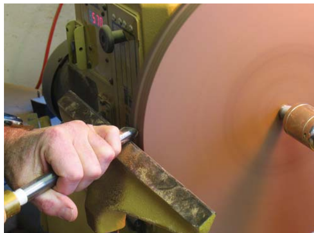
Round up. The first turning task is making the blank truly round. With the lathe set to about 500 rpm and the tool rest close to the work, make the cut with a bowl gouge across the thickness of the blank.
