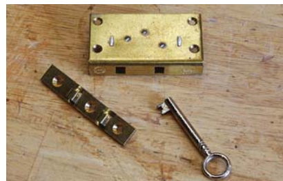
It takes three. Chest or box locks come with a third part, a strike. Protrusions on the strike become engaged with the lock's main lever to secure your valuables.
