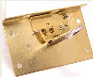
Mission completed. The main lever has slid to the unlocked position. The spring pushes the levers down to hold the lock open.
