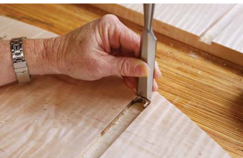
Square 2. With the chisel's flat facing away from the waste, define the end of the mortise then chisel out the remaining waste.
