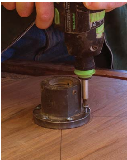
Dead center. The face plate is carefully positioned in the center of the top side of the turning blank and attached with #10 screws.
