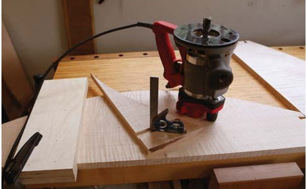
Trust but verify. After marking the dado locations and affixing my jig for the first cut, I ran a dado on a test piece first to confirm the depth of cut – which is 1/4".
