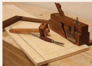
Raised-panel layout. With nothing more than a marking gauge and a rabbet plane, you can easily make raised panels.
