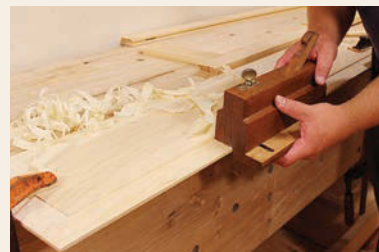
Adjust by eye. Make minor adjustments to the approach angle of the rabbet plane to sneak up on the bevel. Watch the corners; they will tell you where more wood must be removed. The adjacent bevels should meet in a straight line from the corner of the field to the outside corner of the bevel.
