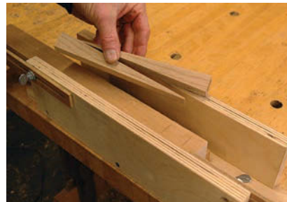
Line 'em up. After the end of the mortise layout is aligned with the bit, lock the workpiece in place using wedges.
