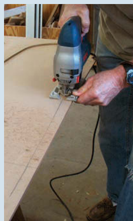
Cut out. Carefully cut the template with a jigsaw, staying tight to the line transferred from the paper.
