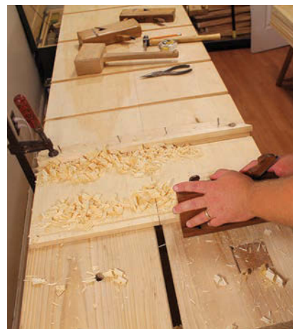
Two rabbets at once. Like planing the dados, planing the rabbets in both sides together ensures good alignment. It also prevents the rabbet on the near side board from splchling at the far edge.
