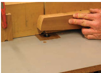
Cutting geometry. Move right to left when cutting at a router table.
