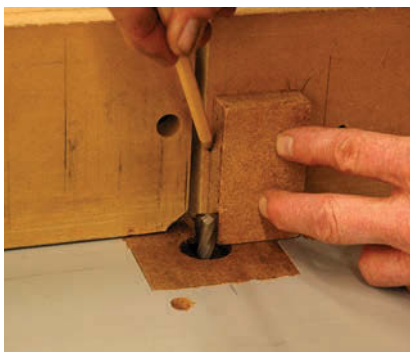
Bit of rotation. As you rotate the bit by hand, it pushes your scrap piece away. When the scrap stops, you've found the starting point of your cut. Align your mortise layout on these marks.
