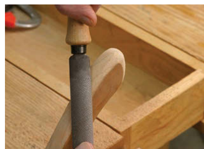
Off the top. A finer-grained rasp follows and quickly refines the surface by cutting off the peaks between the valleys.
