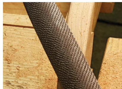
Regularly random. Hand-stitched teeth on rasps are in rows, but slight variations in the spacing allow more teeth to work to leave a smooth surface.
