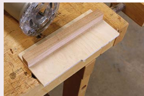
Dialed-in location. Running the router up the assembled jig cuts the jig exactly where the edge of the router bit does its work.
