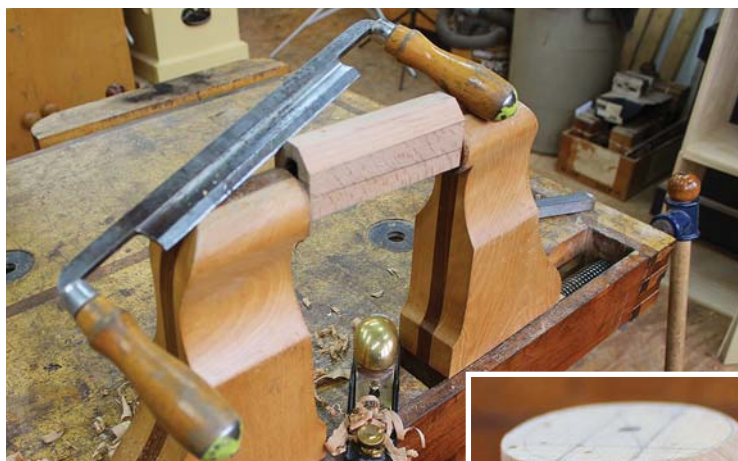
Shaping setup. My clamp for this sort of work resembles a lathe's headstock and tailstock. It holds the work securely as I shape the oval handle with a drawknife, block plane and spokeshave.
