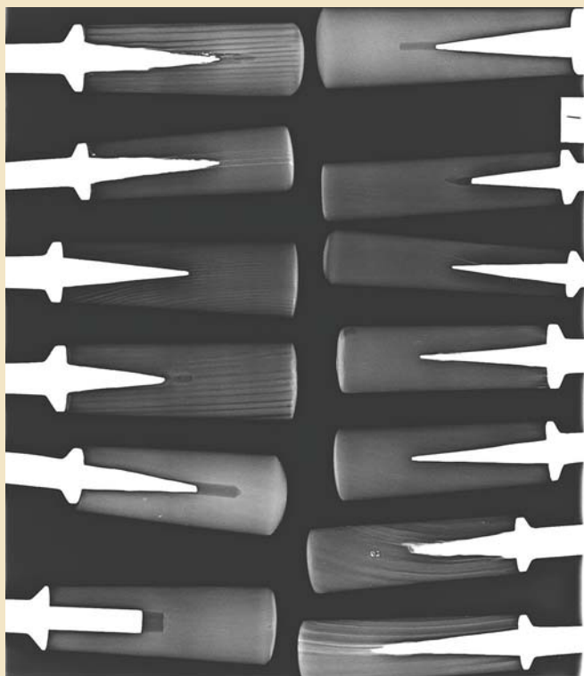
Inside & out. An X-ray reveals the tangs inside oval-bolstered mortise chisels.
